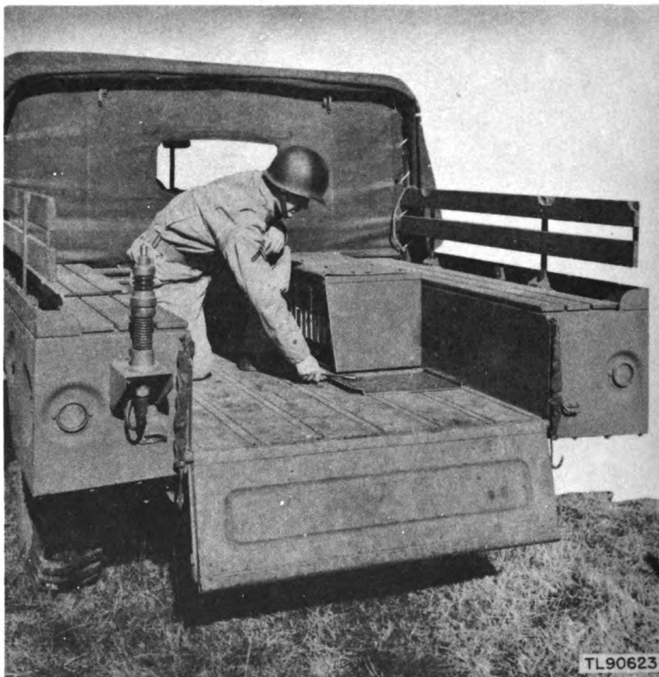
Figure 20. Bolting mounting plate to floor of vehicle.
