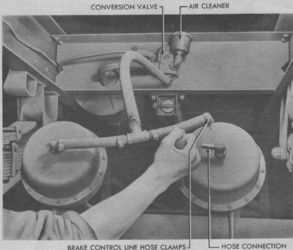
Figure 22—Removing Power Cylinder Diaphragm Cover Screws
