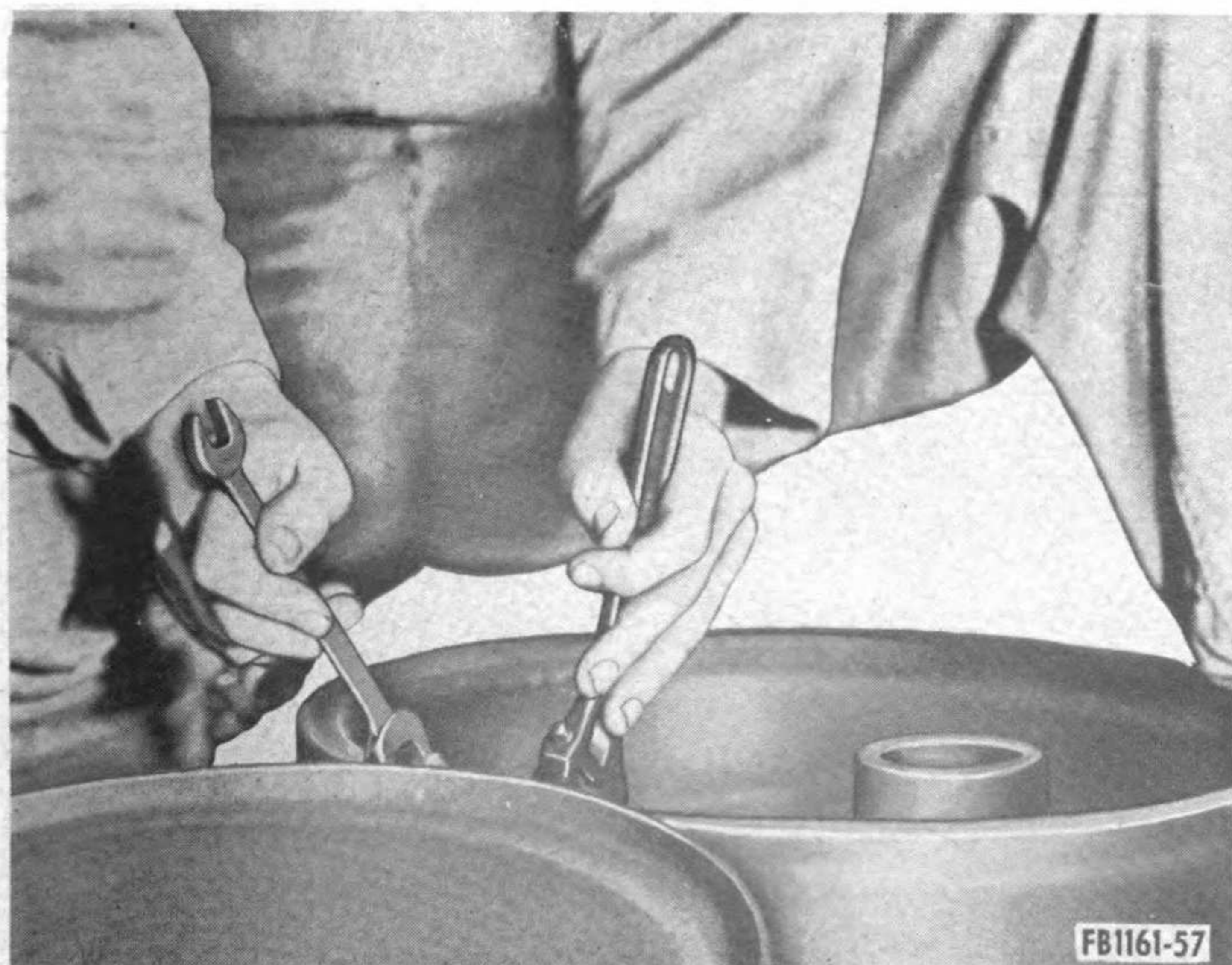
Figure 57. Removing manhole cover from tank.
