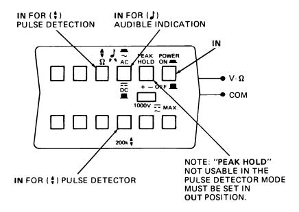
(2) Follow procedure for resistance measurement function (para 2-7g).
