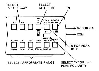
(2) To capture and display peak value, operate PEAK HOLD and slide switches as charted below for the appropriate input condition:
