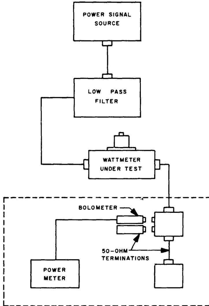
Figure 7-1. Coupler-Detector Test Set-up
