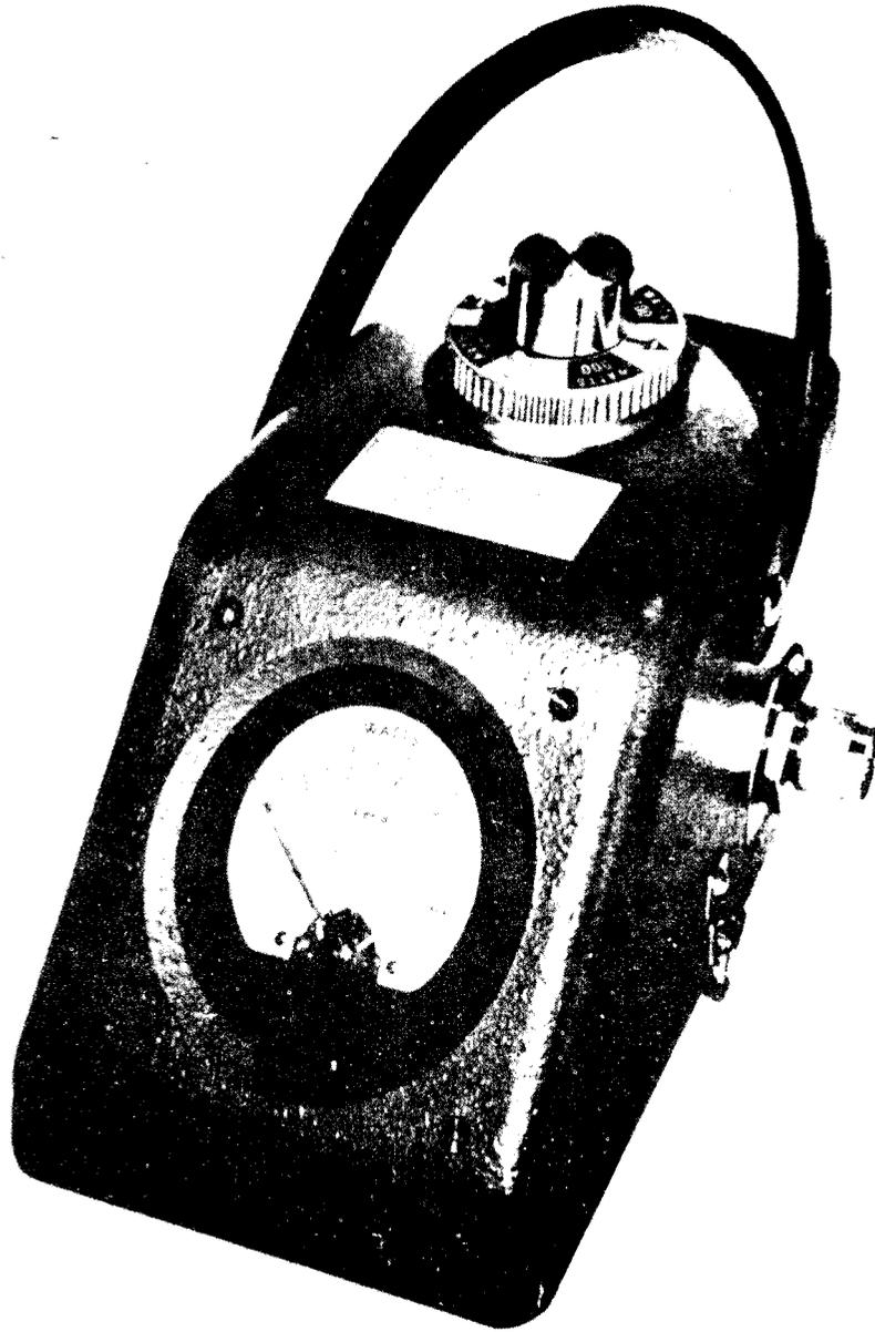
Figure 1-1. Wattmeter AN/URM-120
