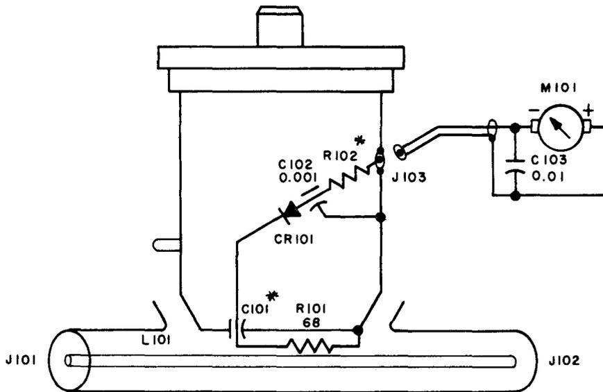
Figure 1-2. Wattmeter AN/URM-120, Schematic Diagram
