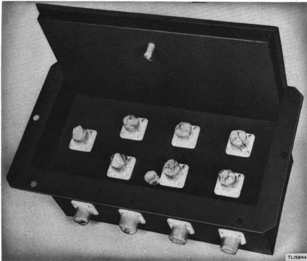
Figure 22. Control Box BC-1278-A, receptacles masked for moistureproofing and fungiproofing.
