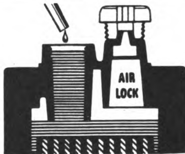
3. Fill well with distilled water. Air lock prevents solution rising above bottom of well.
