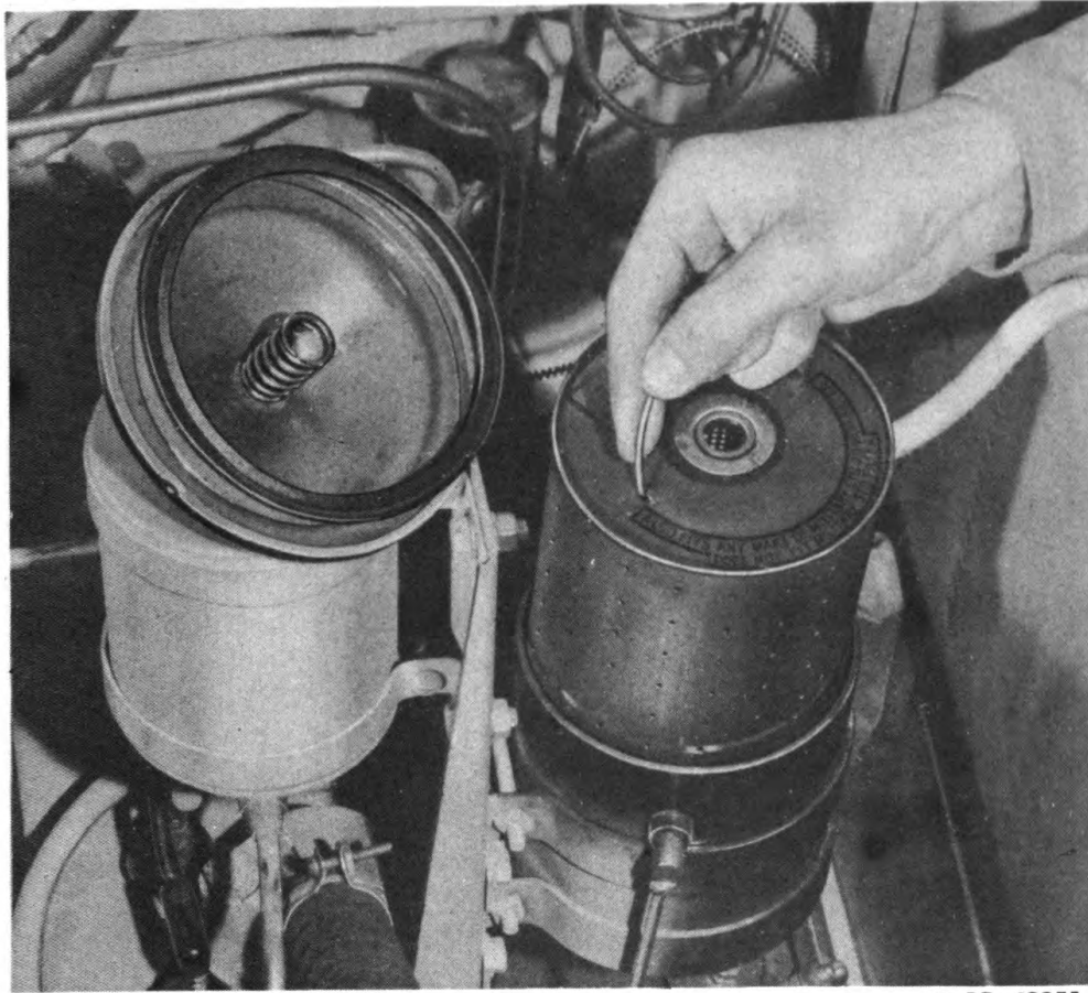
Figure 31—Oil Filter Cartridge Removal
