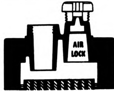
2. Place cap on safety-vent forming air lock in breather-chamber.
