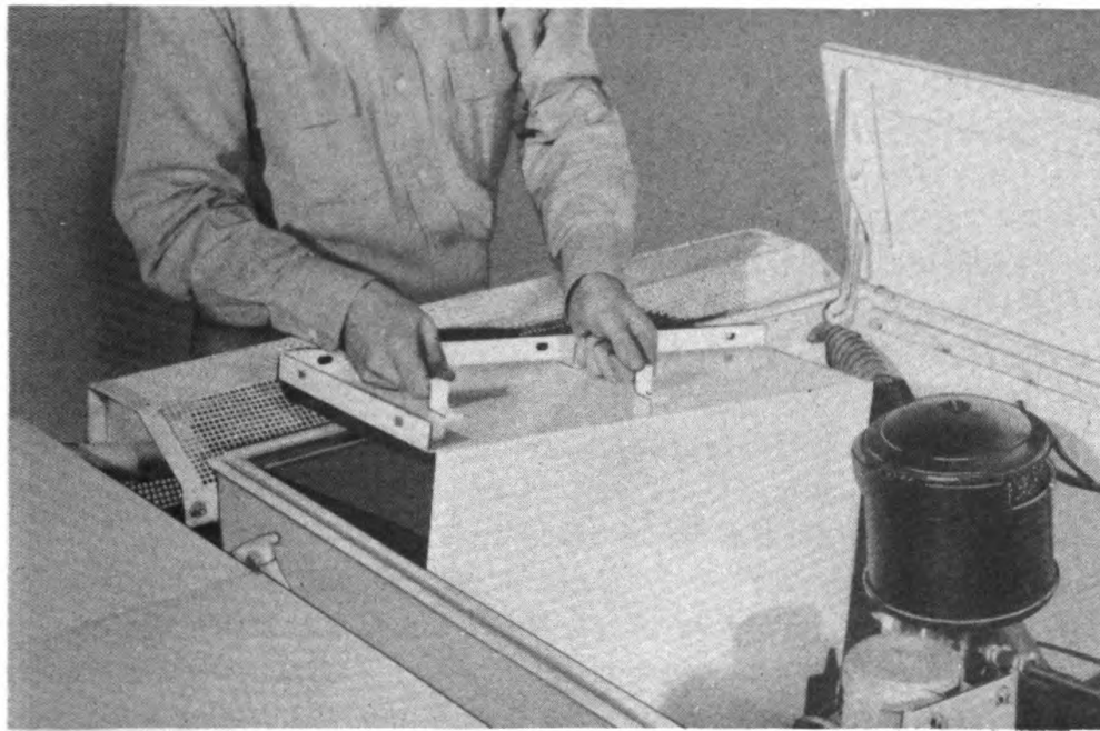
Figure 24 — Battery Compartment Cover Removal
