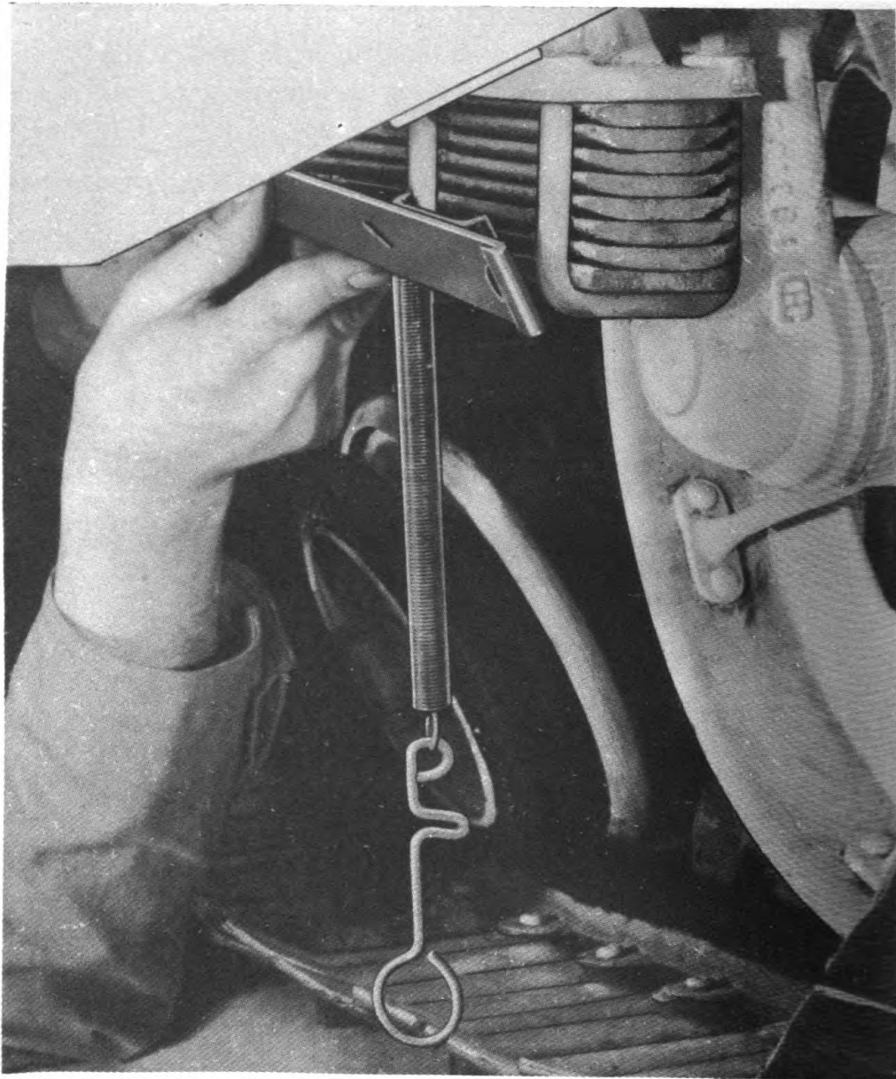
Figure 84—Positioning Track Tension—Gage SD902836
