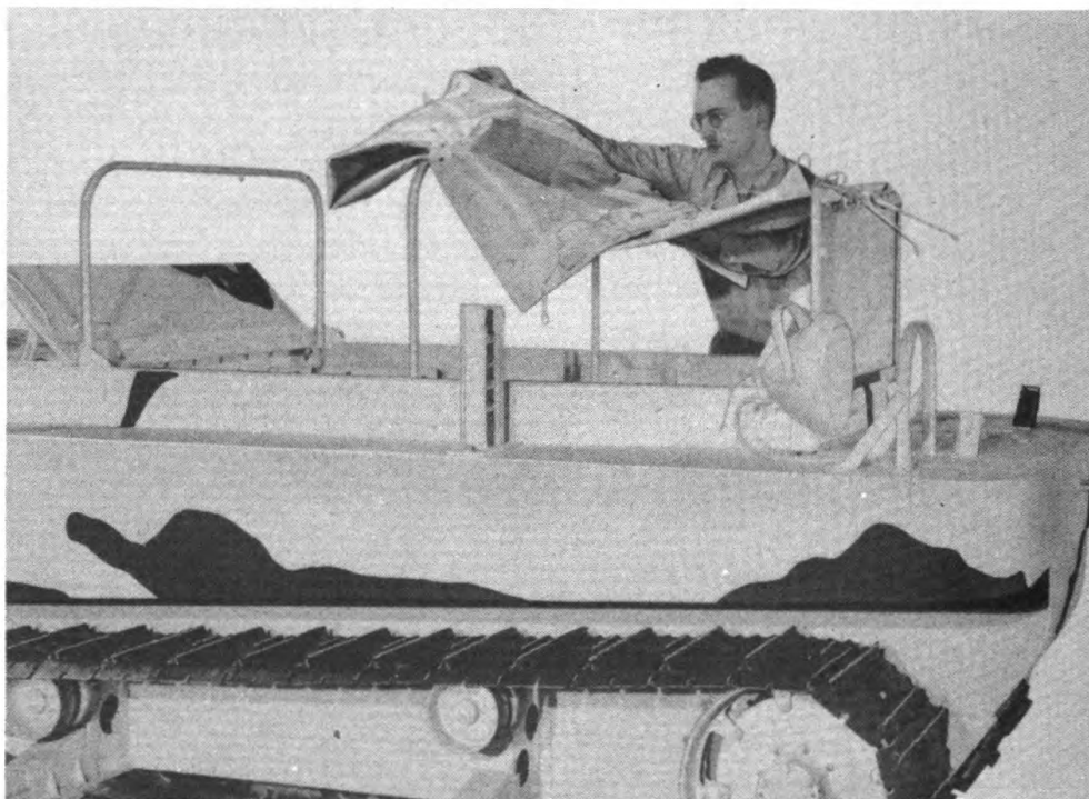
Figure 19—Removing Top from Vehicle
