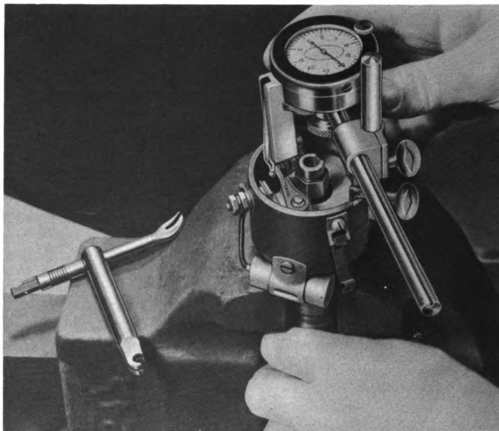
Figure 41—Checking Distributor Contact Point Gap with Dial Indicator UMS-40 and Alinement Tool AEE-38
