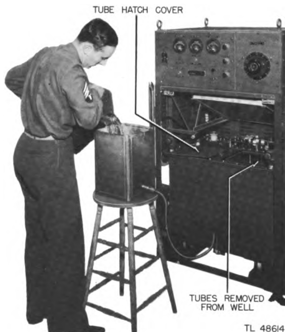
Figure 3-1. Refilling modulator oil tank.
