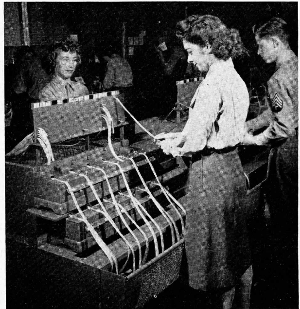
SEMI-AUTOMATIC RECEIVING CABINET—ONE OPERATOR HANDLES EIGHT CIRCUITS.
