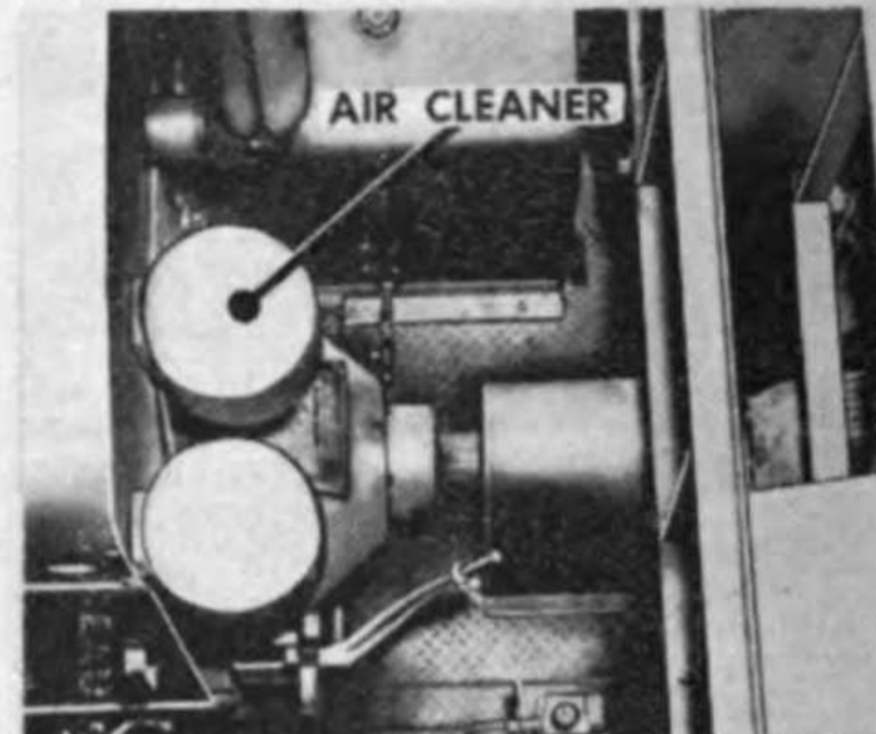
REFERENCE 10: Remove, clean, refill oil reservoir to level mark.
