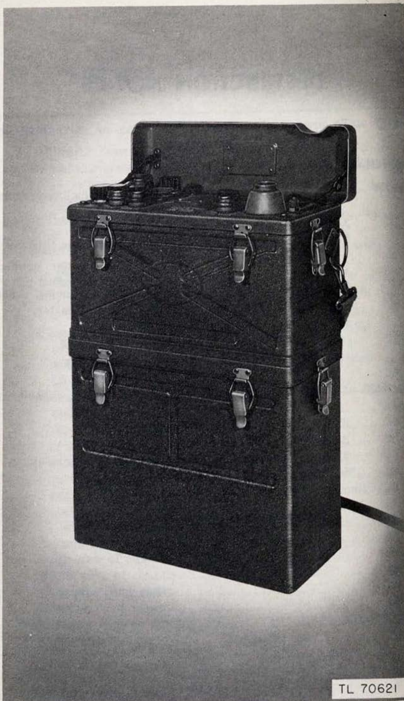
Vibrator Power Supply PP-114/VRC-3, shown mounted under Radio Receiver and Transmitter BC-1000-( ).
