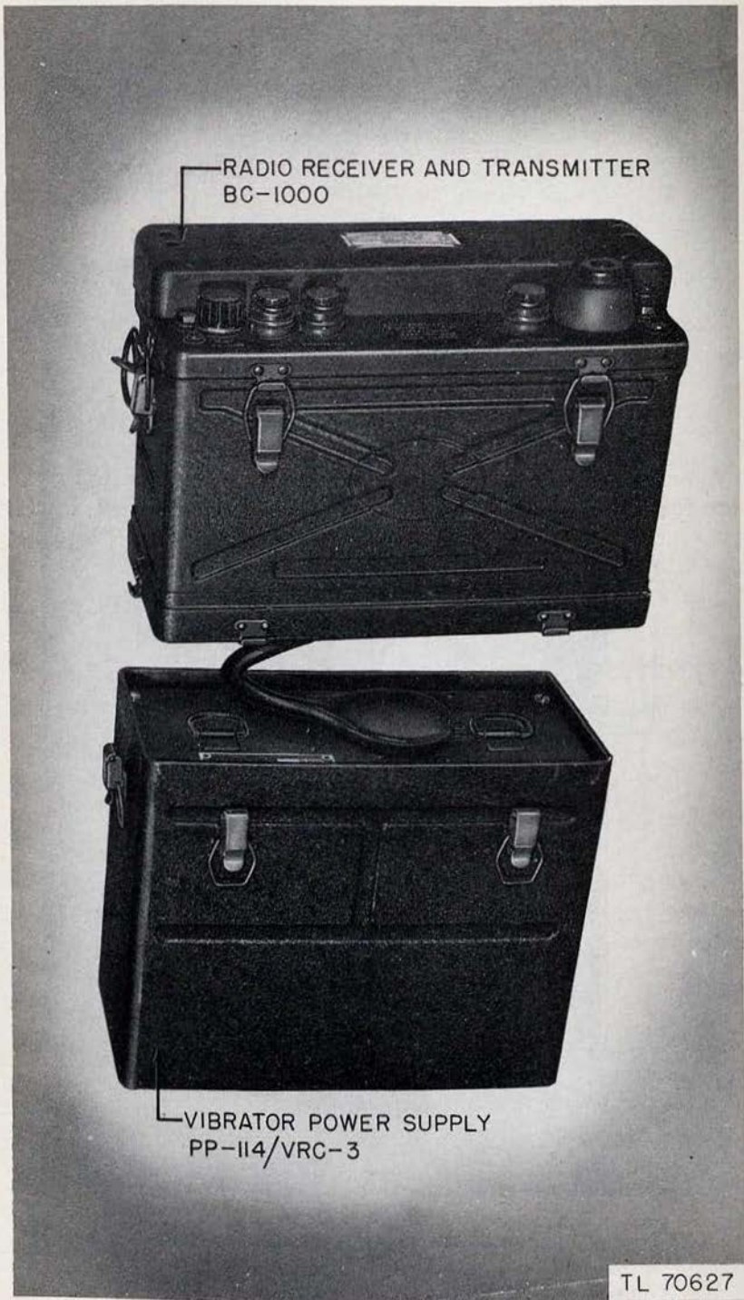
Figure 7. Connection of Vibrator Power Supply PP-114/VRC-3 to Radio Receiver and Transmitter BC-1000-( ).
