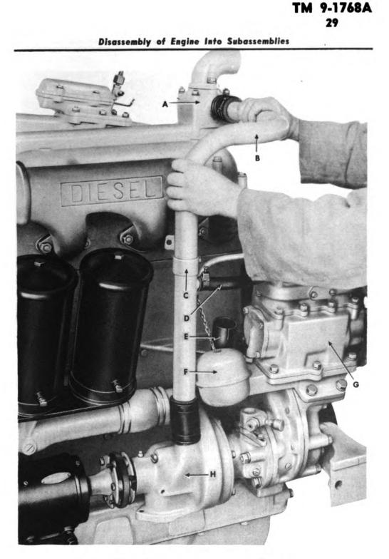
A - THERMOSTAT HOUSING B- THERMOSTAT BY-PASS TUBE C--CLAMP D--AIR COMPRESSOR BY-PASS HOSE
