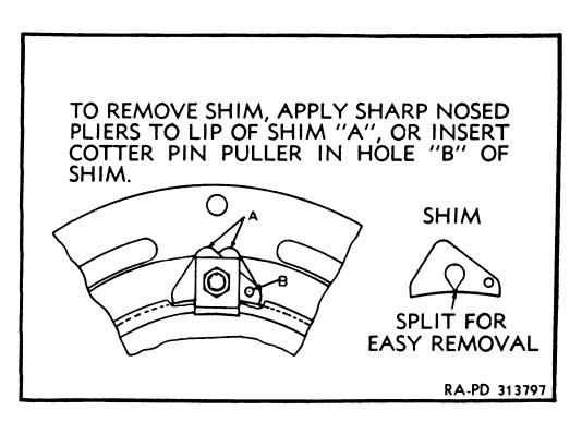
Figure 104—Clutch Shim Removal
