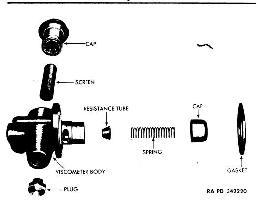
Figure 83—Viscometer Instrument, Disassembled
