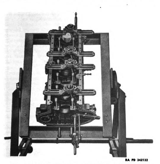
Figure 29—Line-boring machine (41-B-20) Installed for Linereaming Camshaft Bearings (Rear End)
