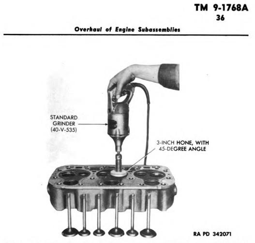
Figure 61—Grinding Intake Valve Seat, Using Grinder (40-V-535) and 3-inch Hone (45-degree Angle)
