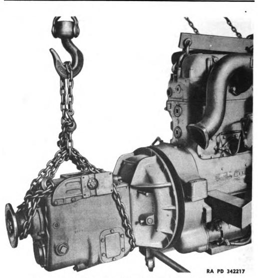
Figure 10-Removing Transmission From Engine
