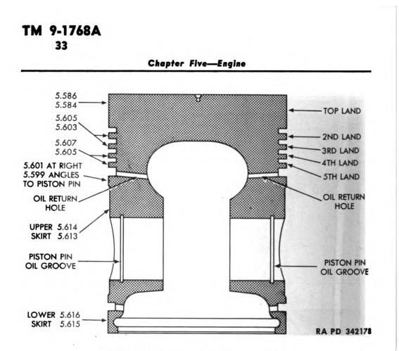
Figure 39—Sectional View of Piston
