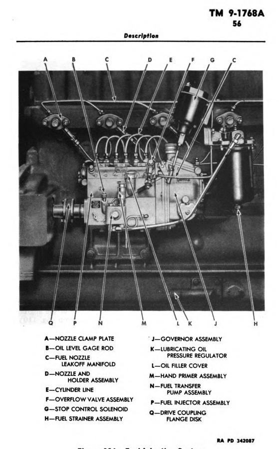
Figure 106—Fuel Injection System
