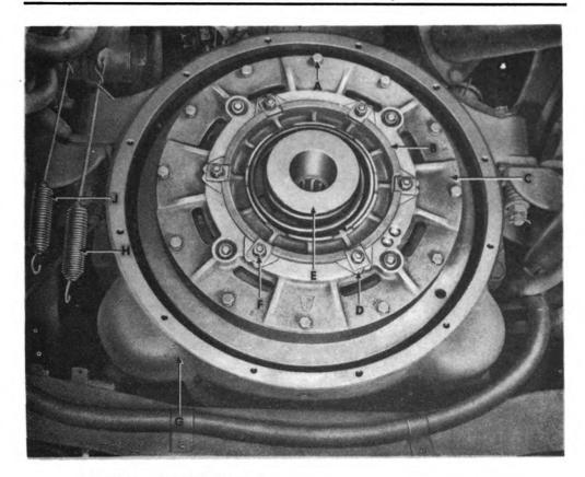
A --- CLUTCH MOUNTING BOLT B--- ADJUSTING PLATE C--- PRESSURE PLATE ASSEMBLY D--- ADJUSTING SHIMS E--- CLUTCH RELEASE SLEEVE
