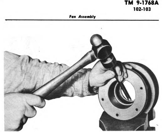
RA PD 342214 Figure 178—Removing Bearing Cup From Fan Pulley Hub
