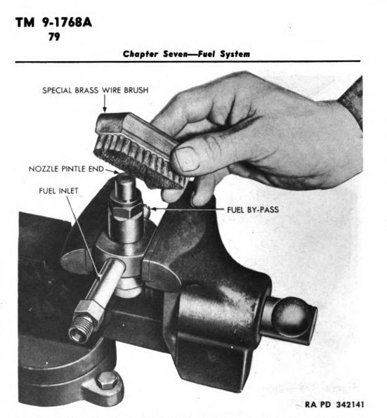
Figure 156—Cleaning Pintle End of Nozzle, Using Special Brass Wire Brush (38-B-982)
