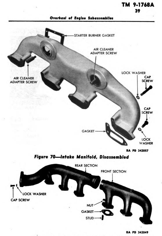
Figure 71—Exhaust Manifold, Disassembled
