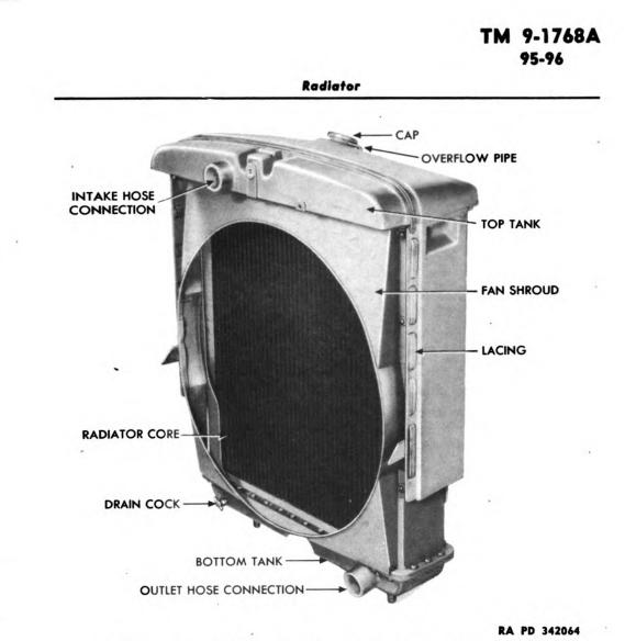
Figure 174—Three-quarter Rear View of Radiator
