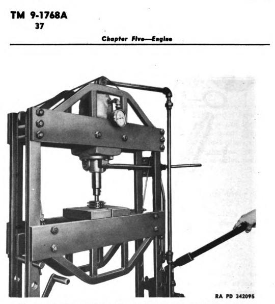
Figure 66—Pressing Fuel Pump Driven Sprocket From Shaft
