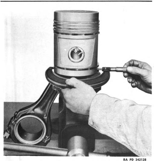
Figure 38—Measuring Diameter of Piston Skirt
