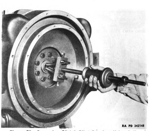
Figure 53—Removing Clutch Pilot Bearing, Using Püller (41-P-2957)
