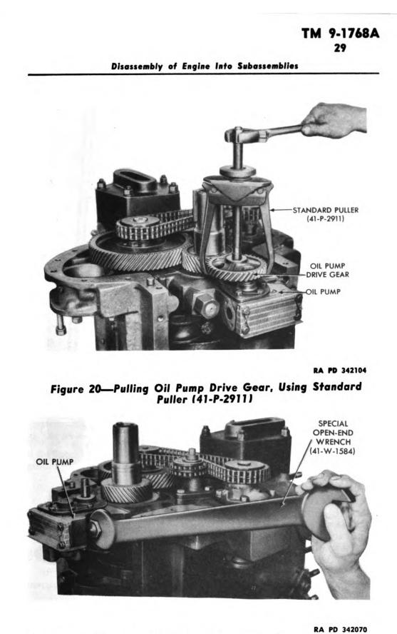
Figure 21—Removing Nuts From Front Main Bearing Cap, Using Special Wrench (41-W-1584)
