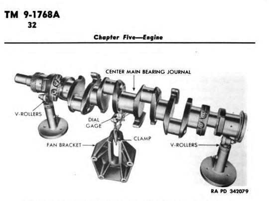
Figure 34—Method of Checking Crankshaft for Run-out
