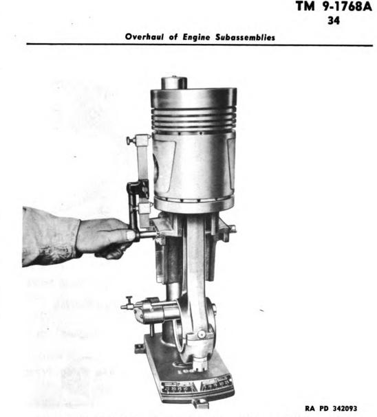
Figure 49—Checking Connecting Rod Alinement, Using Aliner (41-A-135)
