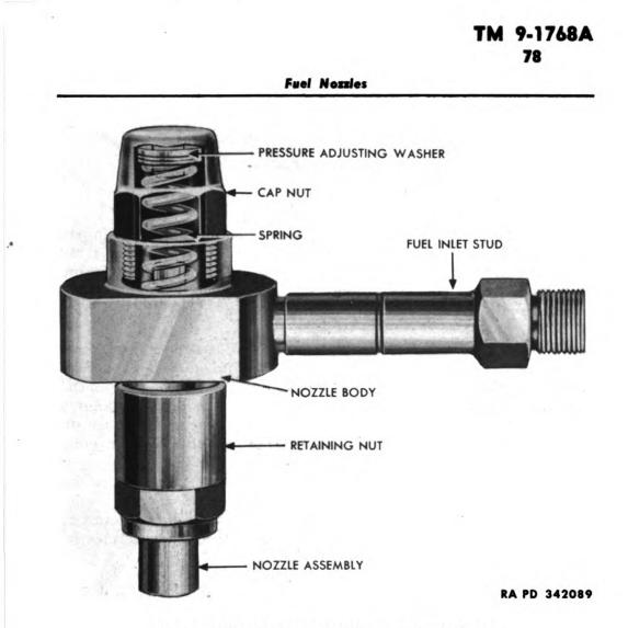
Figure 153—Cutaway View of Fuel Nozzle
