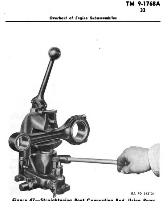
Figure 47—Straightening Bent Connecting Rod, Using Press (41-P-2730)
