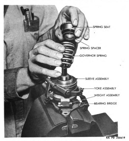
Figure 141—Removing Governor Spring Assembly
