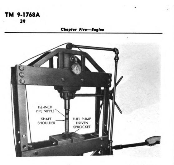
RA PD 342075 Figure 69—Pressing Fuel Pump Driven Sprocket on Shaft
