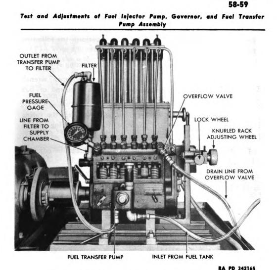
Figure 120—Set-up for Checking Overflow Valve
