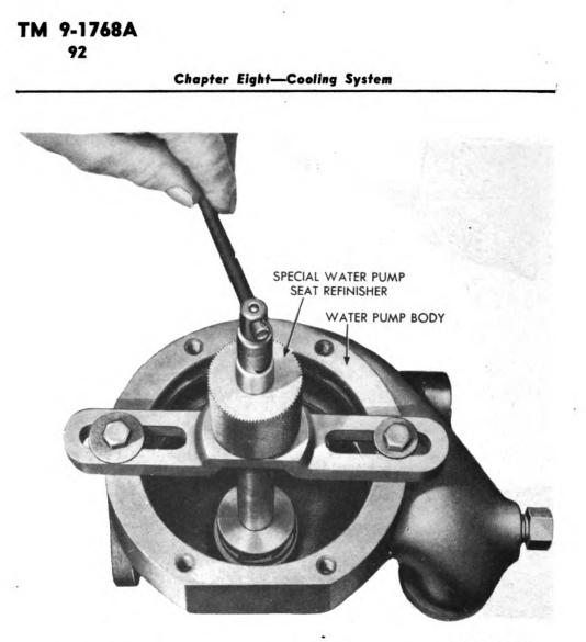
Figure 168—Refacing Seal Washer Seat in Water Pump Body, Using Special Seat Refacer (41-T-3095-500)
