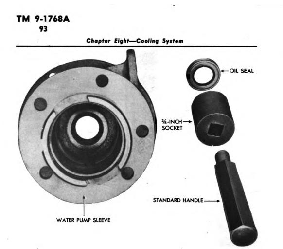
Figure 170—Tools Used To Install New Oil Seal in Water Pump Sleeve
