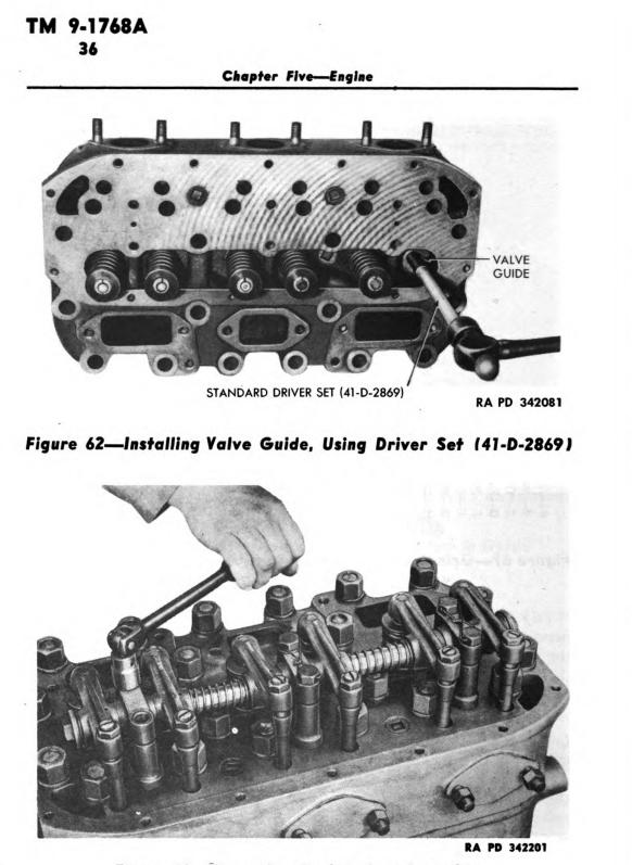
Figure 63—Removing Rocker Arm Assembly
