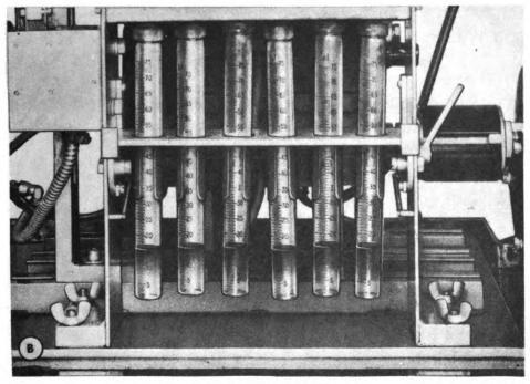
CALIBRATION TUBES—FINAL RUN RA PD 342218 Figure 118—Set-up Showing Steps in Calibration of Fuel Injector Pump
