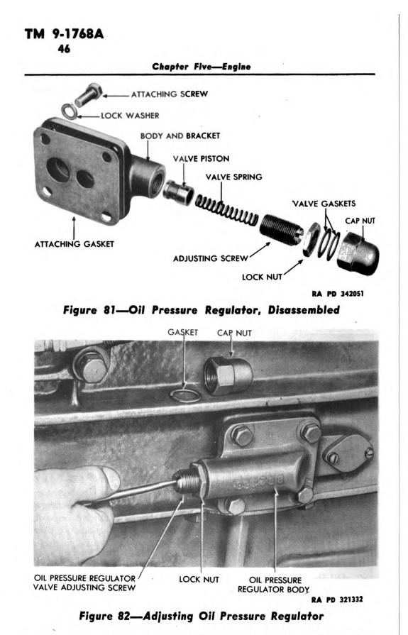
is 12 pounds at  $1\frac{7}{8}$ -inch height. Free length of spring is  $2\frac{1}{4}$  inches. Valve should open at 40 pounds. Clearance of valve in body is 0.002 to 0.006 inch. Wear limit is 0.004 inch.
