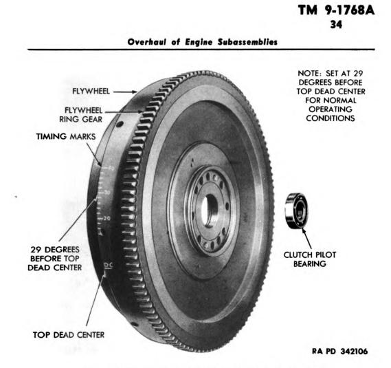
Figure 52—Flywheel and Clutch Pilot Bearing
