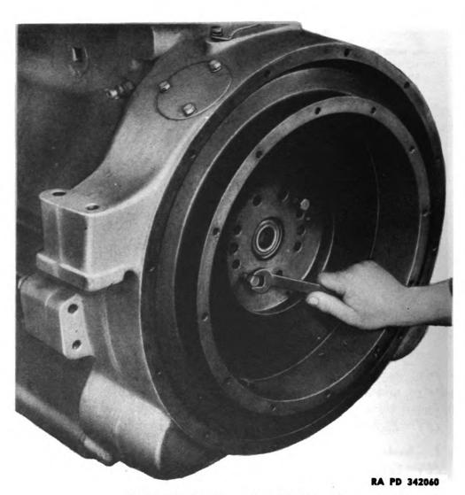
Figure 12—Removing Flywheel
