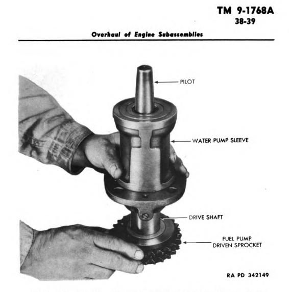
Figure 68—Inserting Fuel Pump Drive Shaft in Sleeve, Using Special Pilot (41-P-405)
