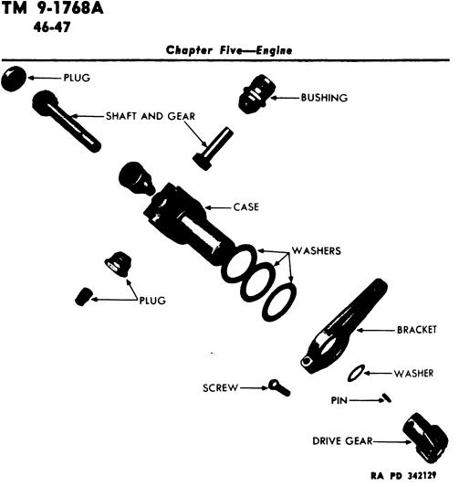
Figure 84—Tachometer Drive, Disassembled
