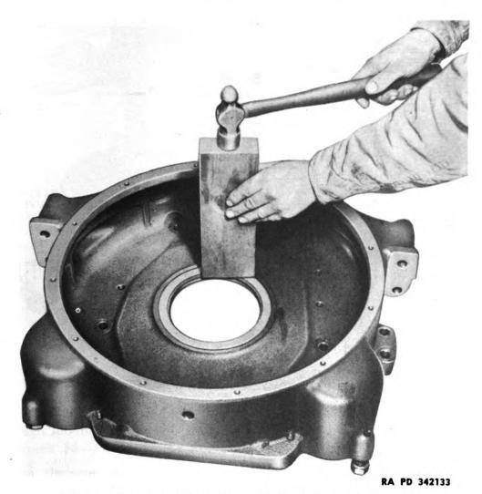
Figure 54—Installing New Oil Seal in Bell Housing
