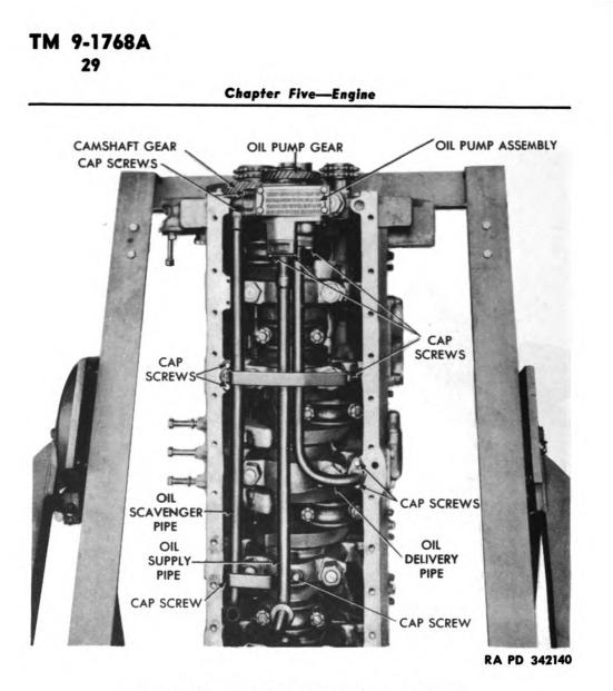
Figure 19—Oil Pipe Assembly Installed
