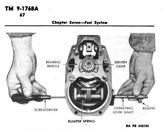
Figure 147—Inserting Operating Lever Shaft
