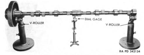
Figure 31—Checking Camshaft Alinement
