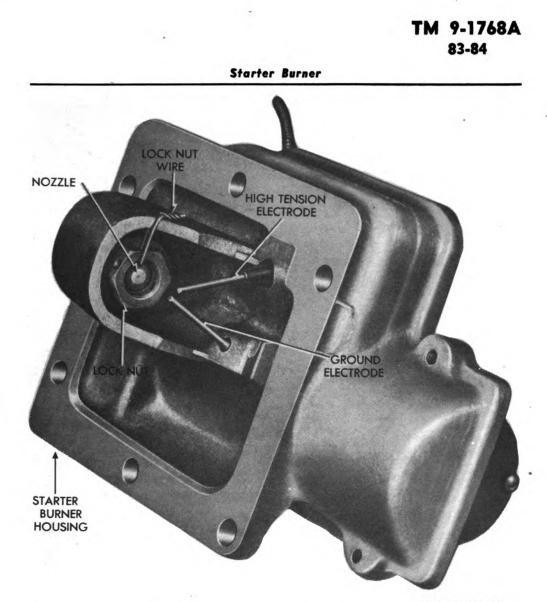
Figure 160—Starter Burner, Showing Nozzle and Electrodes
