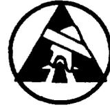
Static electricity can damage the control-monitor modules. Ground the control-monitor before removing a module. Use a grounded wrist strap when handling the a module.
