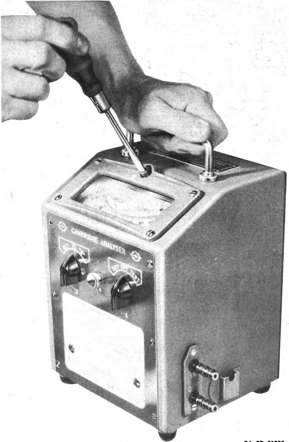
Figure 12—Making Mechanical Zero Adjustment (Calibration No. 1)
