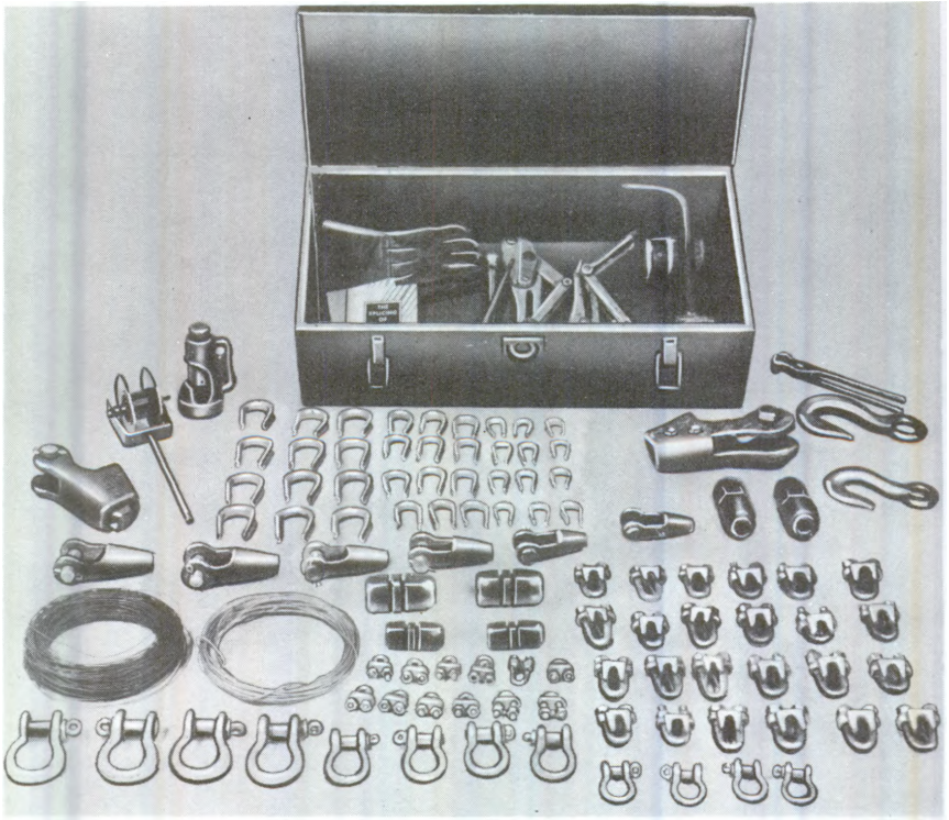
Figure 27. Rigging equipment set No. 1.
