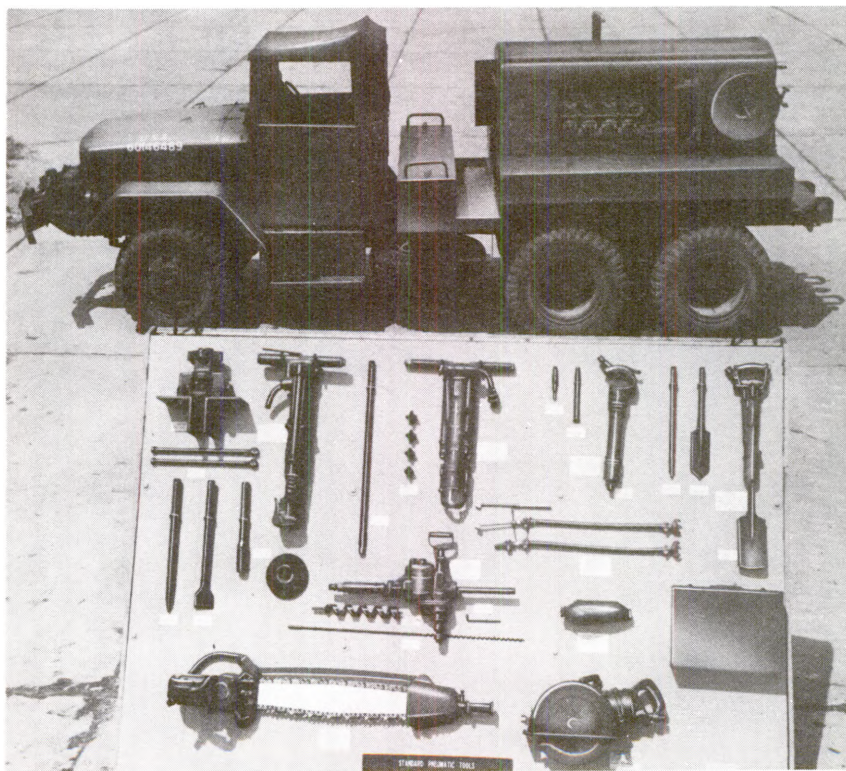
Figure 36. Truck-mounted air compressor, 210-cfm (2½-ton 6 x 6 truck).
