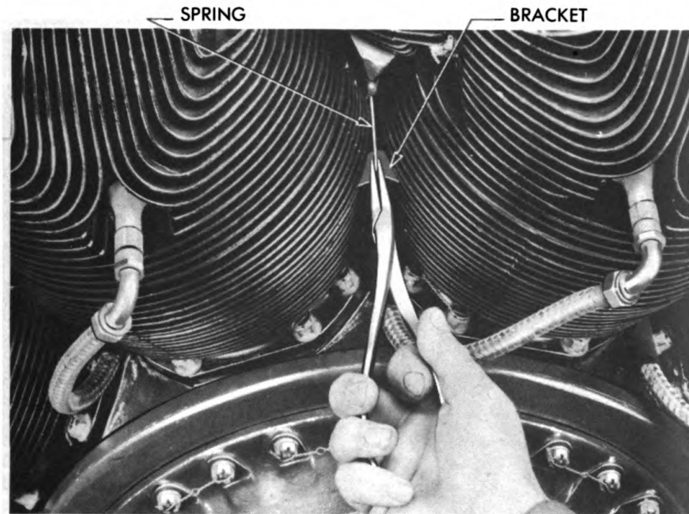
Figure 41 – Unhooking Intercylinder Baffle Attaching Spring
