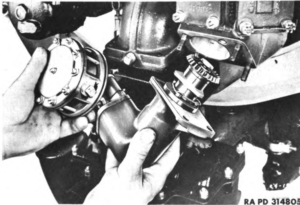
Figure 247 – Installing Fuel Pump
