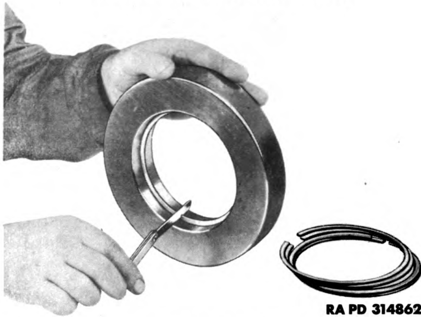
Figure 113 – Measuring Piston Ring Gap Using Gage 41-G-400 and Ring 41-R-2492
