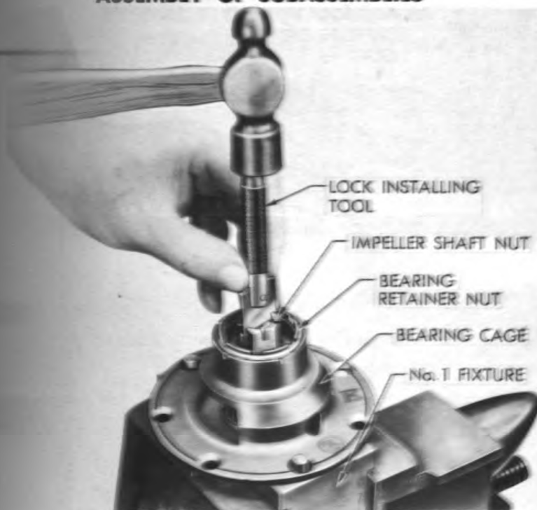
Figure 161 - Installing Lock in Impeller Drive Shaft
