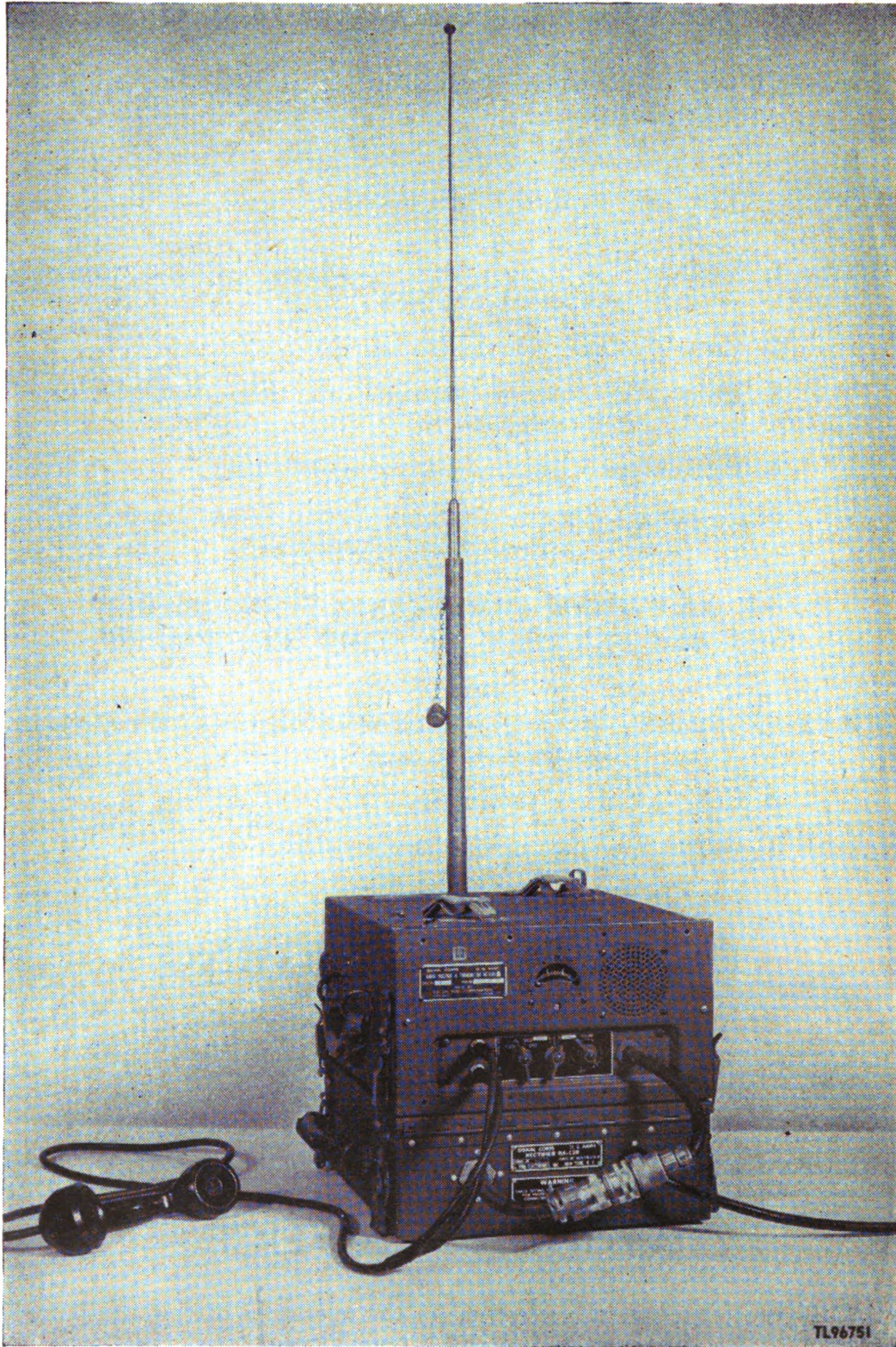
Figure 1. Rectifier RA-120, set up for operation.
