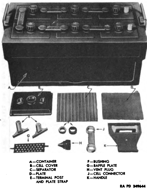
Figure 131. Battery Components.
