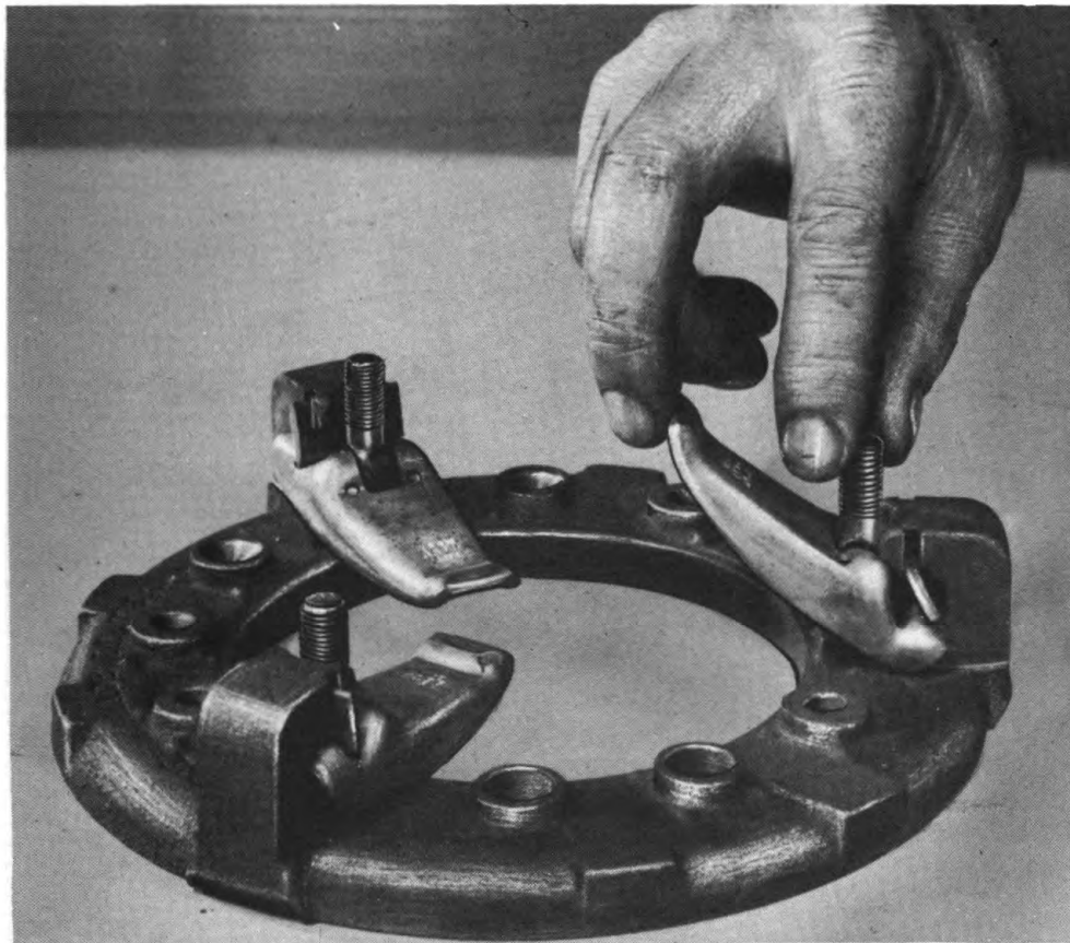
Figure 84—Removing or Installing Release Lever in Eyebolt
