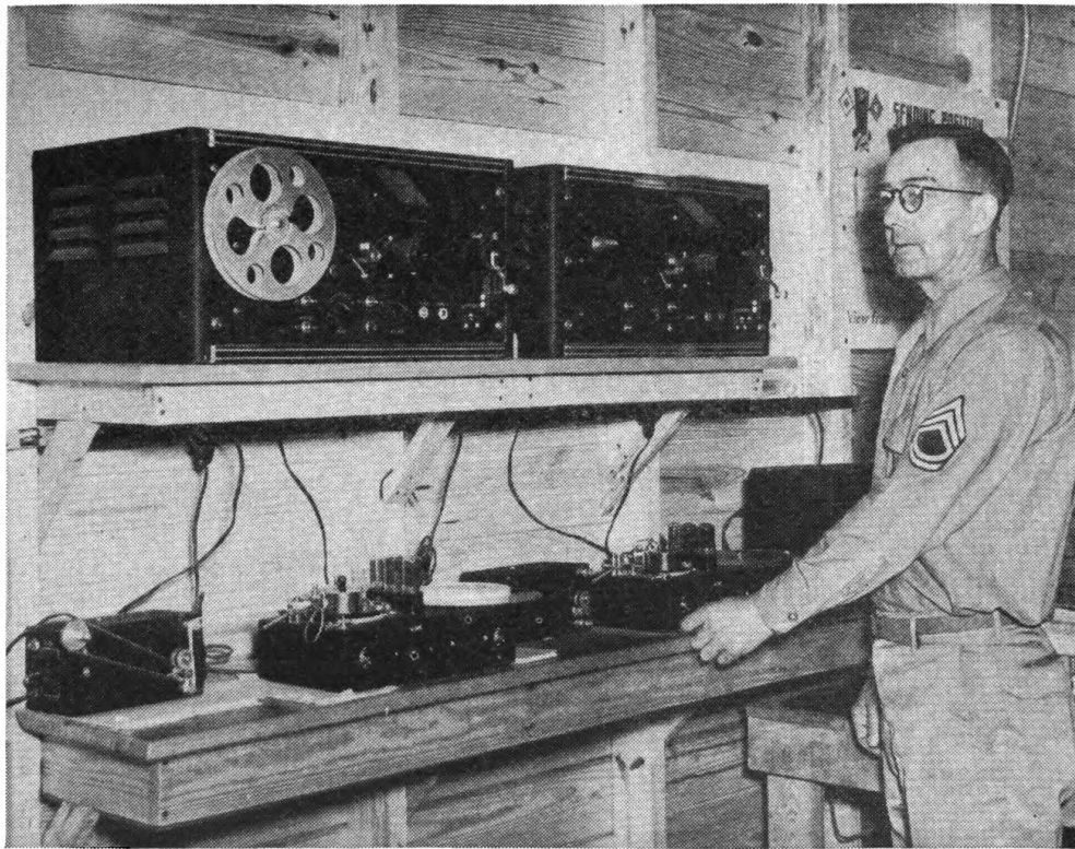
FIGURE 3.—Recorder position. (On lower shelf are two McElroy recorders with associated tape pullers; on upper shelf are two Lon-Ga-Tone units. Tapes made on recorders can be played back immediately on Lon-Ga-Tone keyers.)
