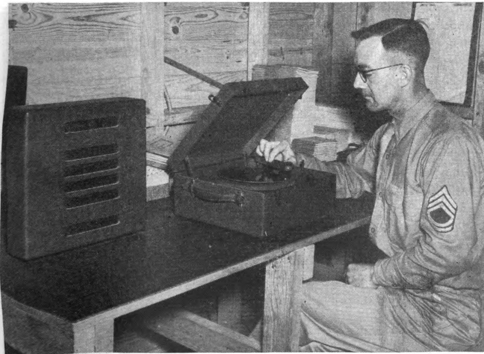
FIGURE 4.—Record player set-up for transmission of radiotelegraph operator aptitude test: (Speaker (left) is detached from cover of carrying case.)
