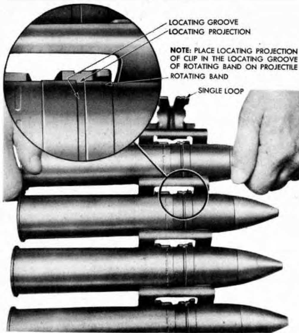
Figure 12—Belting 37-mm Ammunition
