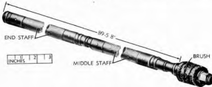
Figure 5—37-mm Bore Brush M8 (B157305) and 37-mm Cleaning Staff M5A2 (B154621)
