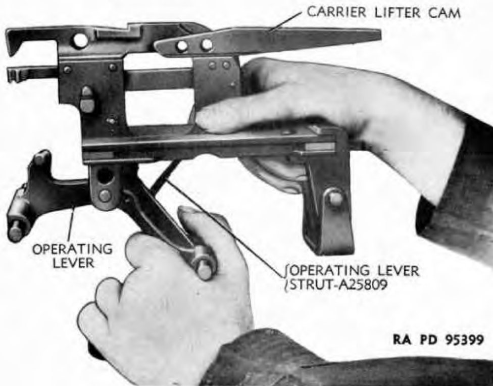
Figure 46—Easing the Operating Lever Forward
