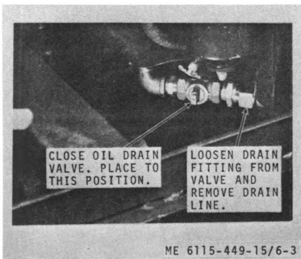
Figure 6-3. Engine oil drain line, removal and installation.
