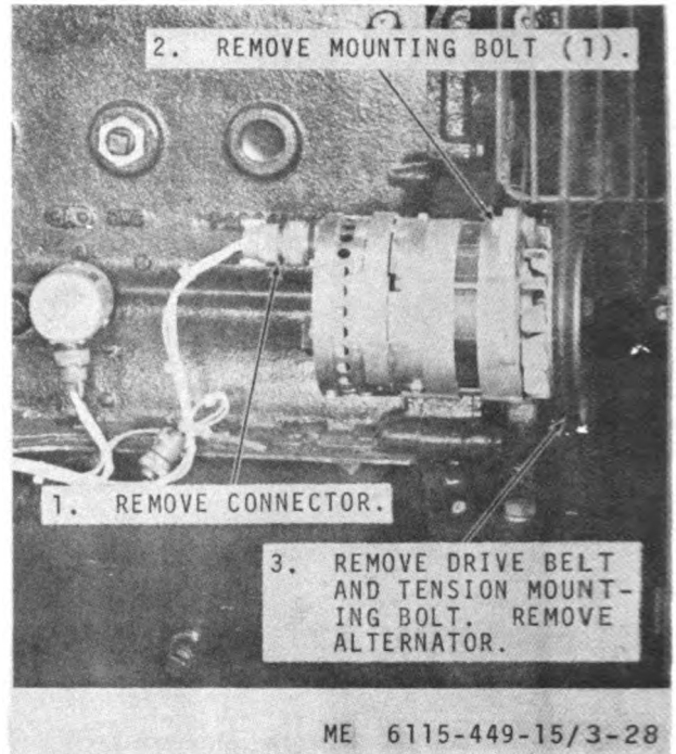
Figure 3-28. Alternator, removal and installation.
