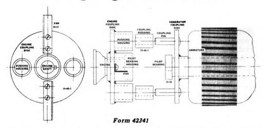
The above drawings show the coupling arrangement of these plants in detail. In time, the rubber bushings (44) of this coupling will wear and lose their resiliency and must be replaced.
