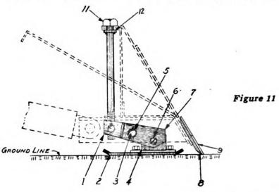
inserting the proper amount of shims, at (1) Figure 9, between the angle clips at the hinge point of the scraper, and then bolting up rigid. Desired crown is then correctly and automatically maintained.
