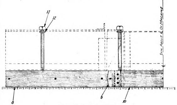
Assembly of Scraper Blade
