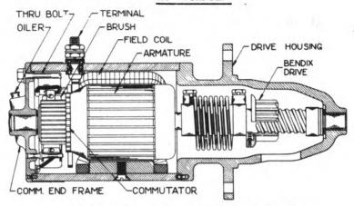
Figure V - Delco-Remy Starting Motor
