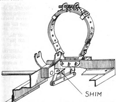
Figure 45A. Showing adjustment of clutch and brake lever linkage by inserting shims. For general view of steering lever assembly, see Parts Section.
