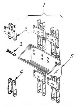
Figure 112. Bucket and bucket line chain.
