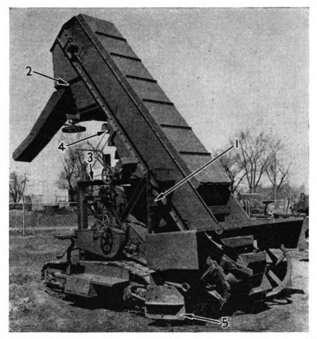
Figure 114. Loader in normal operating position. For ordinary loading operations,
