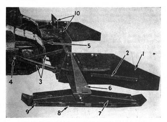
Figure 132. Floating cleanup scraper with guide wings attached.
