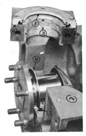
Figure F Rear Bearing Cap and Seal
