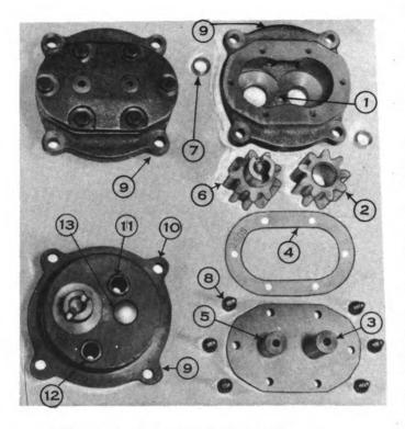
Figure M - Exploded View of Oil Pump
