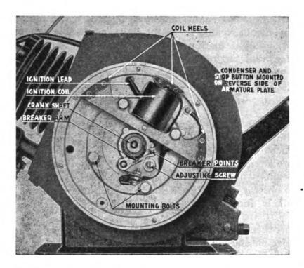
Its operation is extremely simple:—As the pole pieces of the magnet pass over the heels of the coil, a magnetic field is built up about the coil, causing a current to flow thru the primary winding.
