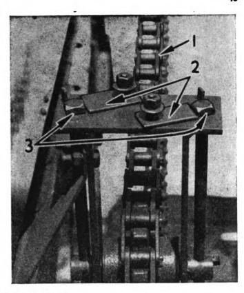
Figure 41. Take-up for Bucket Line drive chain showing lock plates and take-up bolts,
