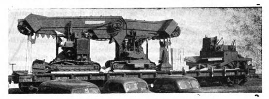
Figure 46. Method of transporting two loaders and a B-G Finisher on a standard 53' flatcar.
