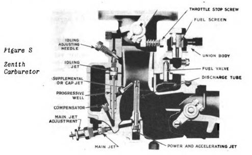
The Main Jet flow varies with suction, delivering more fuel as the engine speed increases, thus its tendency is to richness at top engine speed. The Compensating Jet is not affected by suction, thus flows the same at all speeds and has a tendency to leanness at top engine speed. In combination, the rich and lean jets give an average mixture of correct proportions.
