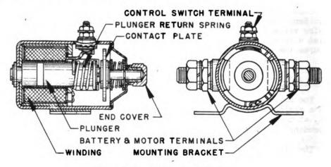
Figure AA - Magnetic Switch
