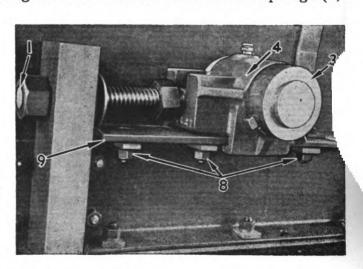
Figure 102. Bucket line chain take-up, operating on the boom head shaft, has Acme screw thread.
