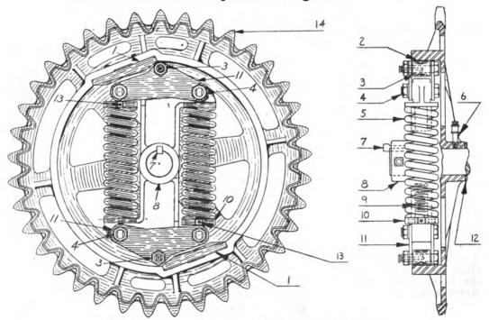
Figure 104. Details of spring release sprocket.
