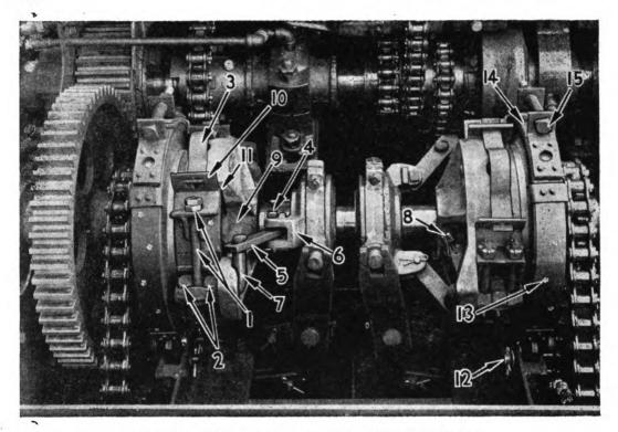
Figure 120. Replacing clutch bands and linings.
