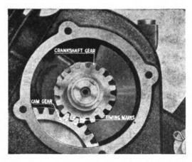
VALVES — The valves are properly timed on every IRON HORSE before it leaves the factory, therefore it should cause no concern. However, if the engine has been completely disassembled and the valves thrown out of time, proceed as follows: Note punch marks on cam and crankshaft gears.
