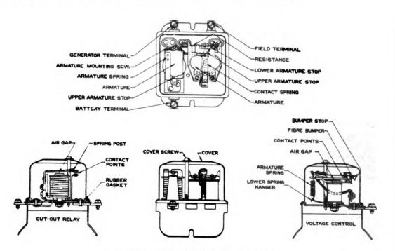
Figure Z - Step-Voltage Control Unit
