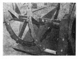
Figure 110. Replaceable, notched wearing strips on the feeding spirals. The entire spiral assembly is bolted to the foot shaft.
