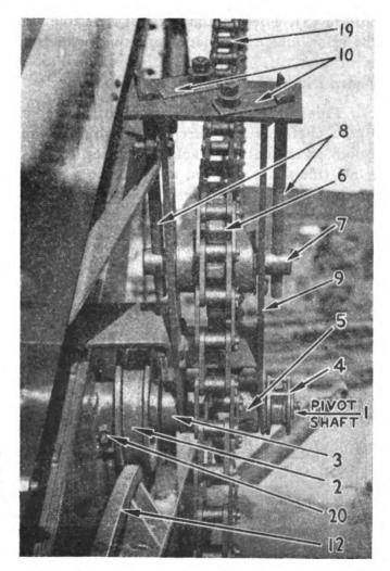
Figure 106. Bracket on side of boom showing pivot shaft, and bucket line drive chain sprocket.
