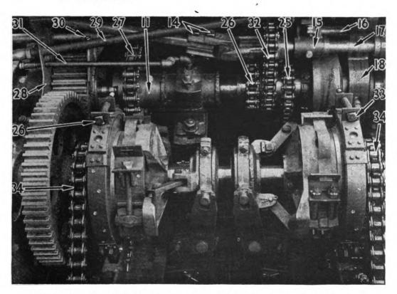
Figure 118. Interior of tractor unit housing showing main jack shaft above and crawler clutch shaft below.
