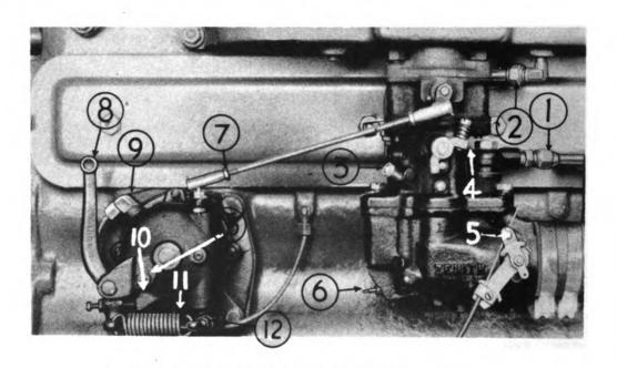
Figure R - Close-up of Governor and Carburetor.
