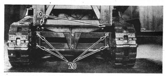
Figure 131. Crawlers remain parallel over uneven ground through use of the Barber-Greene oscillating type of axle.
