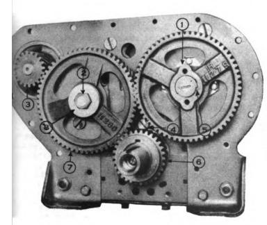
Figure I - Timing Gear
