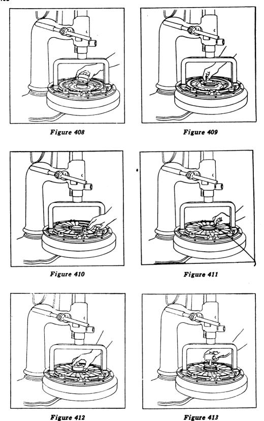
Assemble the remaining fulcrum ring (113) firmly and carefully over the sleeve (116). Be sure no ball bearings become displaced, or that the levers overlap each other. Figure 412.
