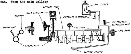
line, side passages are drilled to the main bearings and idler gear stud. From the main bearing the oil is delivered to the crank bearings by means of the drilled crankshaft. The piston pin receives its oil from the crank pin bearings through the rifle drilled connecting rods. The cylinders are lubricated by oil thrown from the crank pin bearings.
