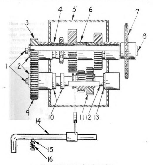
Figure 125. Cross section of gear box.
