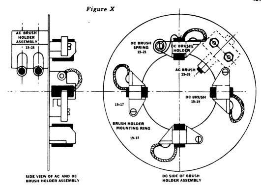
Above is shown the brush holder arrangement in detail. Brushes must be replaced before they are worn to the extent that they will not make proper contact on the commutator or slip rings. Clean commutator and slip rings occasionally with #00 sand paper.
