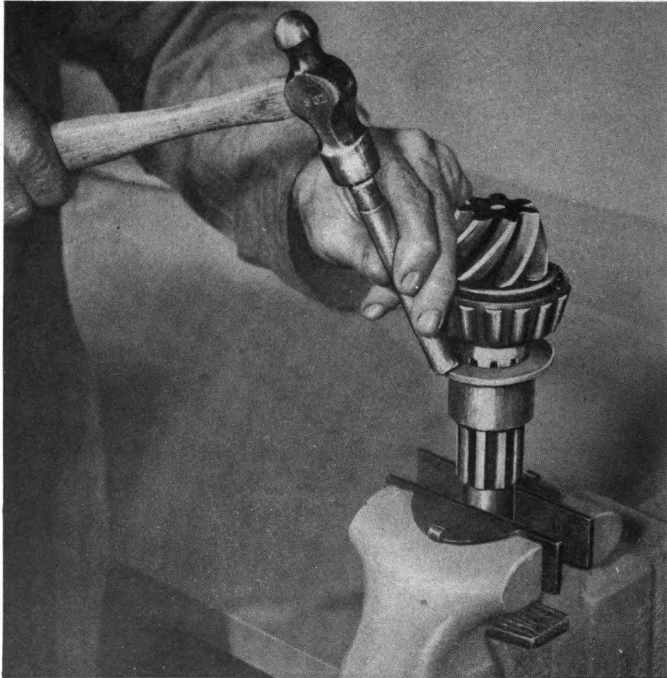
Figure 70—Removing Pinion Low Speed Gear Bearing Sleeve and Thrust Washer
