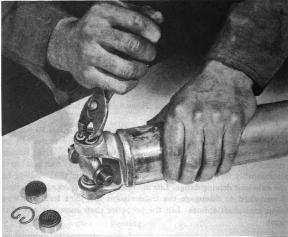
Figure 31—Universal Joint Bearing Lock Ring Removal
