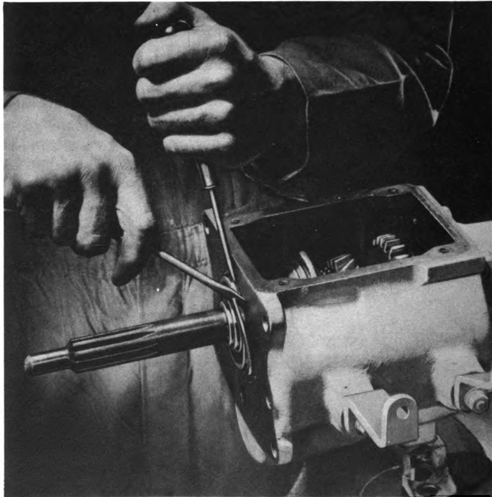
Figure 7—Pinion Bearing Retainer Ring Removal
