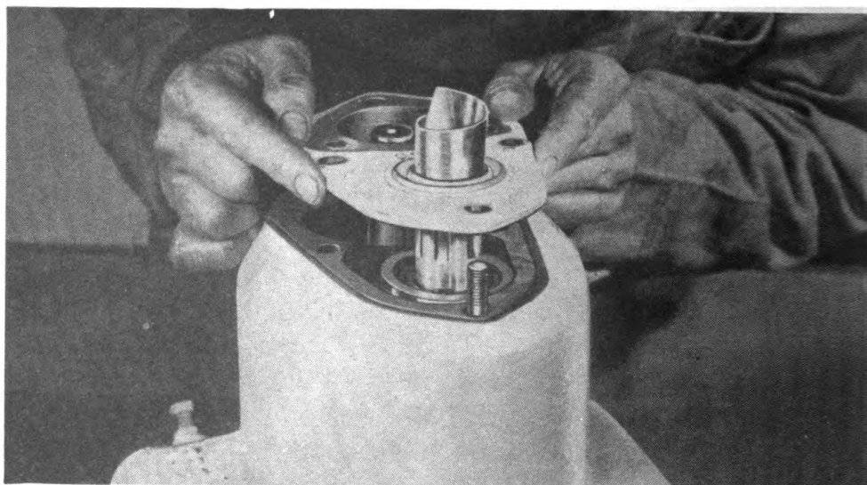
Figure 87—Method of Installing Axle Transmission Front Cover Plate
