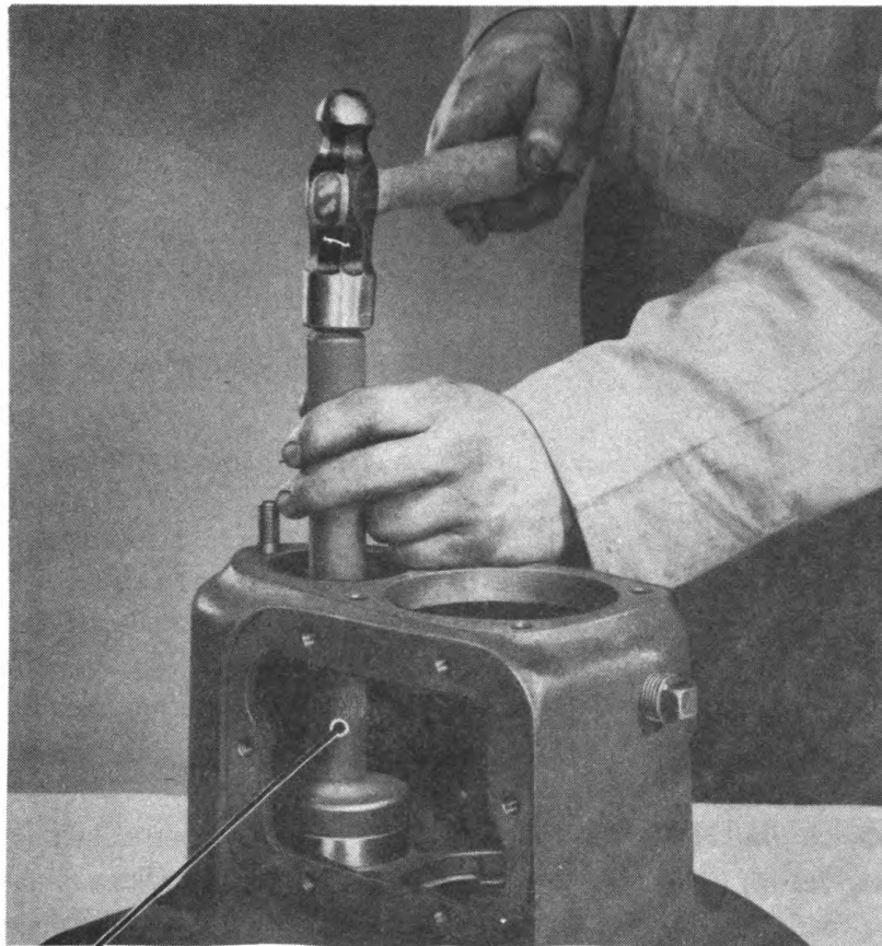
Figure 80—Installing Mainshaft Front Oil Seal
