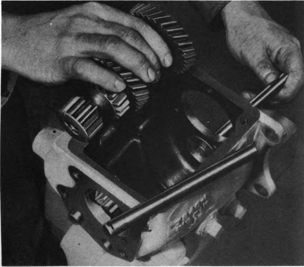
Figure 25—Method of Installing Countershaft Gear Cluster and Shaft
