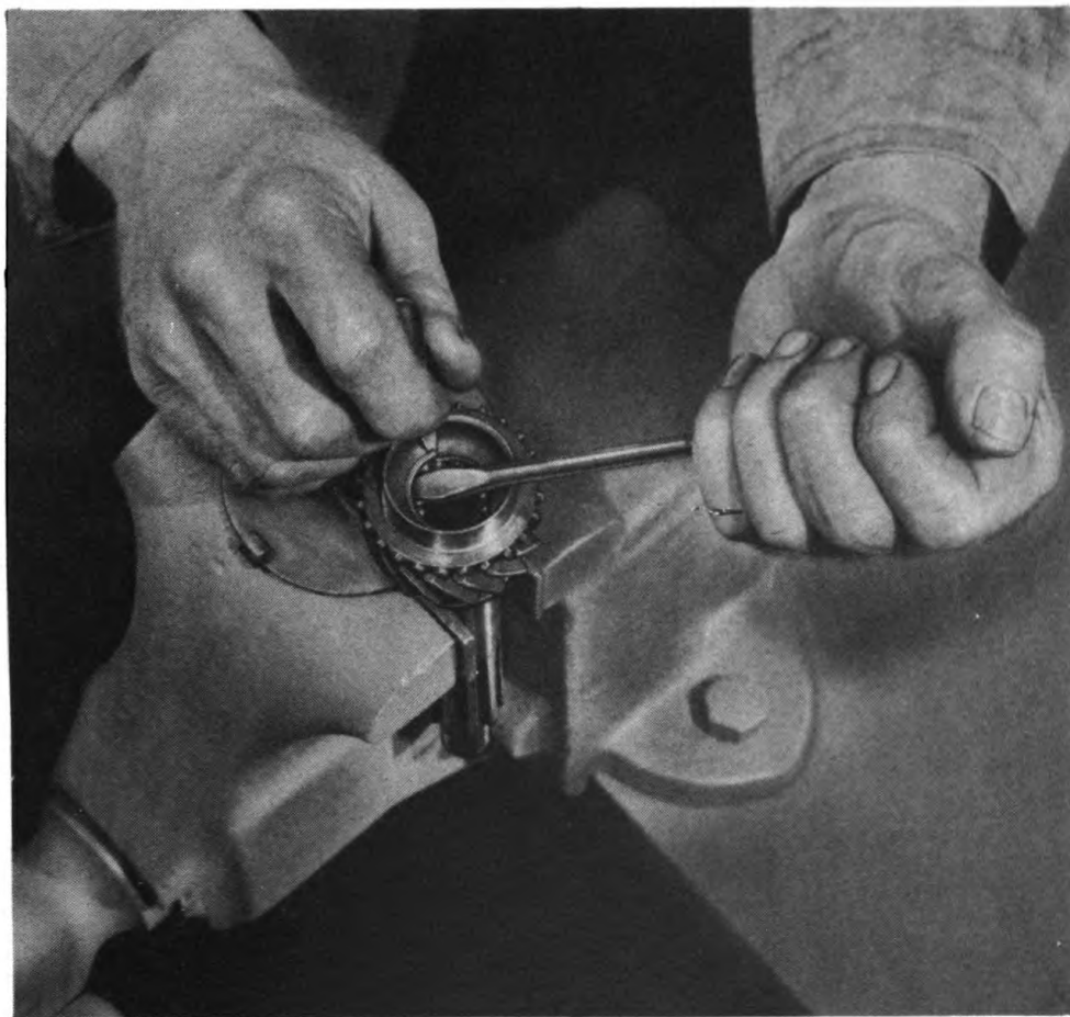
Figure 18—Pinion Bearing Rollers Lock Ring Removal
