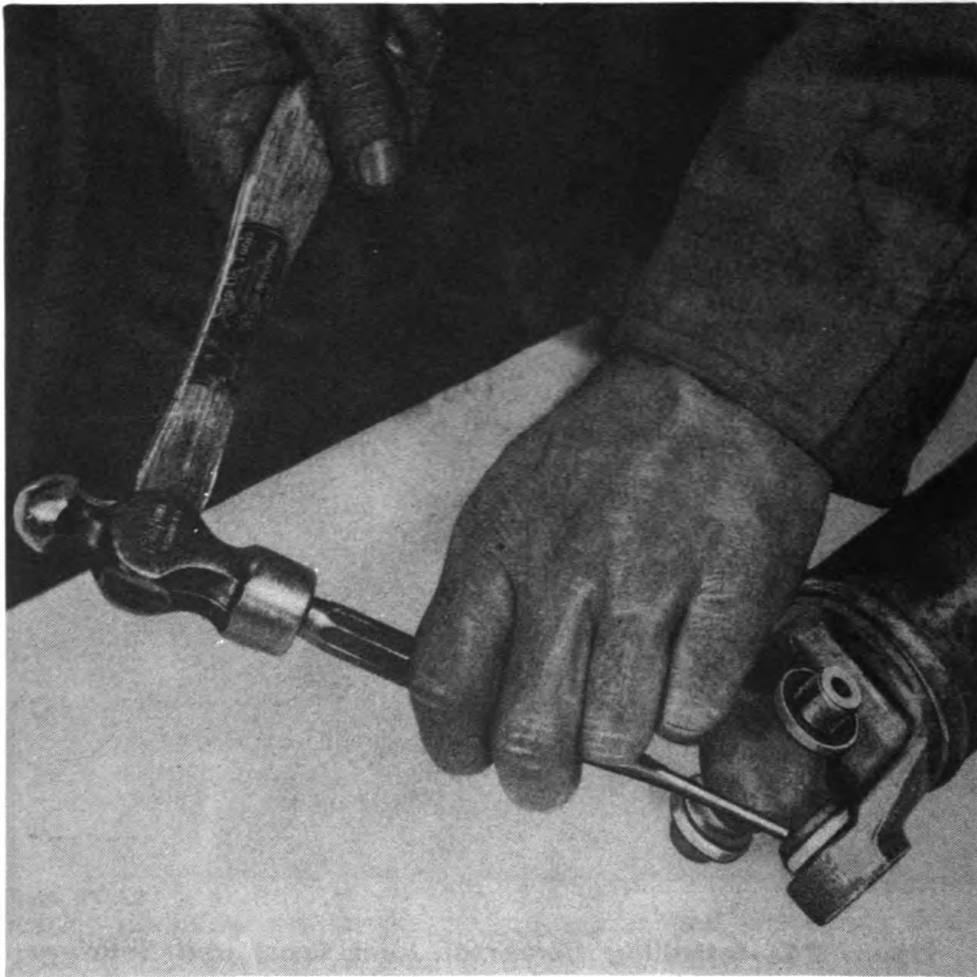
Figure 35—Eliminating Bind at Bearing Seals
