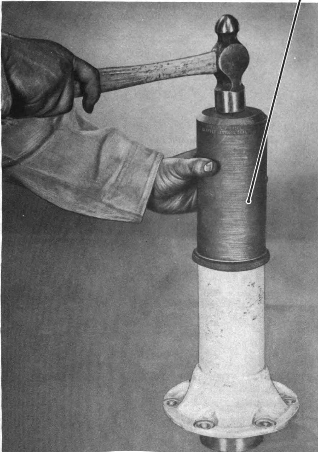
Figure 40—Installing Drive Wheel Carrier Oil Seal
