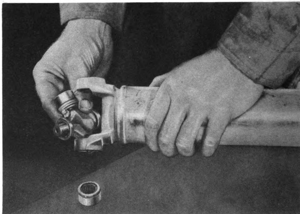
Figure 33—Universal Joint Cross Removal
