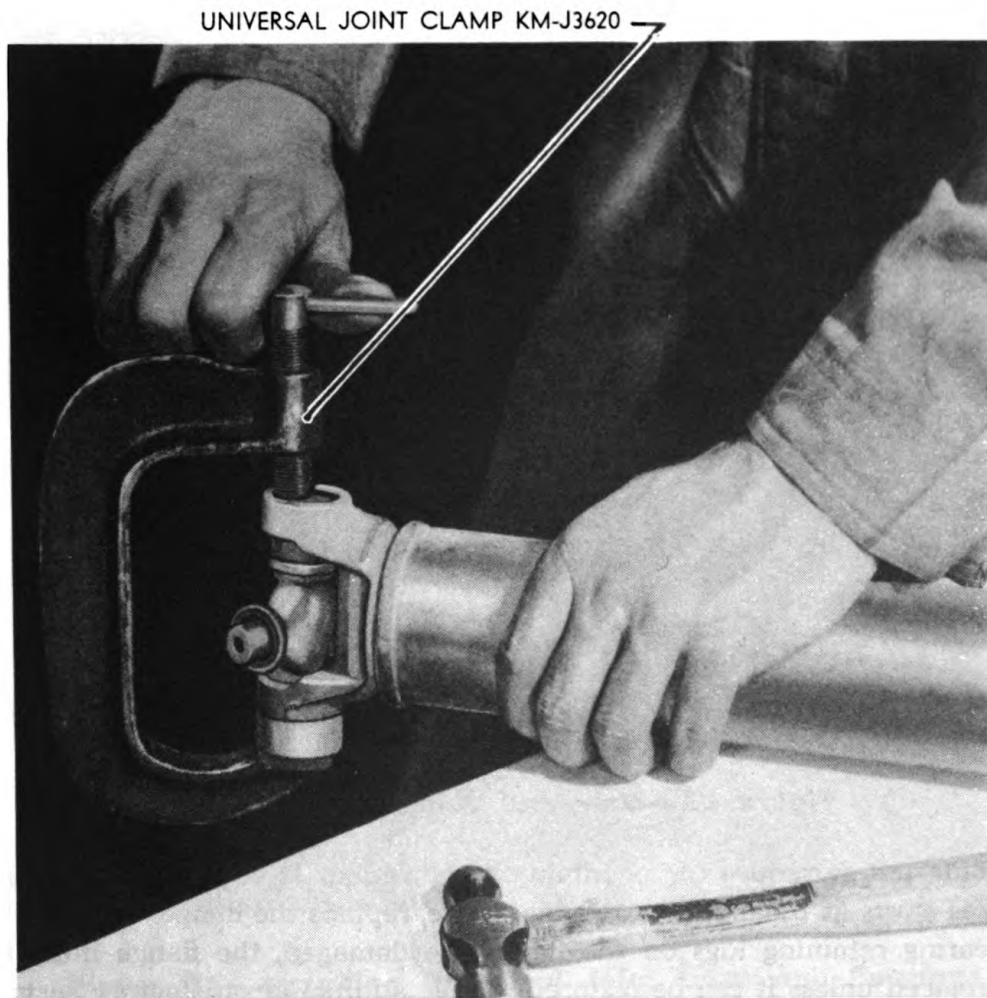
Figure 32—Method of Removing Universal Joint Bearings
