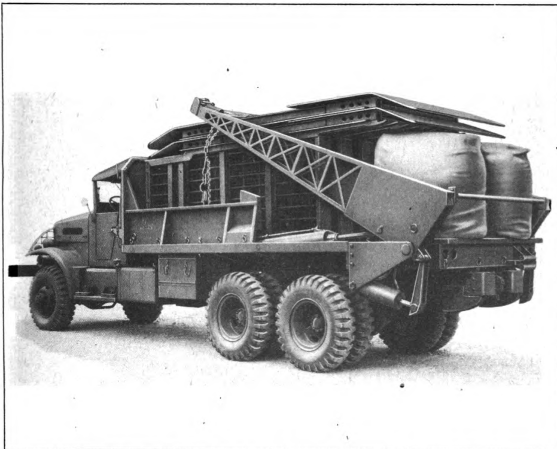
Figure 1. Hydraulic Bridge Erecting Crane with Typical Load
