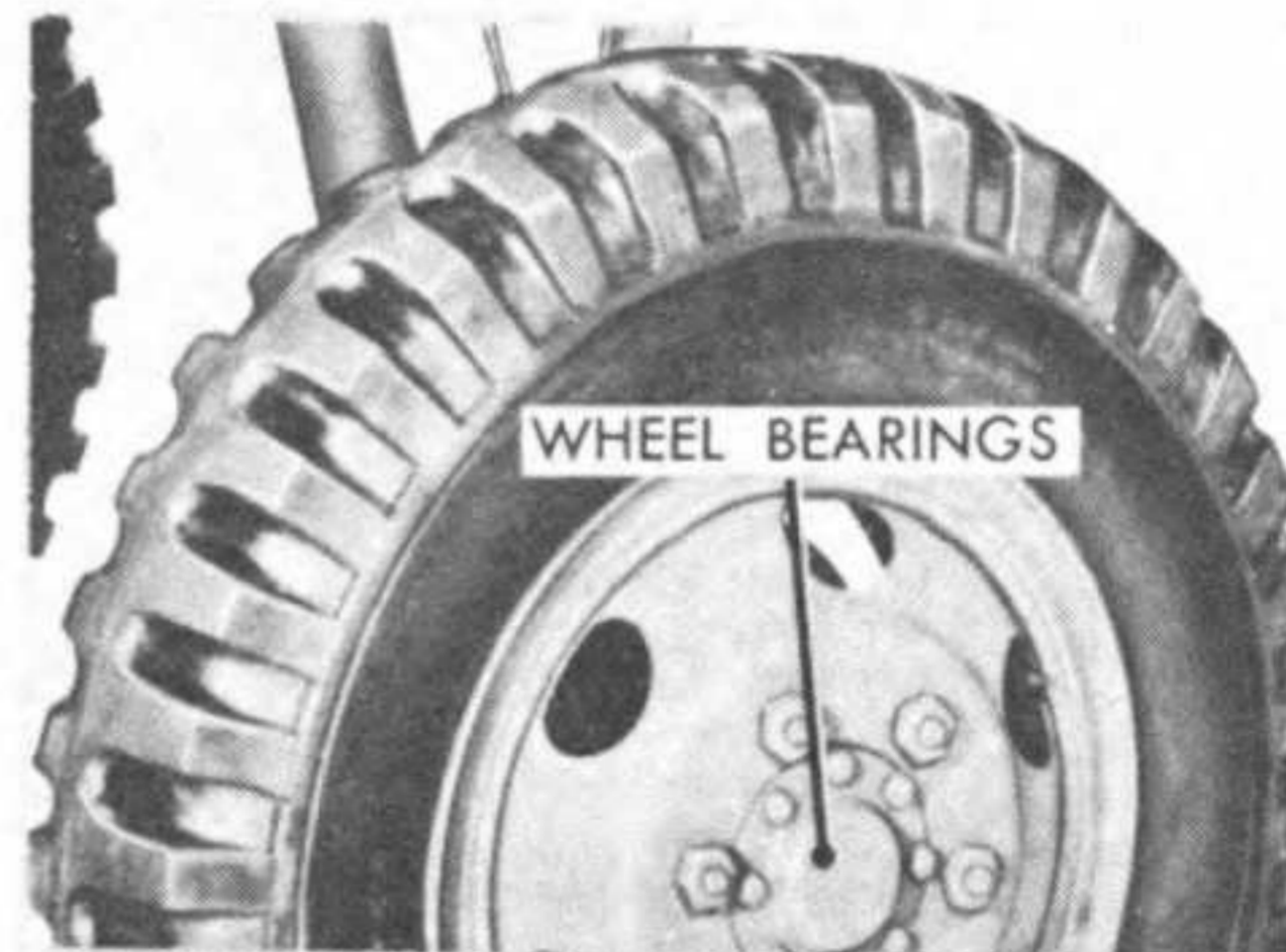
REFERENCE 6: Remove wheel, clean and inspect all parts, repack bearings and reassemble.
