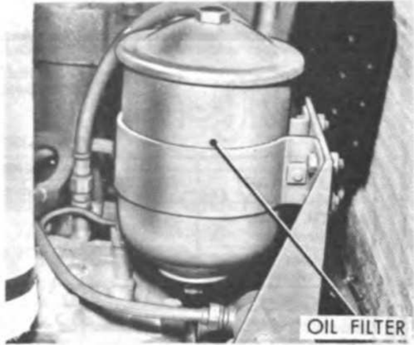
REFERENCE 2: Remove, clean housing, renew element, replace.
