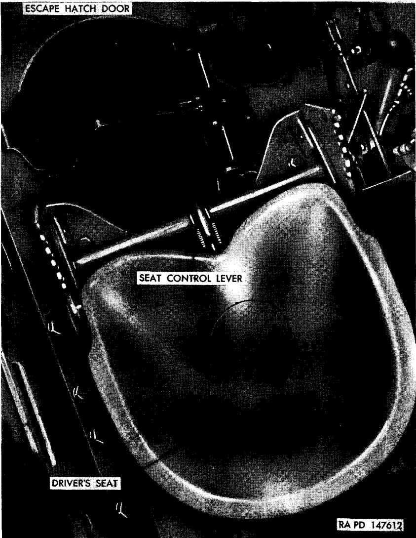
Figure 12. Driver's seat controls and escape hatch door.
