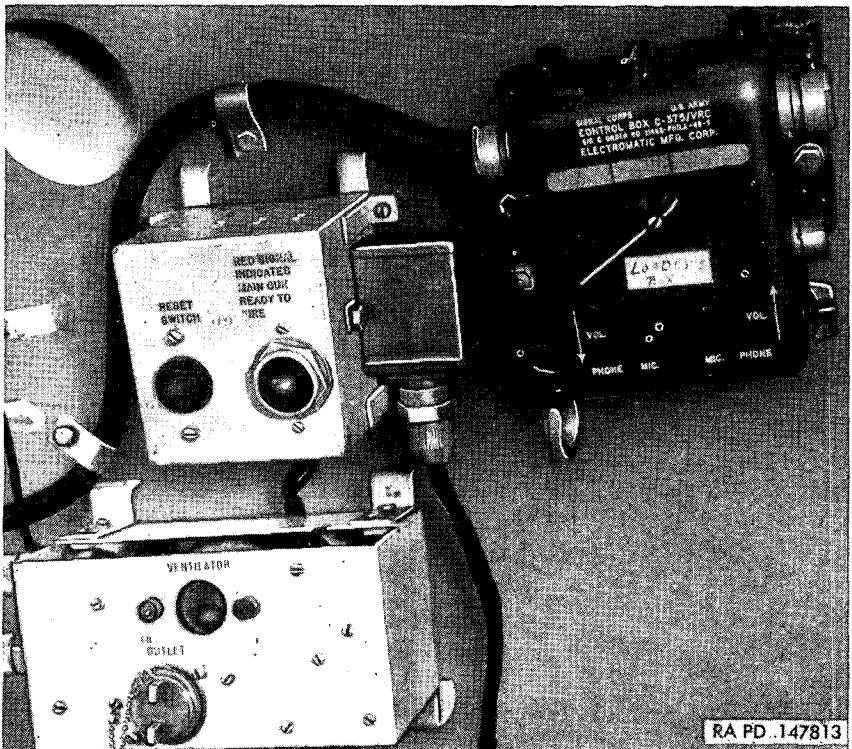
Figure 370. Loader's control box C-375/VRC.
