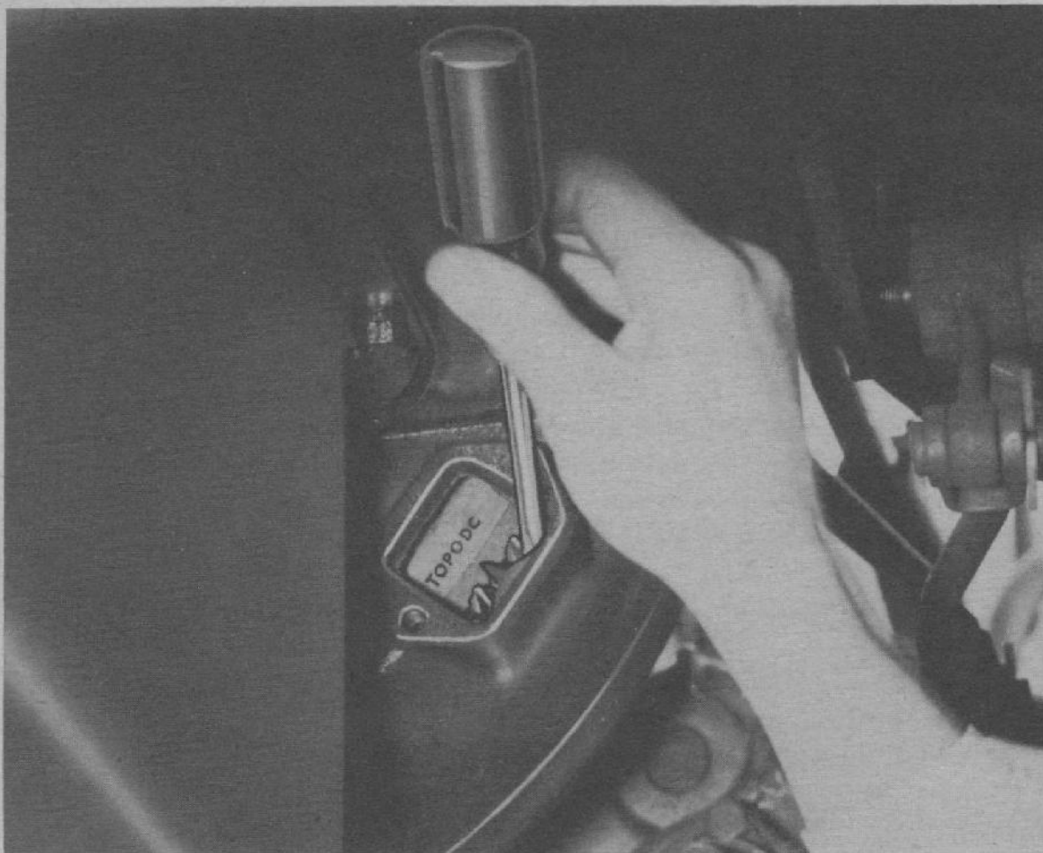
Figure 98—Timing Engine Flywheel
