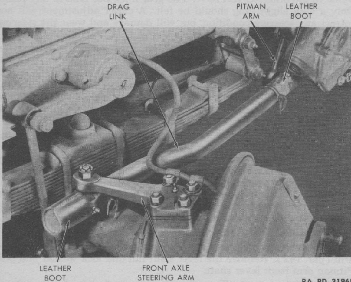
Figure 172—Removing Steering Pitman Arm
