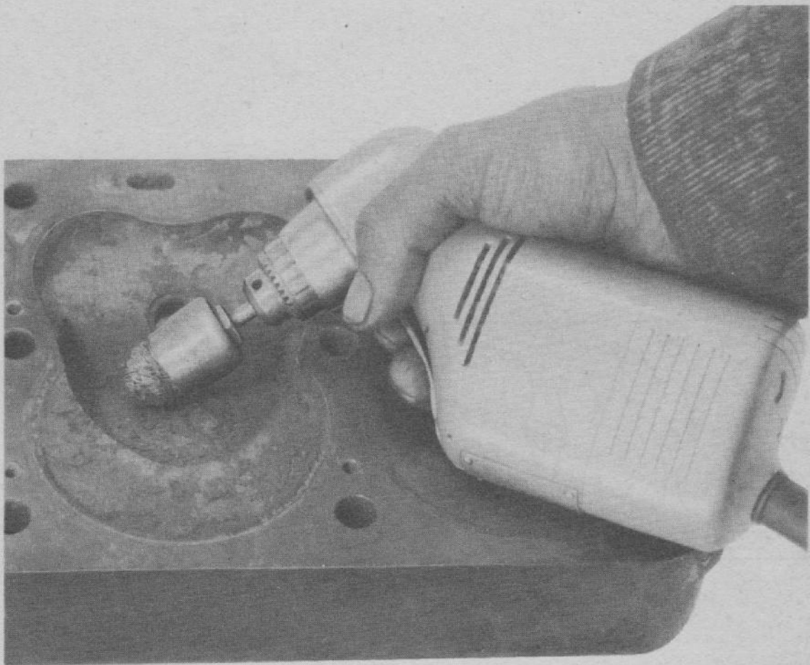
Figure 55—Removing Carbon from Cylinder Head
