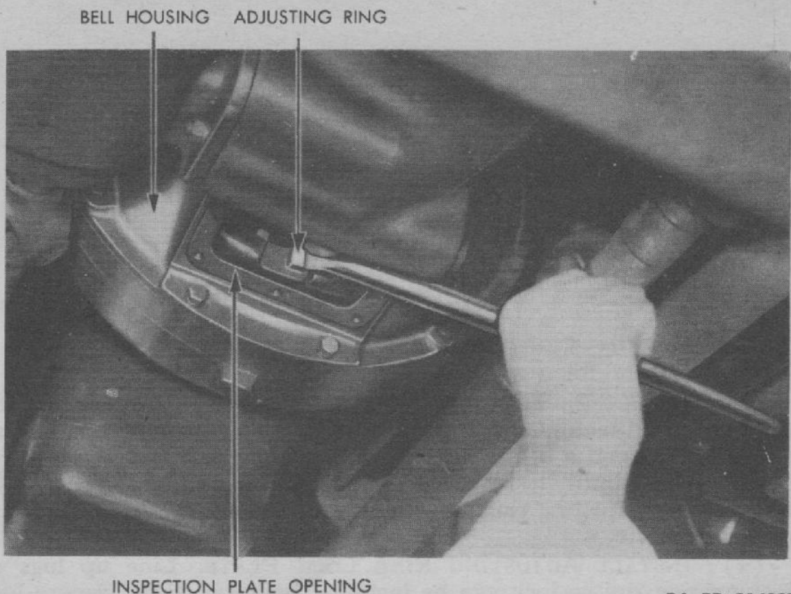
Figure 69—Turning Adjusting Ring
