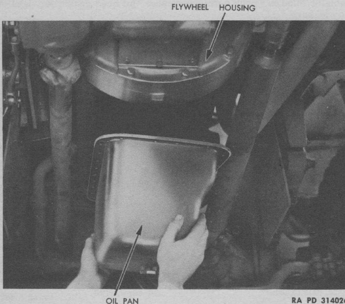
Figure 58—Removing Oil Pan
