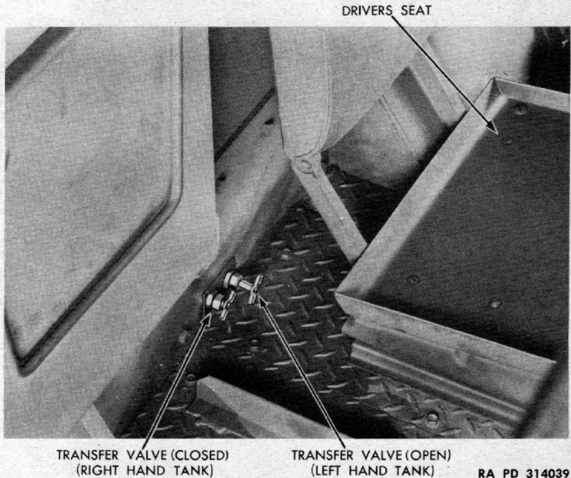
Figure 72—Fuel Tank Transfer Valve
