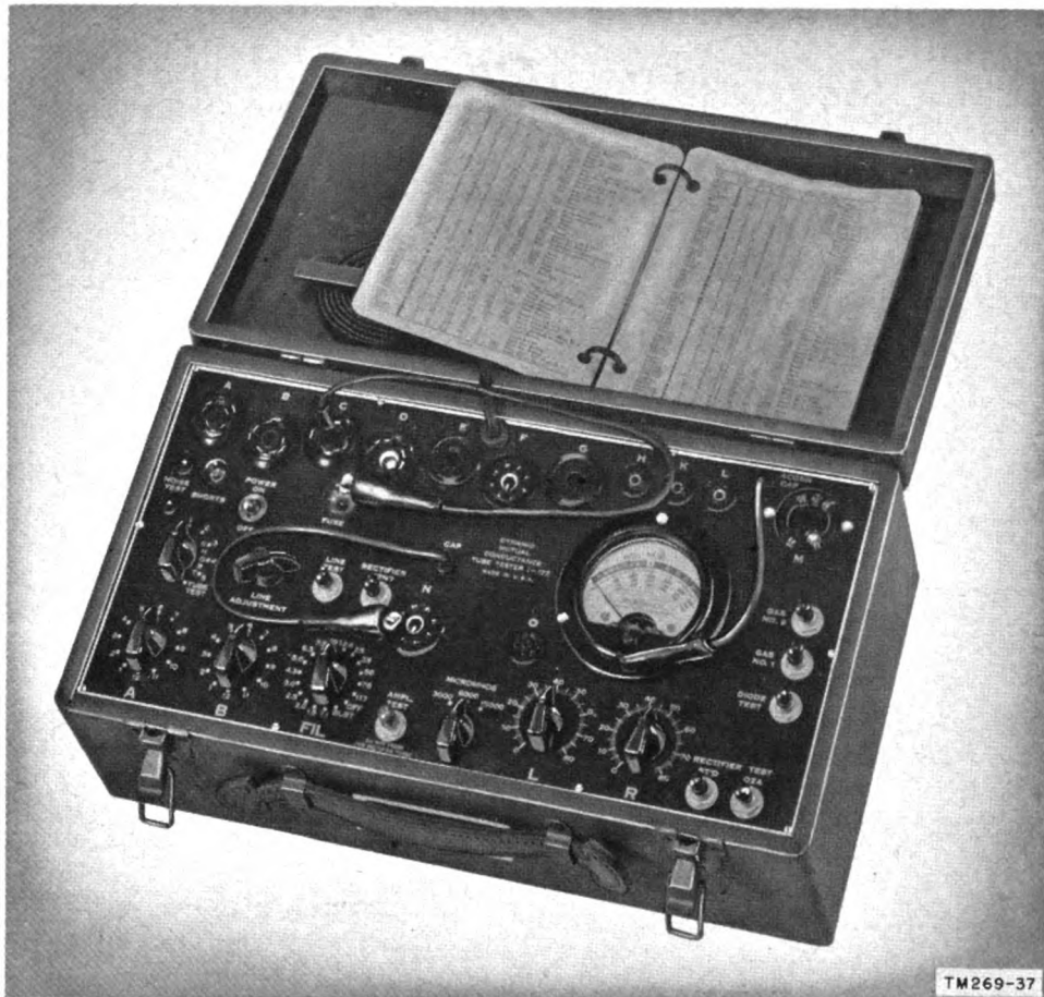
Figure 38. Tube tester I-177.
