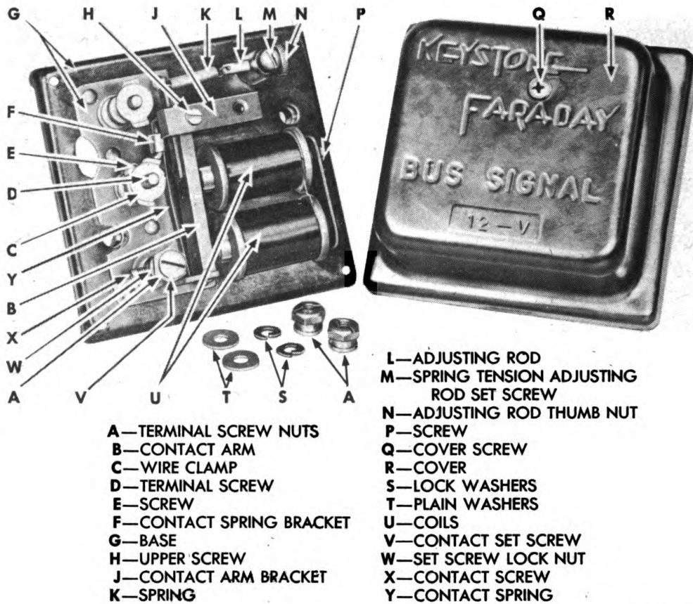
Figure 77 — Low-pressure Air Indicator Buzzer — Top View
