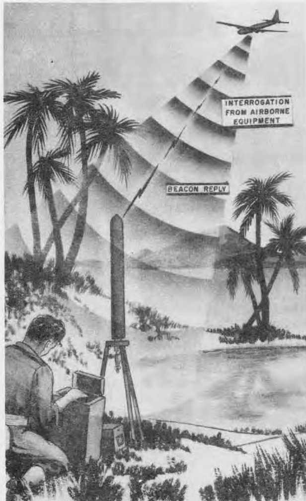
Aircraft Interrogation Triggers Beacon Reply which establishes its identity & position in range and azimuth. July 1945
