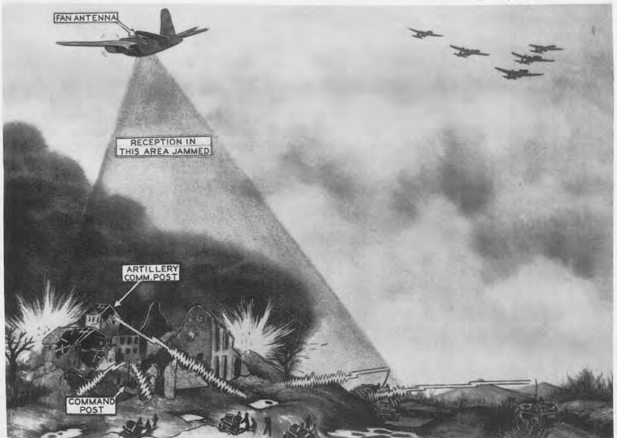
Radio Transmitting Set AN/ART-7 is an airborne jammer used to disrupt enemy ground radio communications operating with-in its frequency range.
