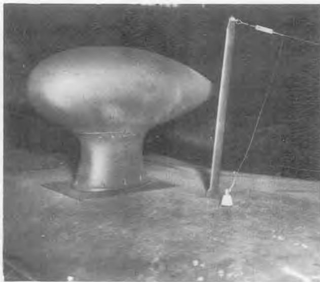
Loop and Loop Housing for AN/ARN-7 installed in fuselage above pilot and co-pilot on C-64 aircraft.
