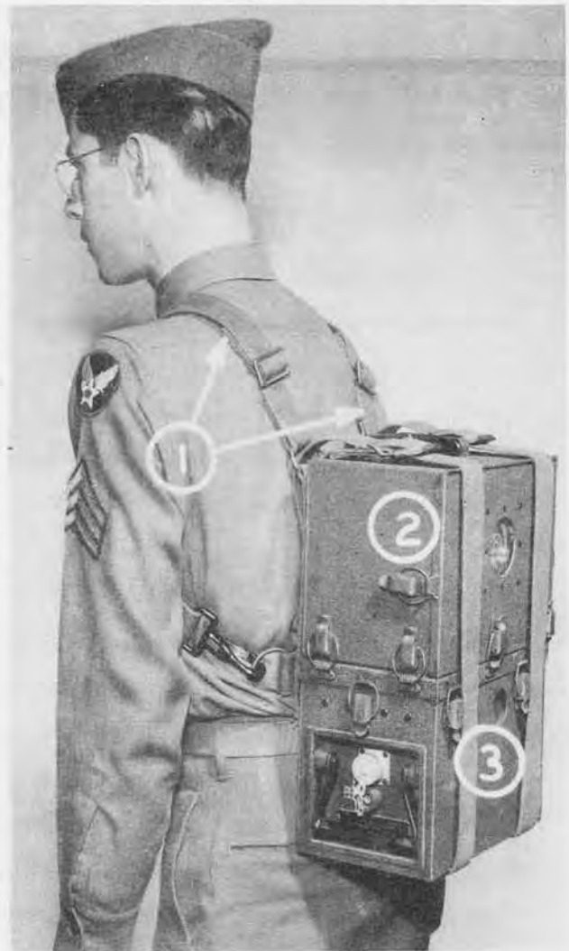
Battery Charger & Battery in carrying position-entire equipment may be packed in 2 packages & carried by one man. (1) Harness MX-253/UPN-1 (2) Rectifier Battery Charger PP-116/UPN (3) Battery Case CY-222/UPN-1.
