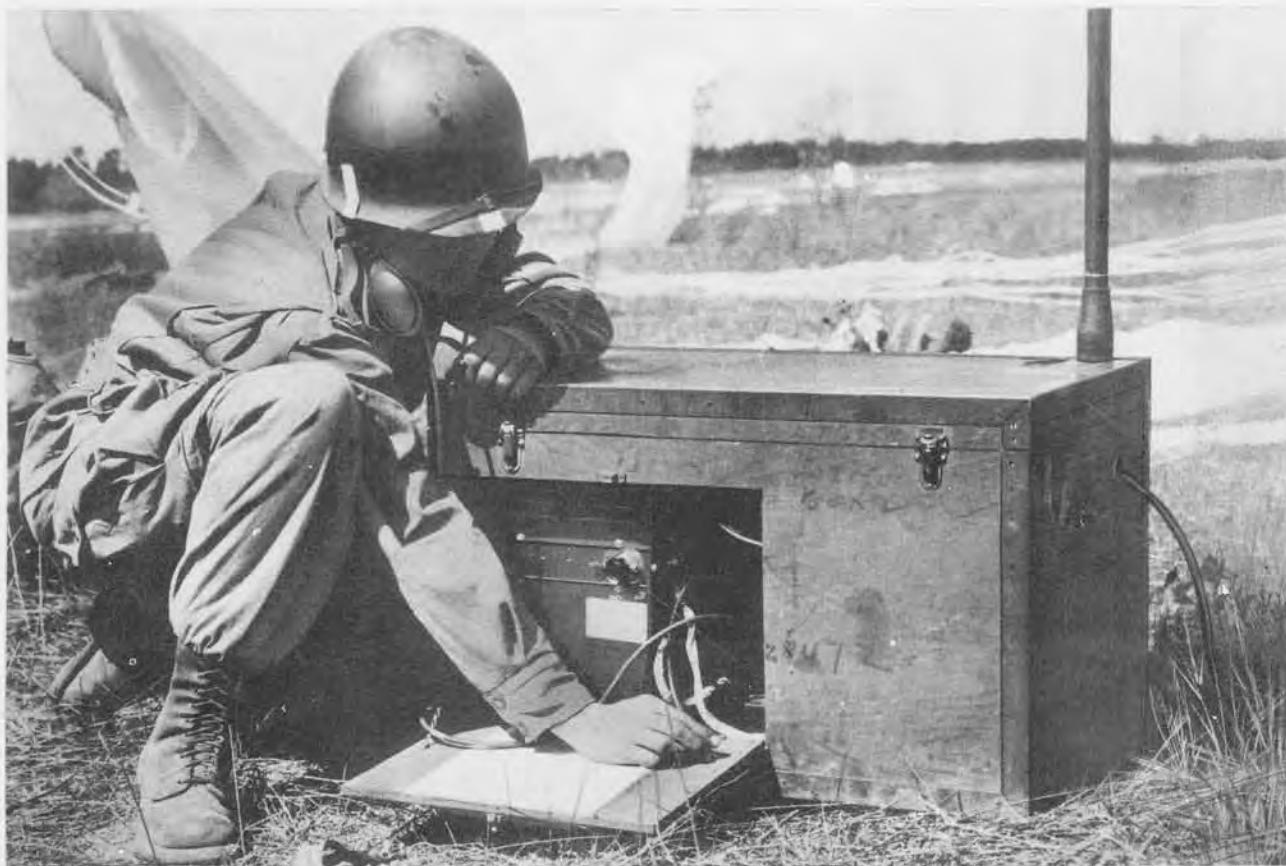
Beacon Transmitter AN/TPN-3 is an air transportable Radar Beacon providing homing facilities to troop carrying aircraft under conditions of poor visibility.
