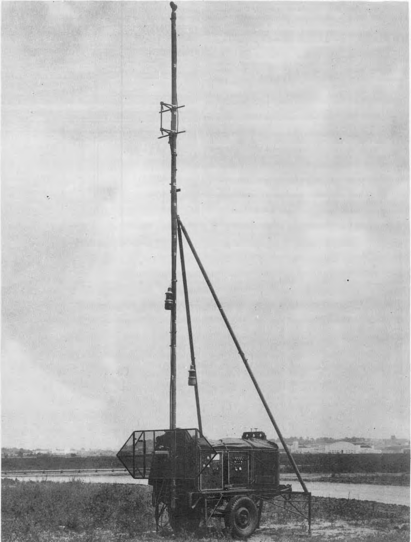
In operation Radio Set AN/CRN-2 is located approximately 750 feet from the approach end of the runway and 400 feet to one side (or the other) of the runway's center line.
