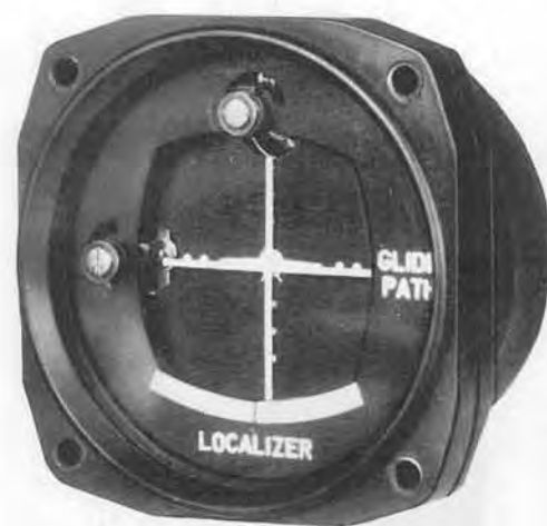
The Vertical Pointer of Indicator I-101 records position of aircraft with regard to alignment to runway.
