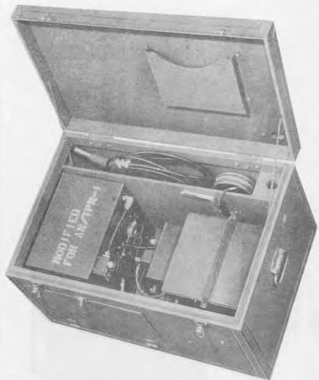
AN/TPN-1 packed in Case CY-21/TPN-1 is air transportable and easily assembled.
