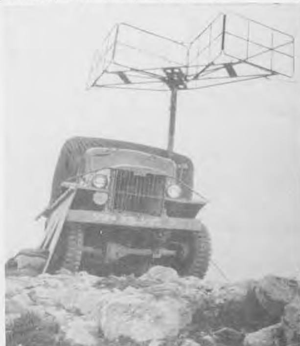
Radio set AN/CPN-2 should be placed on the highest terrain available and away from surrounding hills or buildings.
