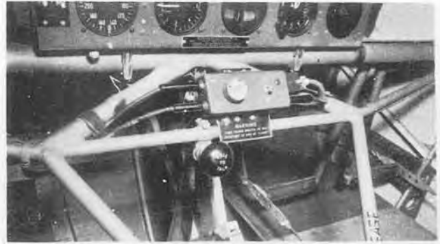
Installation of Control Box and "pull to talk" switch on instrument panel, pilots position in CG-4A glider.
