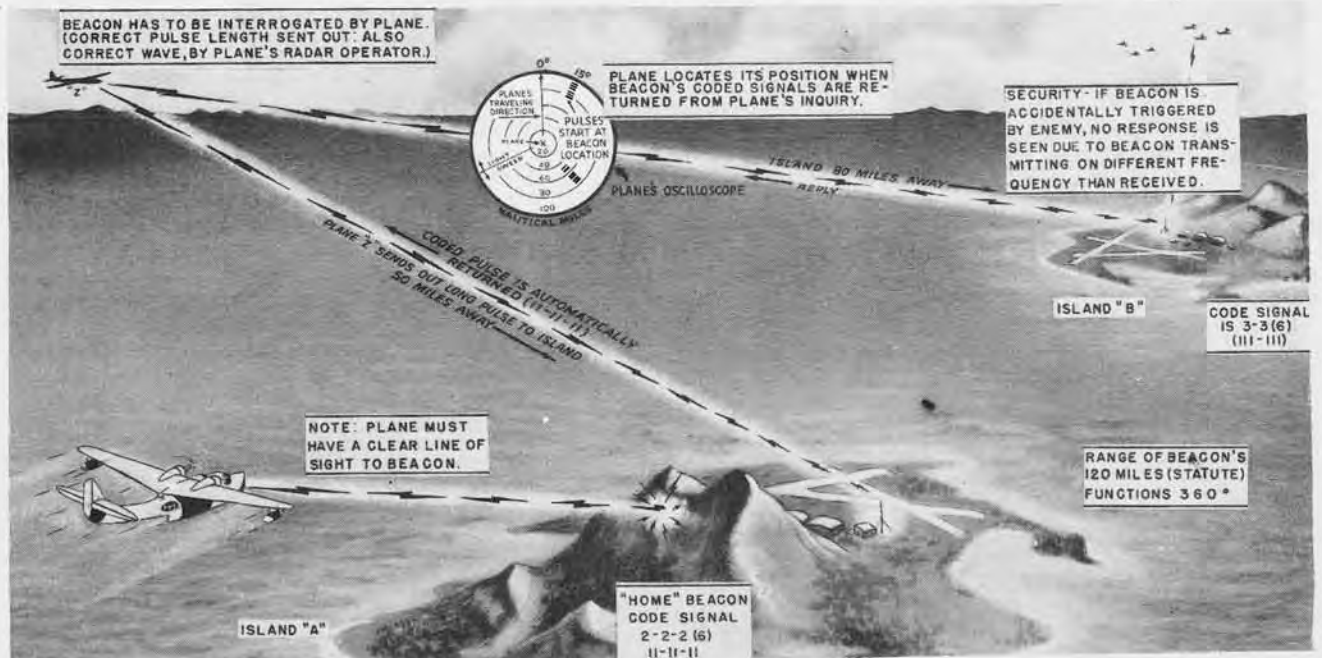
Radio Set AN/CPN - 8 is an Air Transportable Radar Beacon designed to provide range, direction, and identification for homing 10 cm band radar equipped aircraft.
