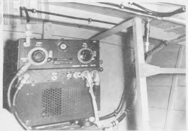
Receiver-Transmitter RT-21/APN-7 installed for operation.
