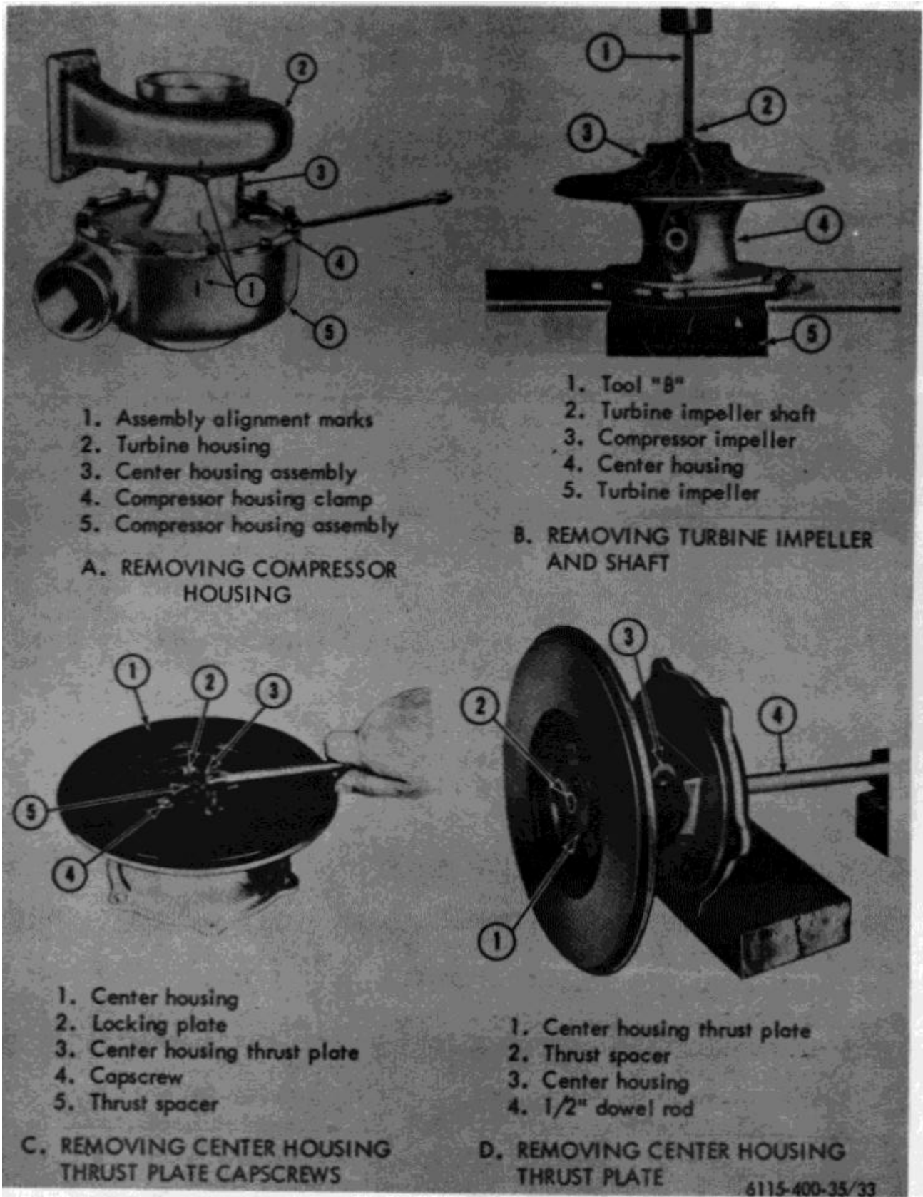
Figure 33. Turbocharger disassembly.
