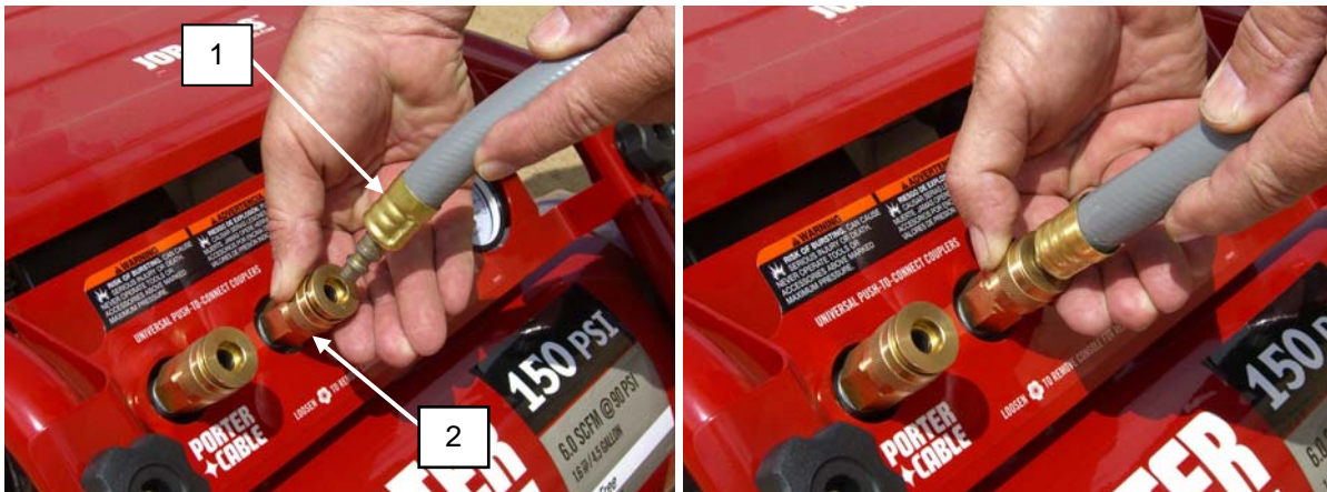
Figure 53. Disconnect Adapter Hose from Air Compressor.
