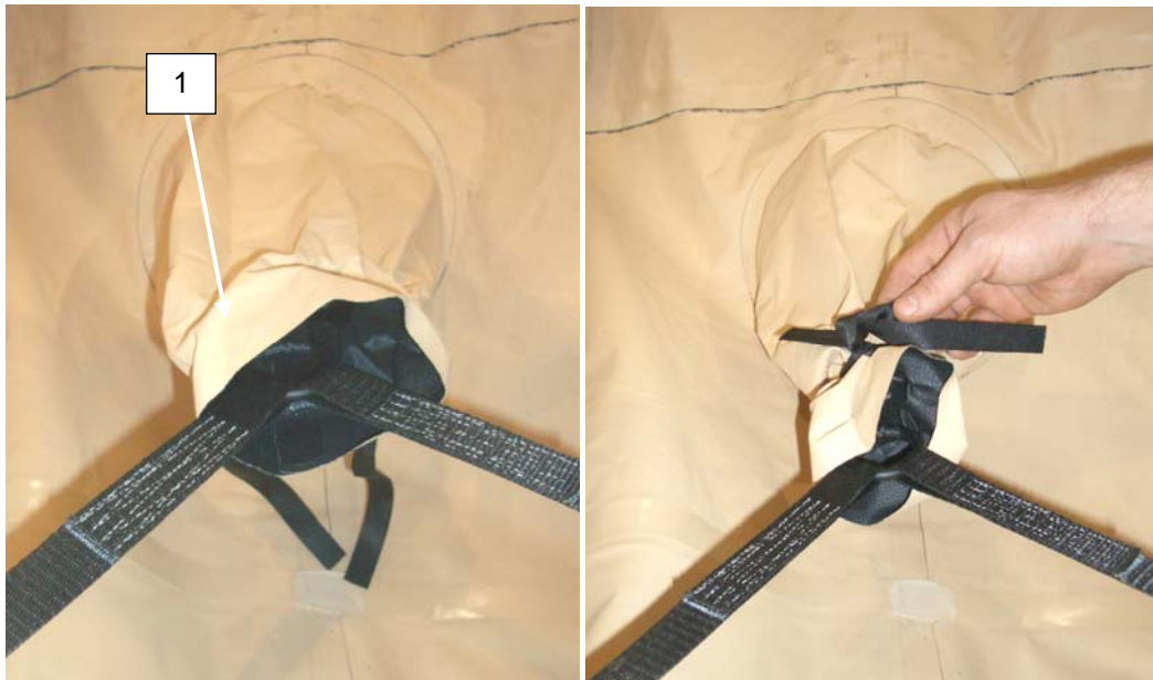
Figure 9. Wrap and Tie External Tensioning Snouts.
