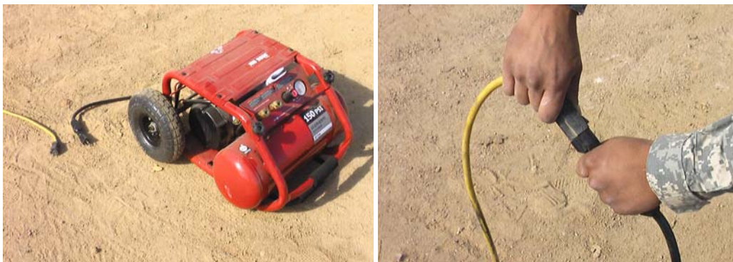
Figure 31. Connect Air Compressor to Power Source.
