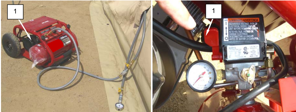
Figure 2. Set Air Compressor On/Auto/Off Lever to OFF.
