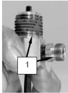
Figure 10. Apply Sealant to Check Valve Threads.
