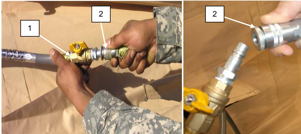
Figure 4. Disconnect Air Compressor Hose from Inflation Hose.
