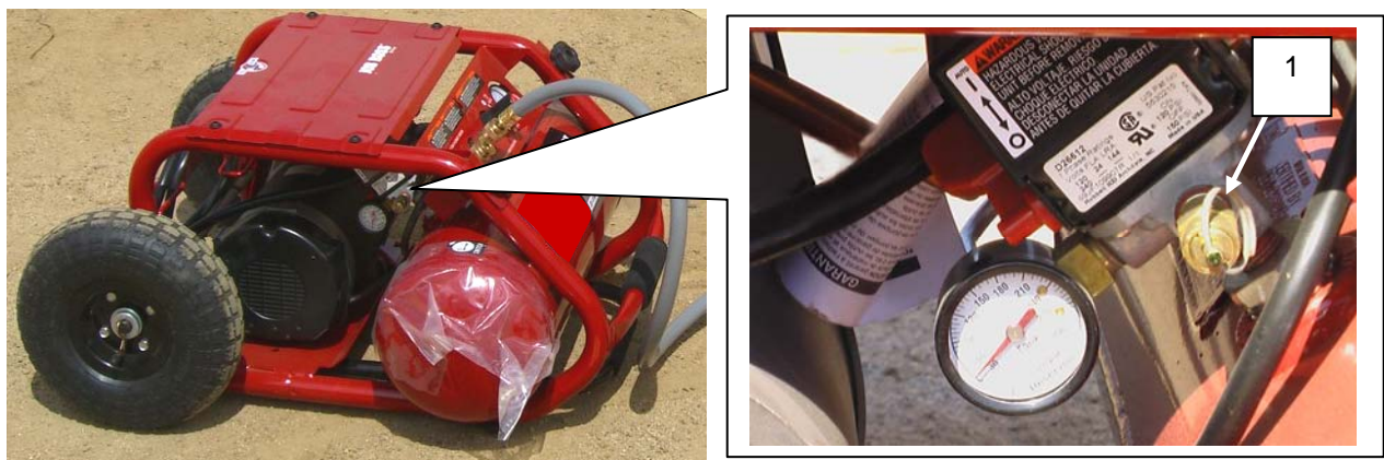
Figure 1. Air Compressor Safety Valve Ring.
