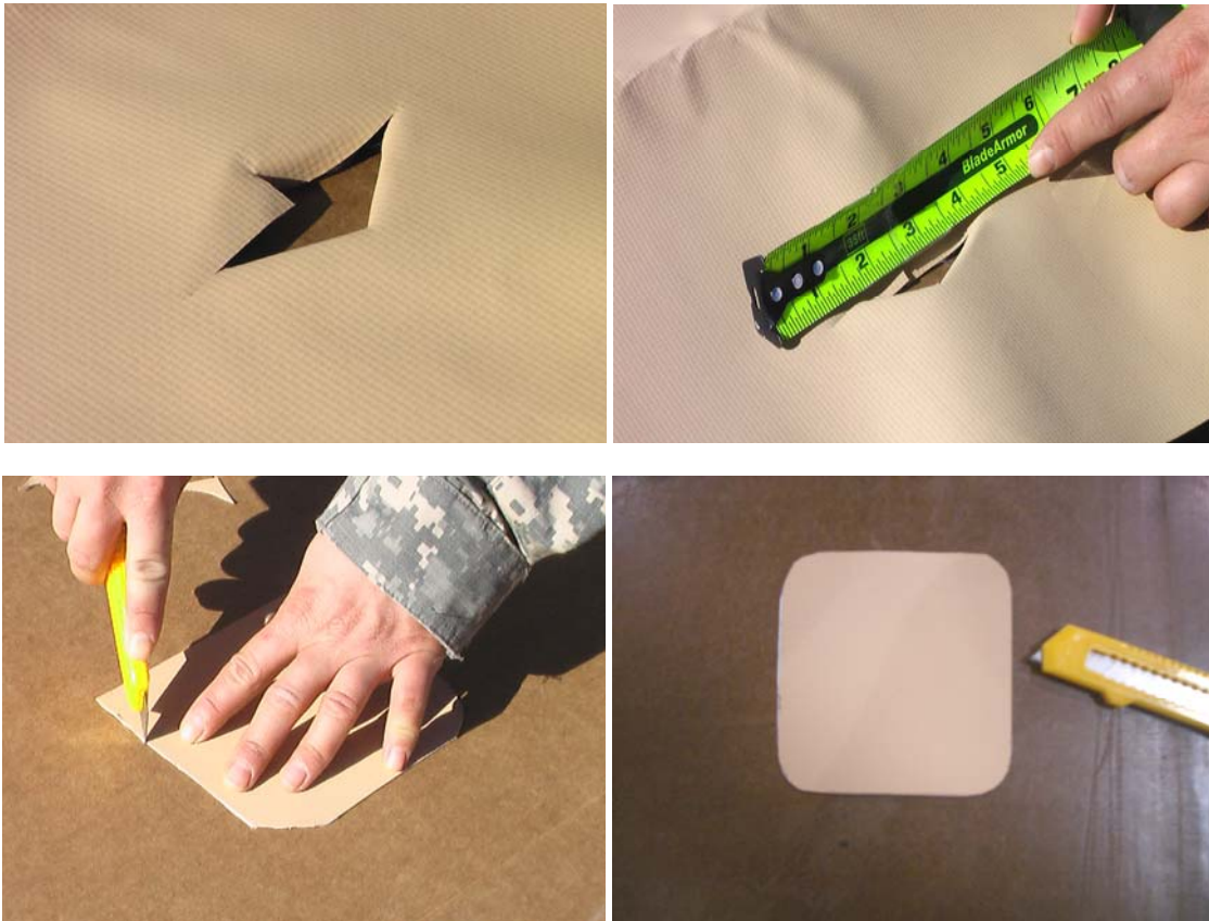
Figure 3. Measure and Cut Temporary Patch.
