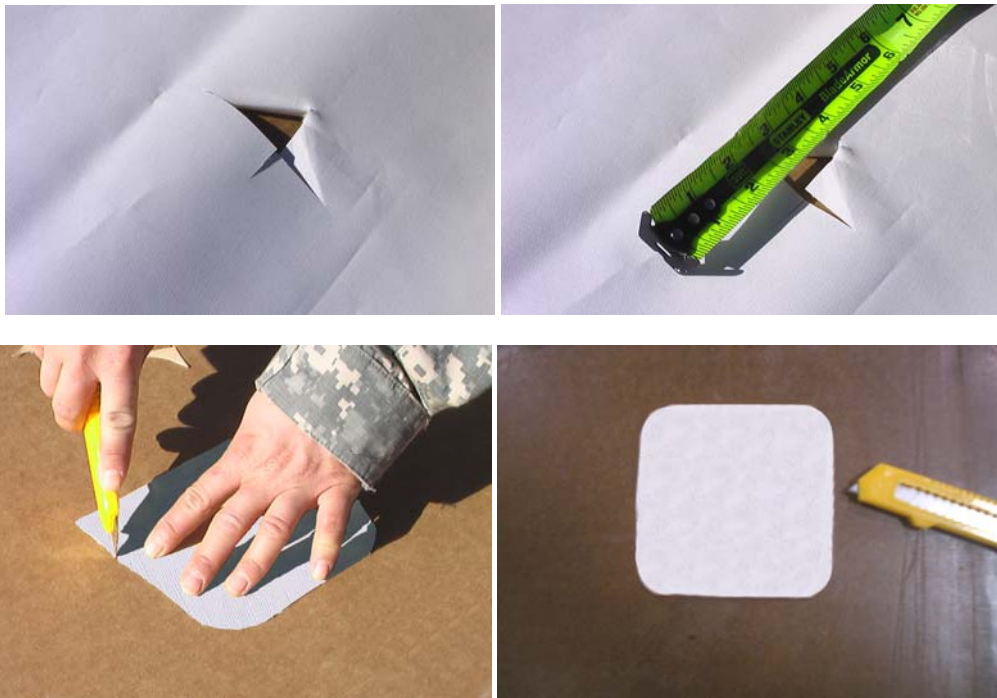
Figure 3. Measure and Cut Temporary Patch.
