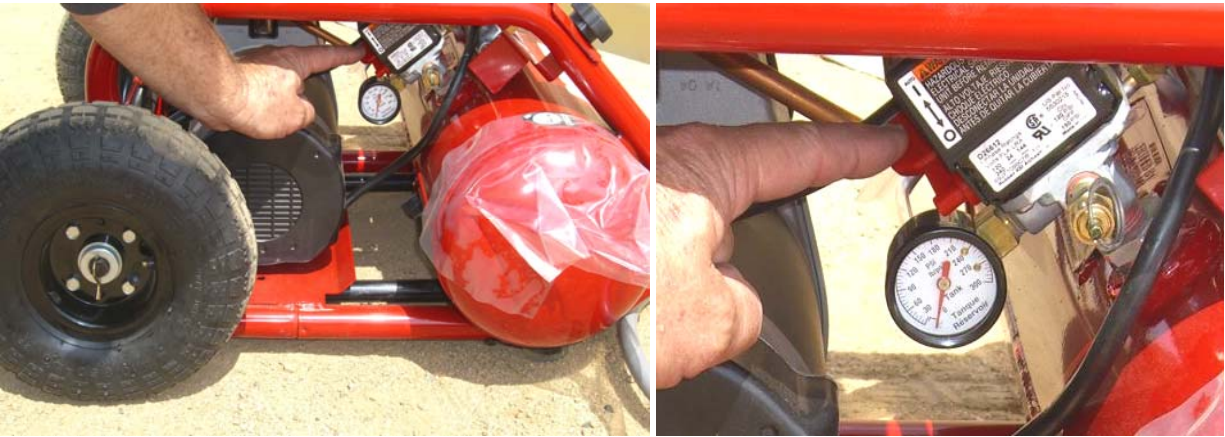
Figure 48. Turn Off Air Compressor.
