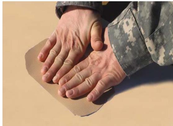
Figure 14. Remove Air Pockets from Patch.
