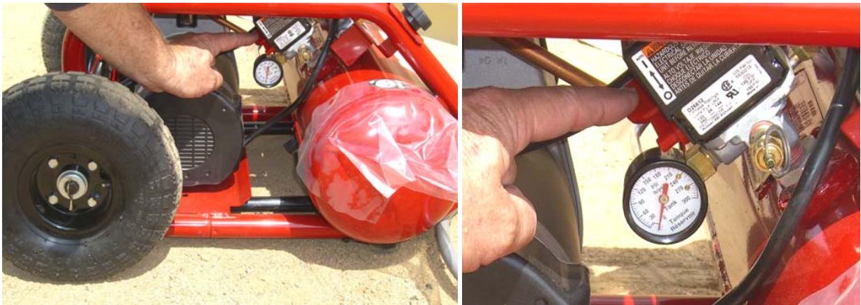
Figure 42. Turn On Air Compressor.
