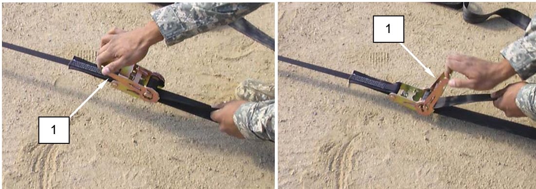
Figure 14. Tighten Upper Ratchet External Bracing Strap with Tensioning Ratchet.
