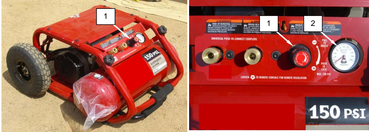
Figure 2. Set Regulator Outlet Pressure to Zero.
