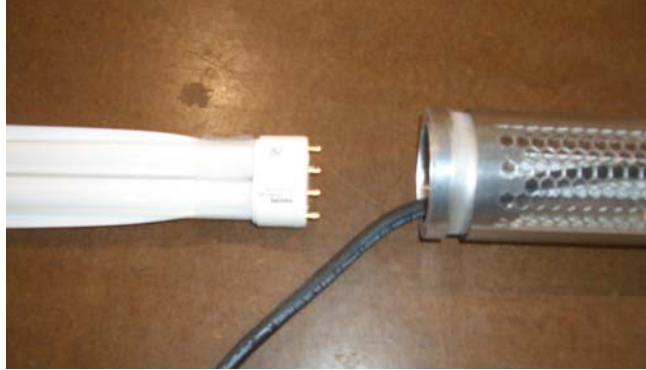
Figure 13. Insert Replacement Fluorescent Bulb into Outer Tube.
