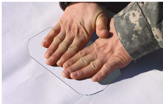
Figure 15. Remove Air Pockets from Patch.
