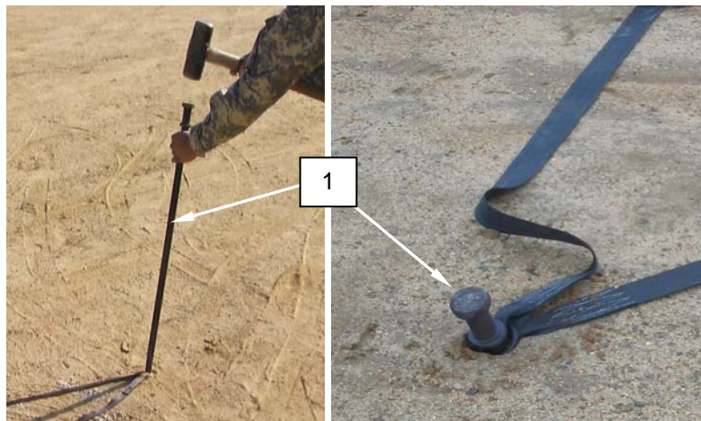
Figure 6. Position Bracing Strap End Rings.
