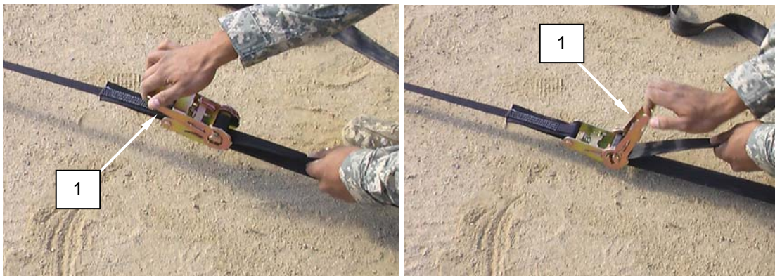
Figure 17. Tighten Upper Ratchet External Bracing Strap with Tensioning Ratchet.
