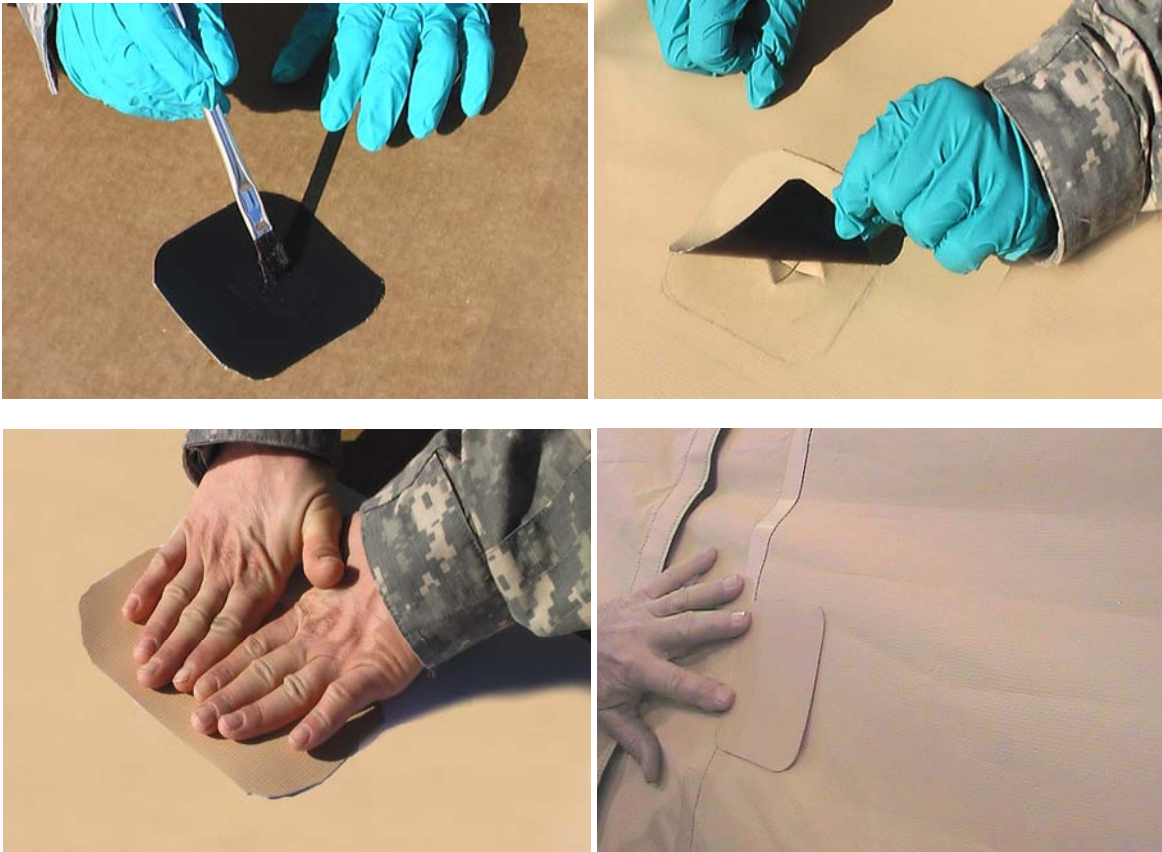
Figure 13. Applying Permanent Patch to Damaged End Section.
