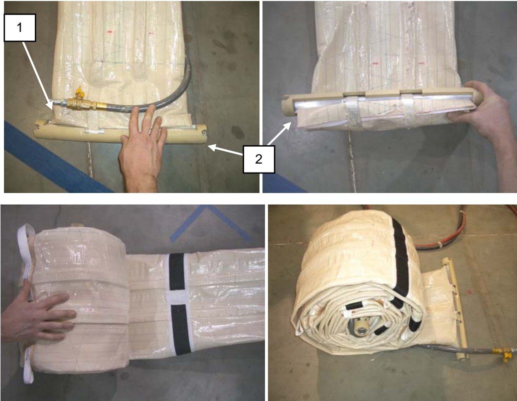
Figure 12. Rolling Up the Airbeam.
