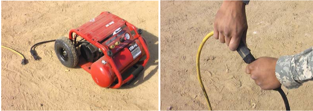
Figure 3. Connect Air Compressor to Power Source.
