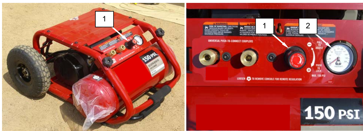
Figure 3. Set Regulator Outlet Pressure to Zero.
