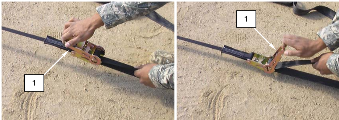
Figure 11. Tension Lower Ratchet External Bracing Straps.
