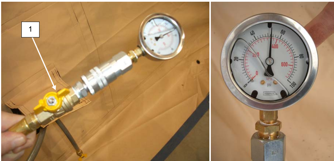
Figure 11. Open Deflation Air Hose Ball Valve.
