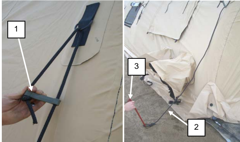
Figure 16. Remove Side Ropes and Tent Pins.
