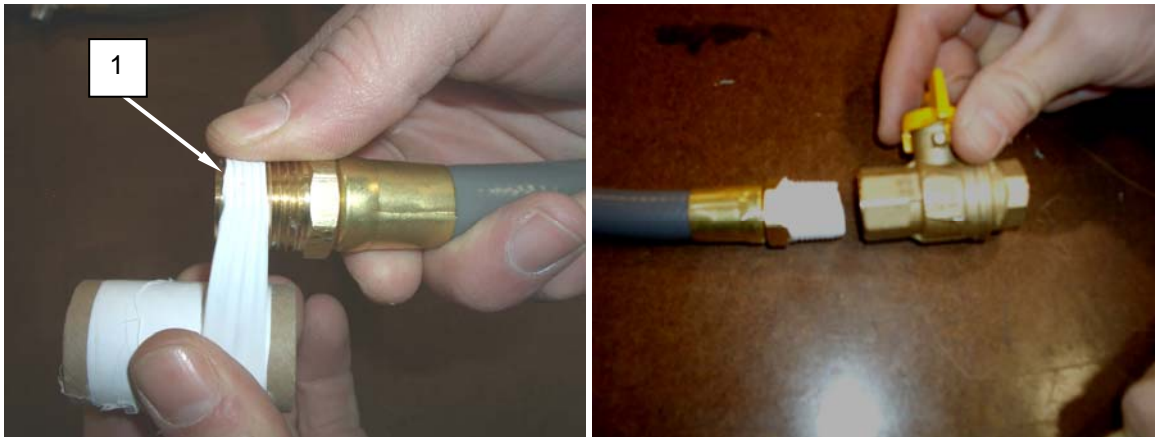
Figure 6. Wrap Airbeam Inflation Hose Fitting Threads with Thread Sealant Tape.
