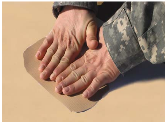
Figure 12. Remove Air Pockets from Patch.
