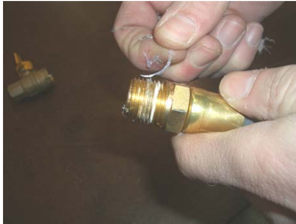
Figure 5. Remove Debris from Airbeam Inflation Hose Fitting Threads.
