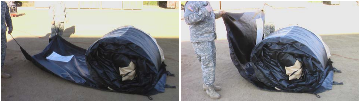
Figure 41. Wrap Transport Cover over Tent.
