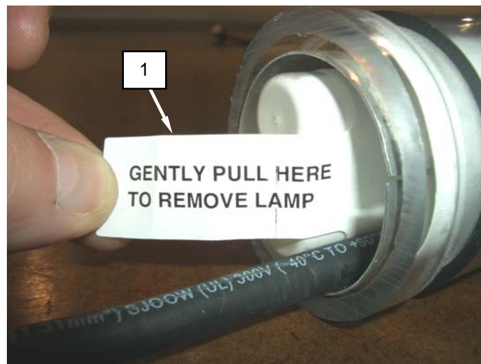
Figure 10. Grasp Bulb Puller and Remove Fluorescent Bulb.
