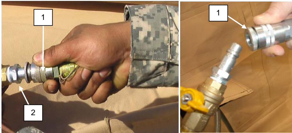
Figure 50. Disconnect Inflation Air Hose from Adapter Hose.
