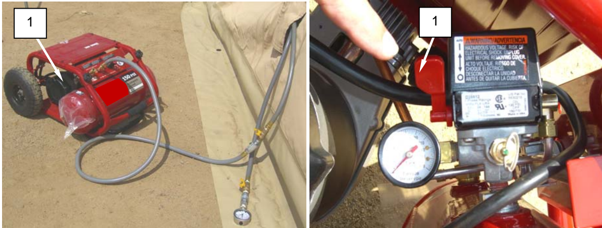
Figure 10. Set Air Compressor On/Auto/Off Lever to ON.
