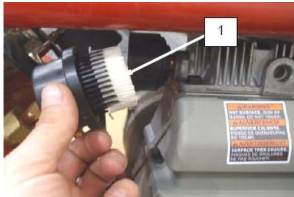
Figure 11. Replace Air Filter in Air Filter Cover.
