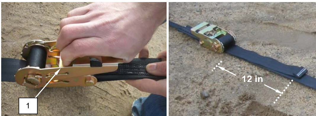
Figure 41. Tensioning Ratchet Strap Excess.
