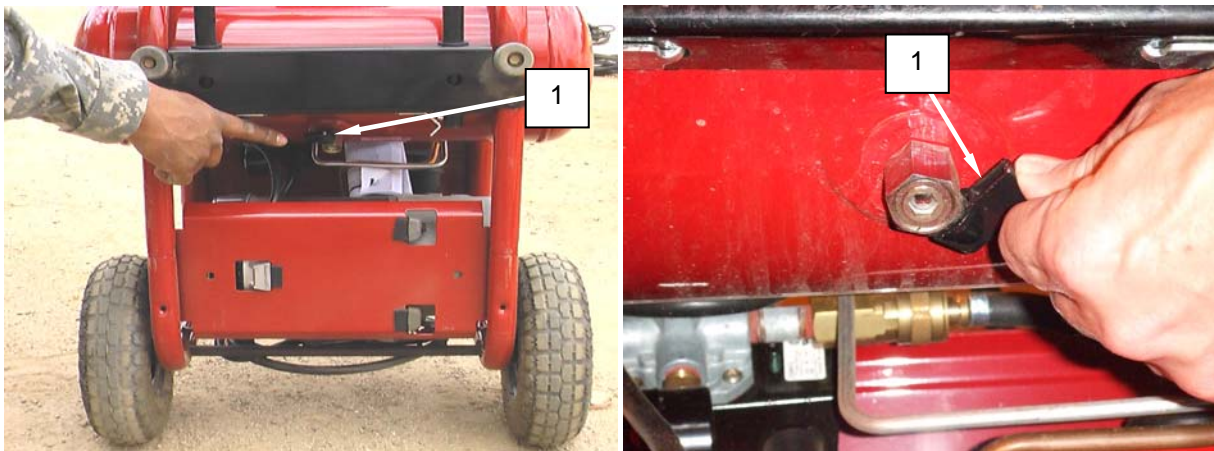
Figure 6. Close Air Tank Drain Valve.
