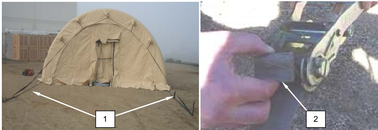
Figure 56. Door End External Bracing Straps.
