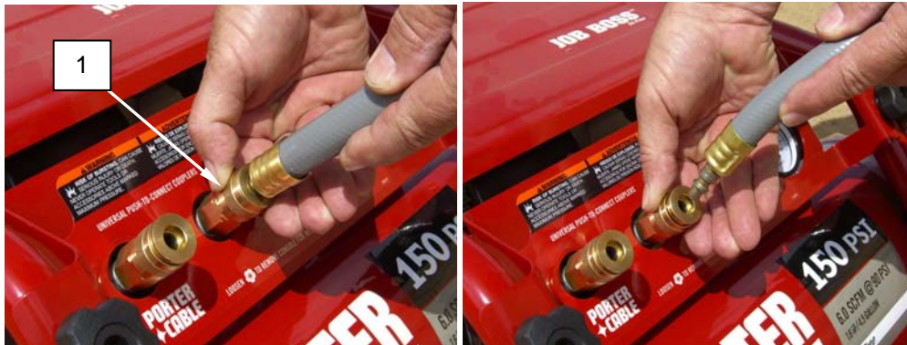
Figure 4. Disconnect Tools or Accessories from Air Compressor QD Fittings.
