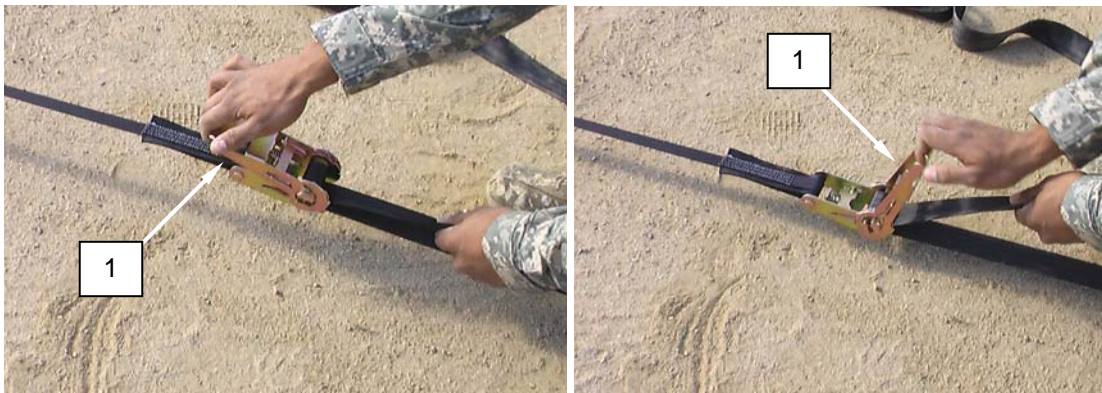
Figure 16. Remove Slack From Lower Ratchet External Bracing Strap.
