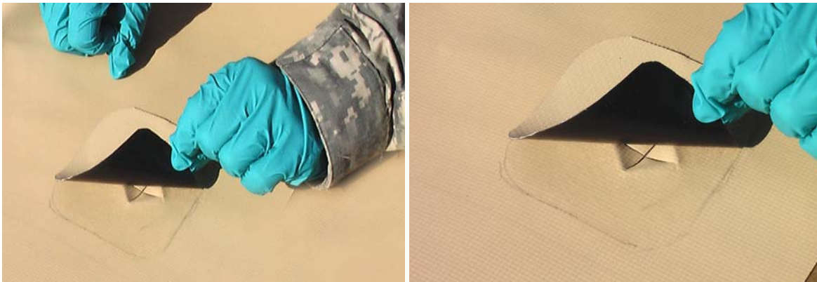
Figure 13. Apply Patch to Damaged Area.
