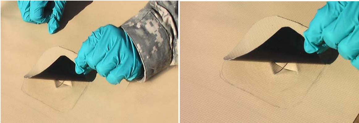
Figure 11. Apply Patch to Damaged Area.
