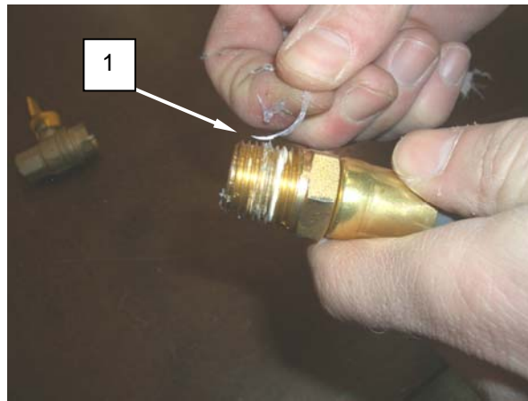
Figure 7. Remove Debris from Manifold Hose Fitting Threads.
