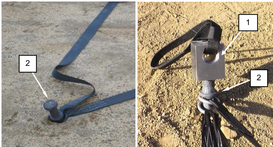
Figure 4. Stake Removal Tool.
