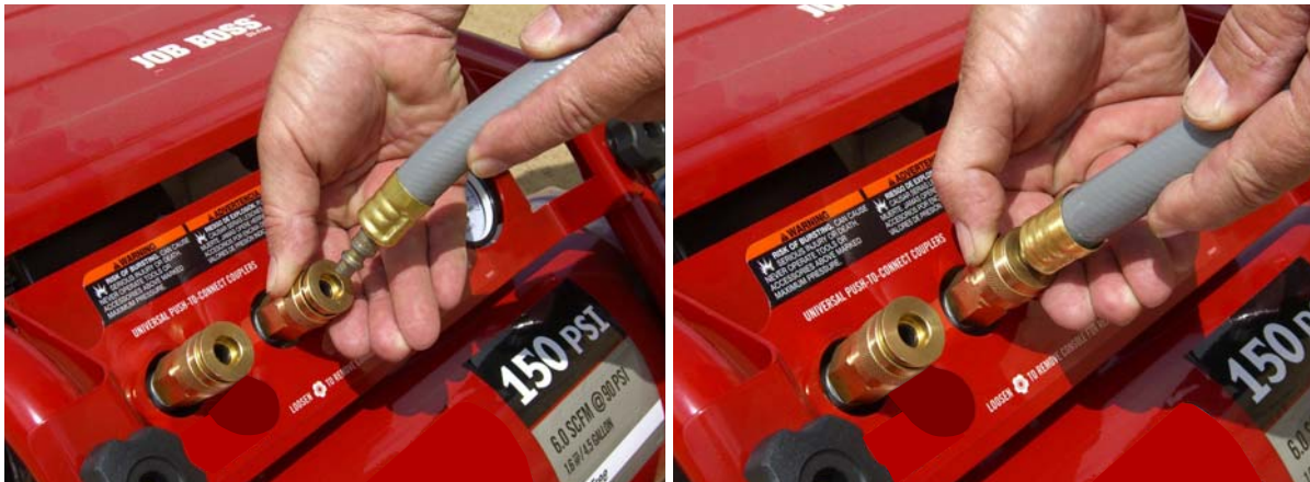
Figure 32. Connect Air Compressor Hose to Air Compressor.
