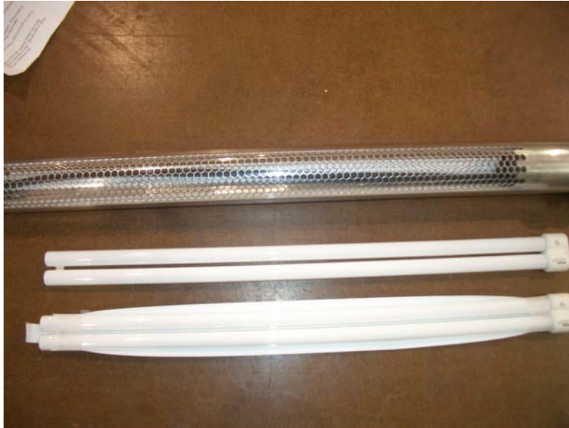
Figure 11. Outer Tube, Bulb and Replacement Fluorescent Bulb.
