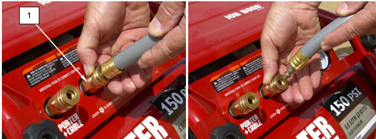
Figure 3. Disconnect Hoses from Air Compressor QD Fittings.
