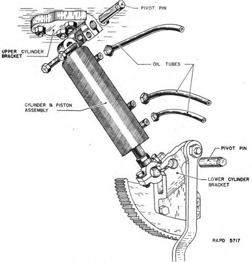
FIGURE 79.—Piston and cylinder.
