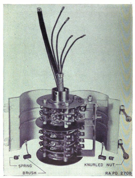
FIGURE 84 .- Collector ring assembly.
