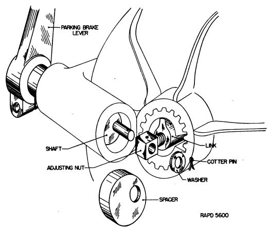
FIGURE 43.—Parking brake adjustment.
