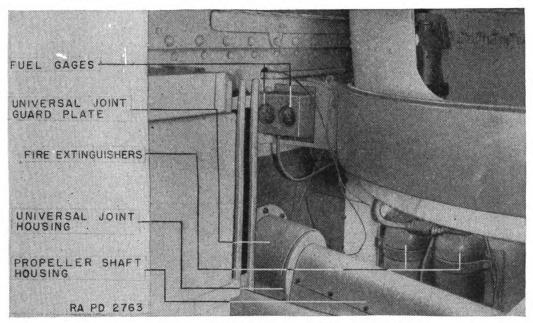
FIGURE 38.—Interior view, right side of bulkhead.
