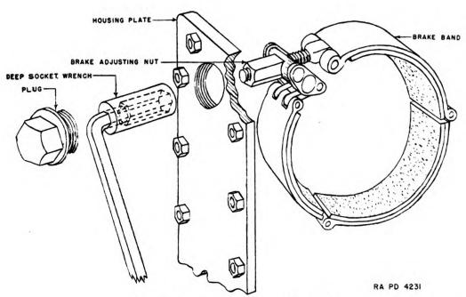
FIGURE 45.—Adjustment of steering brake.
