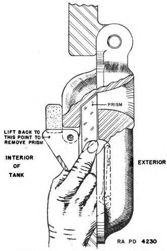
FIGURE 19.—Removal of prism from protectoscope.
