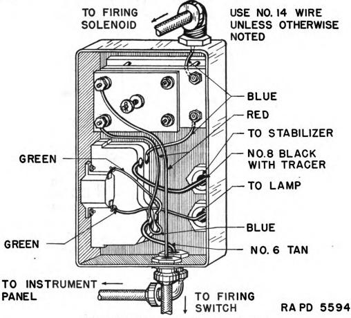
FIGURE 67.-75-mm gun switch and relay box.
