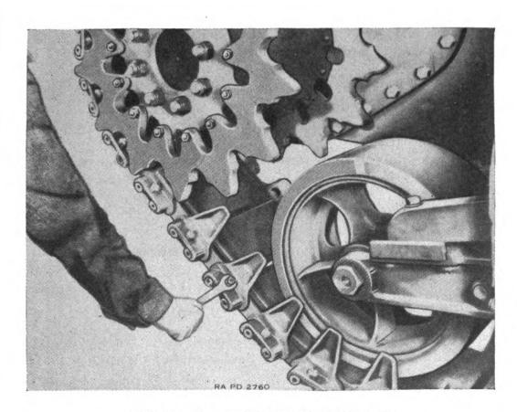
FIGURE 55.—Removing end connection from track.
