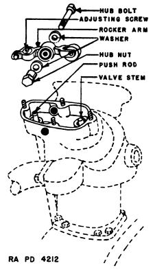
FIGURE 32.—Replacement of valve rocker arm.
