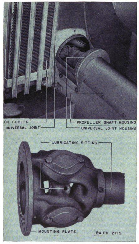
FIGURE 42.—Propeller shaft and universal joint.
