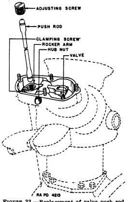
FIGURE 33.—Replacement of valve push rod.
