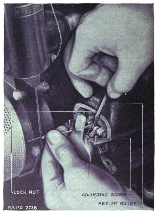
FIGURE 23.—Magneto point adjustment.
