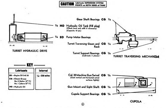
FIGURE 12.—Lubrication instructions for medium tanks M3 and M3A1—Continued.
