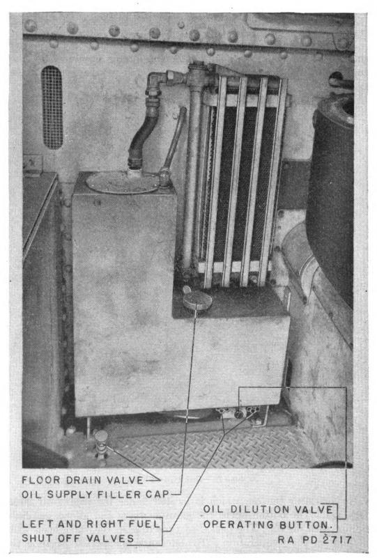
FIGURE 11.—Oil tank and cooler.
