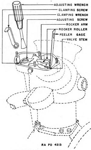
FIGURE 31.—Adjustment of valves.
