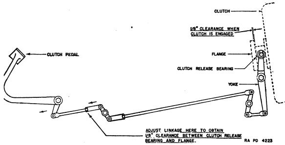
FIGURE 40.—Adjustment of clutch.
