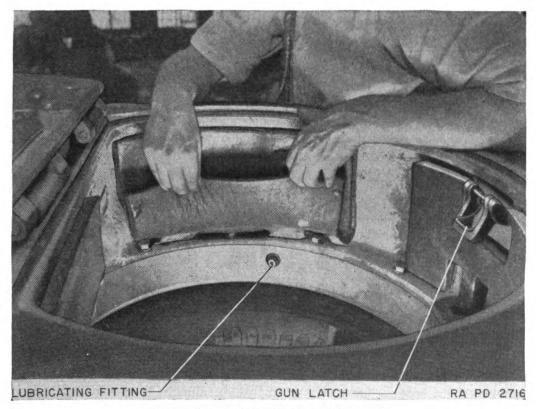
FIGURE 85.—Lubrication fitting in cupola.
