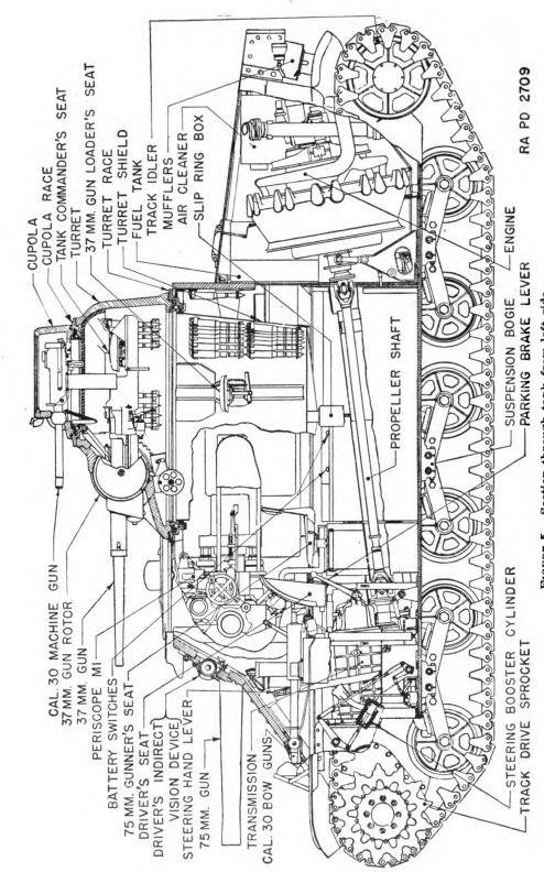
FIGURE 5.—Section through tank from left side.
