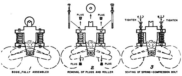
FIGURE 53.—Disassembly of bogie; first steps.
