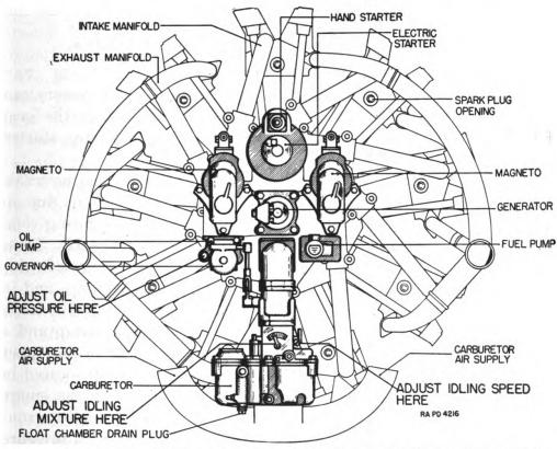
FIGURE 22.—Engine, showing accessories, adjustment of carburetor, and oil pressure.
