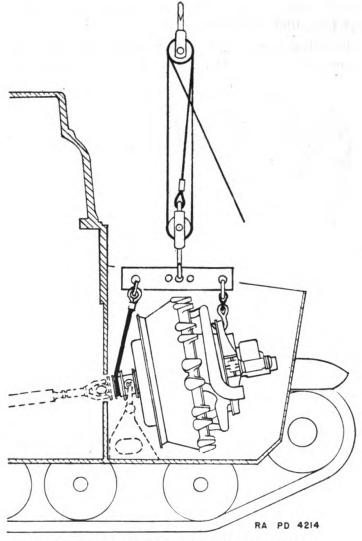
FIGURE 30.—Hoisting of engine, side view.
