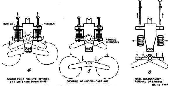
FIGURE 54.—Disassembly of bogie; final steps.
