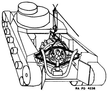
FIGURE 29.—Hoisting of engine, end view.
