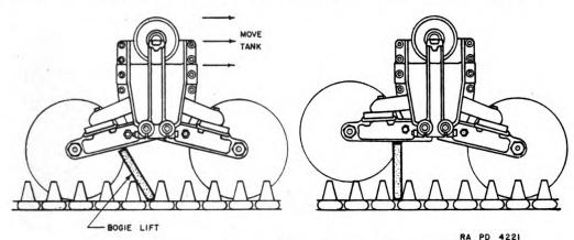
FIGURE 49.—Use of bogie left to raise wheel for removal.
