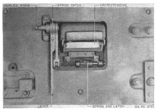
FIGURE 17 .- Pistol port with protectoscope.
