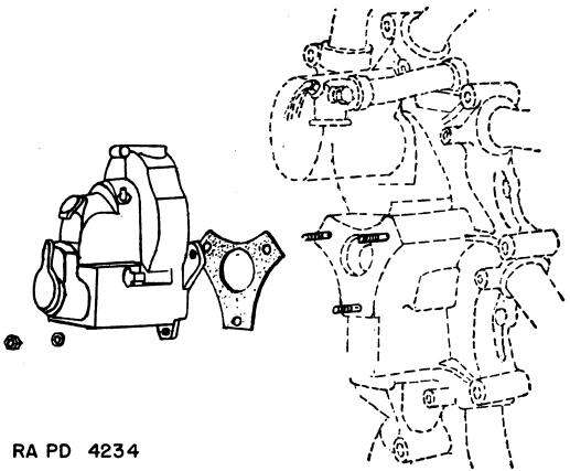
FIGURE 24.—Replacement of magneto.
