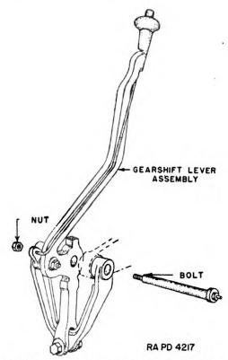
FIGURE 46.—Replacement of gear shift lever.
