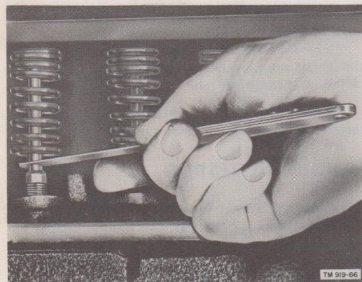
Figure 66. Checking valve tappet clearance.
