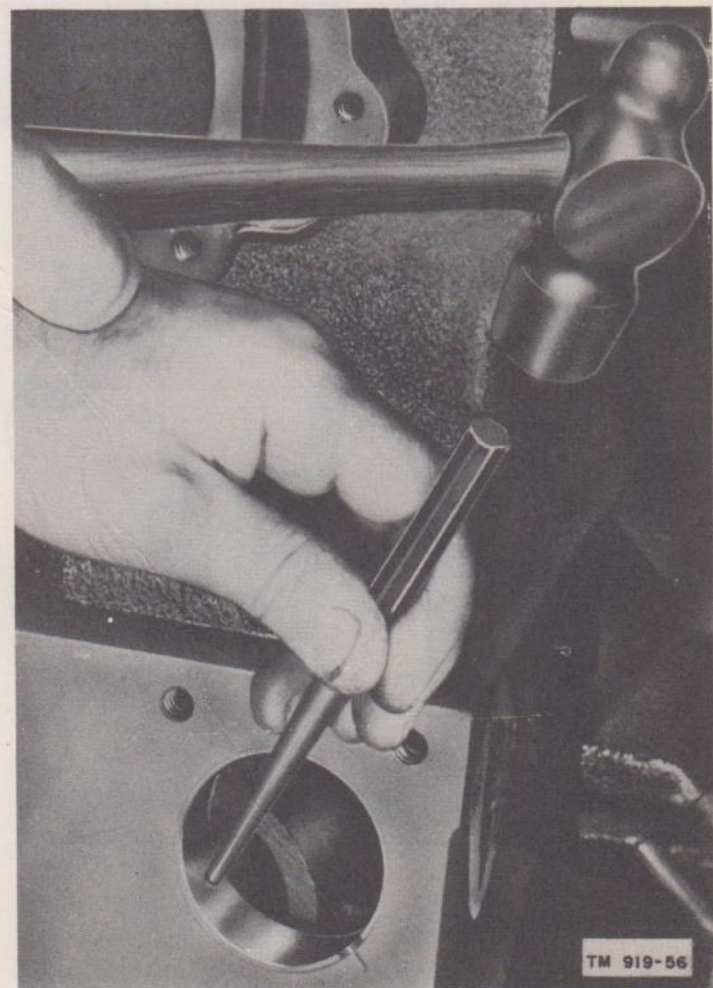
Figure 56. Staking camshaft bearing.
