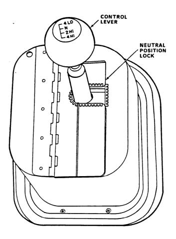
9. Set transfer case control lever to NEUTRAL (N) and engage transfer case lockout.
