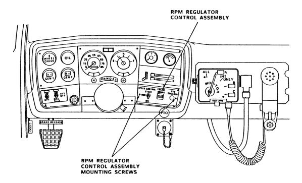
17. Reinstall RPM regulator assembly (item 32, C5122557-1) and secure with two screws (item 50, MS51959-70B). Using a NO.2 cross tip screwdriver, tighten screws.
