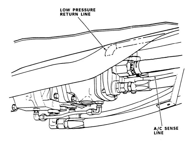
185. Position protective sleeve (item 56, C5131118-3) over generator pump low pressure return line (item 107, C5111009-1). Slide sleeve up hose, until top of sleeve is positioned just below channel bracket (item 6, C5110651-1). Trim sleeve as necessary. Using 1/4" flat tip screwdriver, tighten hose clamp (item 60, AN737TW58) securing protective sleeve (item 56, C5131118-3).
