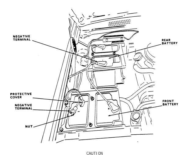
Prevent damage to engine electronic components. Disconnect batteries in following order: First, disconnect negative (-) terminal from rear battery.
