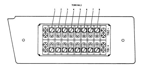
46. Route W67E1 and W67E2 through radio hole in dashboard. Connect W67E1 to TB2-3 and W67E2 to TB2-5 on rear of RPM regulator assembly (item 32, C5122577-1) using 3/16" flat tip screwdriver. Ensure W-67 cable (item 33, C5122564-1) is clear of heater controls in dashboard.
