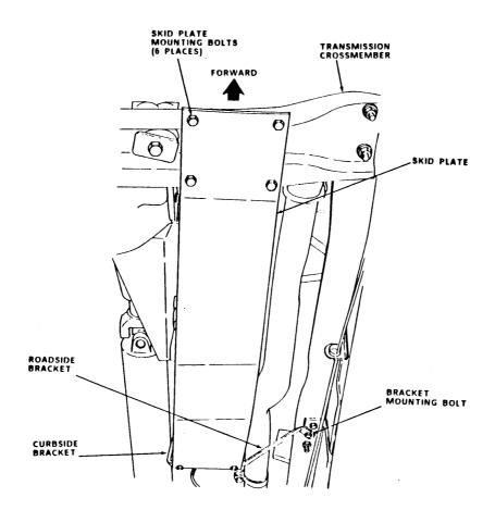
216. Install roadside skid plate bracket (item 5, C5118948-1) on left frame rail with two bolts (item 37, MS90725-8), nuts (item 43, MS51971-1), flat washers (item 45, AN960C416) and lock washers (item 47, NAS1640-416). Install bolts in available hole of frame rail. Using 3/8" drive ratchet handle, 7/16" socket, and 7/16" combination wrench, tighten bolts (item 37, MS90725-8).
