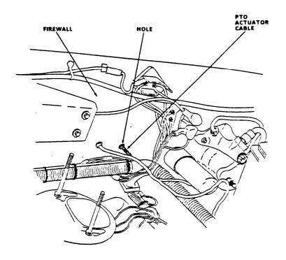
25. Place PTO actuator cable between engine and firewall towards PTO unit.
