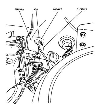
47. Install W-67 cable (item 33, C5122564-1) through hole in firewall and into engine compartment.
