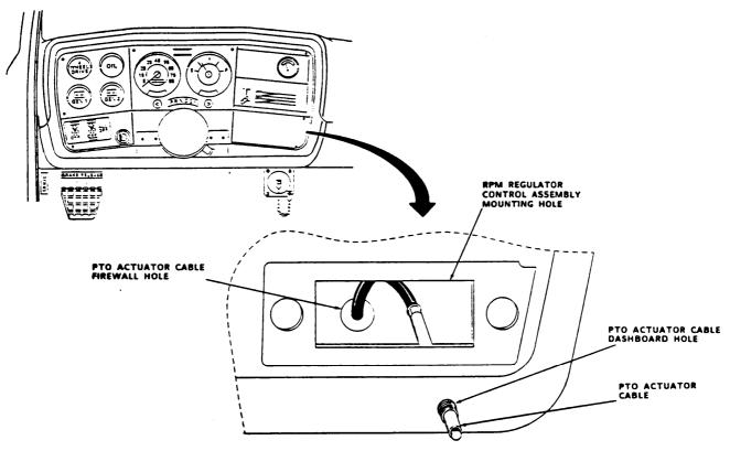
24. In truck cab, insert PTO actuator cable through hole in firewall and install through hole previously drilled in dashboard.
