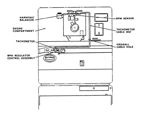
48. In engine compartment, route W-67 cable (item 33, C5122564-1) to sensor pickup at harmonic balancer.
