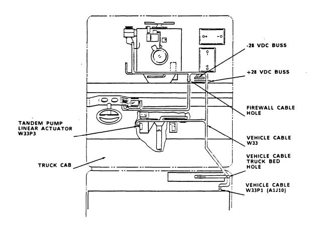
68. Place W-33 vehicle cable (item 29, C5110787-1) through existing hole in the right front corner of the floor of the truck bed. Make sure existing grommet is in good condition. Route W-33 vehicle cable (item 29, C5110787-1) under vehicle along upper vehicle frame, and up through engine compartment to firewall.
