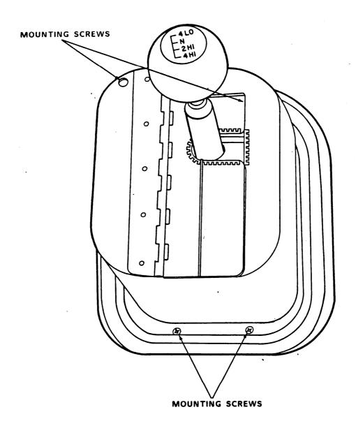
105. Using a no. 2 cross-tip screwdriver, remove and retain four escutcheon plate screws from transfer case shift lever assembly.
