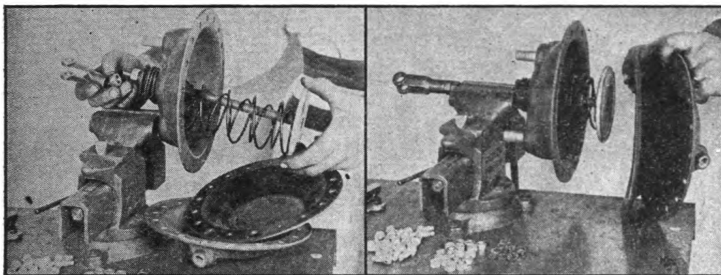
FIGURE 34. BRAKE CHAMBER—PUSH ROD REPLACEMENT. FIGURE 33. BRAKE CHAMBER—DISASSEMBLY.
