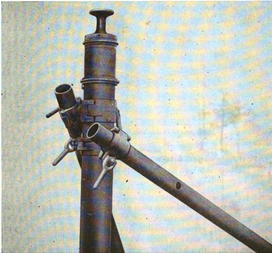
Figure 12. Column-bracing clamp used to fasten bracing strut to trestle column
