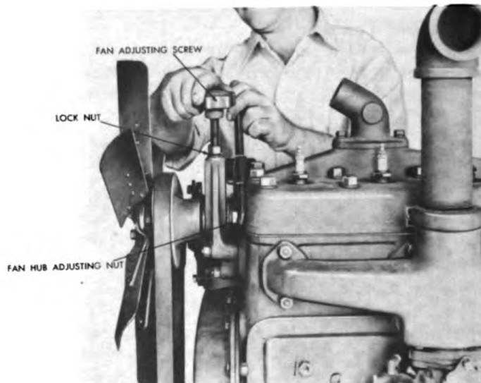
Figure 377. Installing Fan Assembly.
