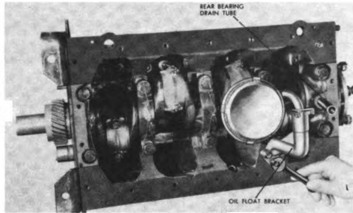
Figure 357. Installing Oil Float and Tube.
