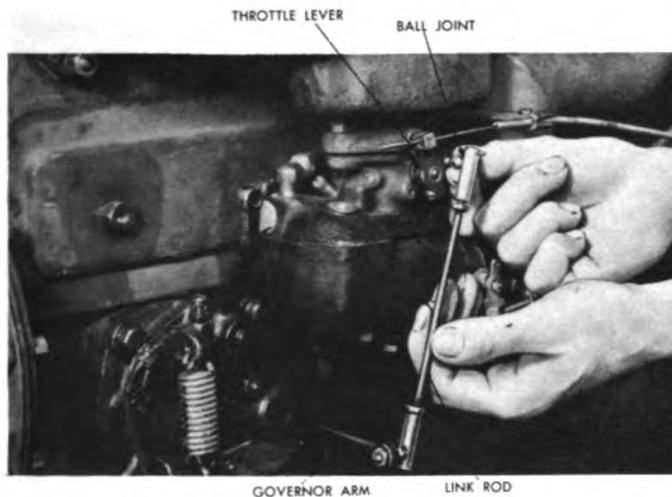
Figure 316. Adjusting Governor Link Rod.
