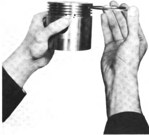
Figure 205. Checking Depth of Ring Groove.
