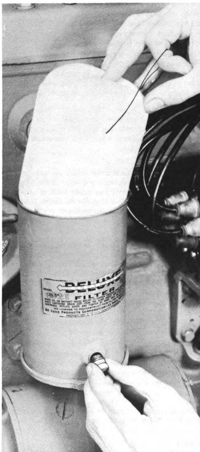
Figure 62. Removing element of oil filter.
