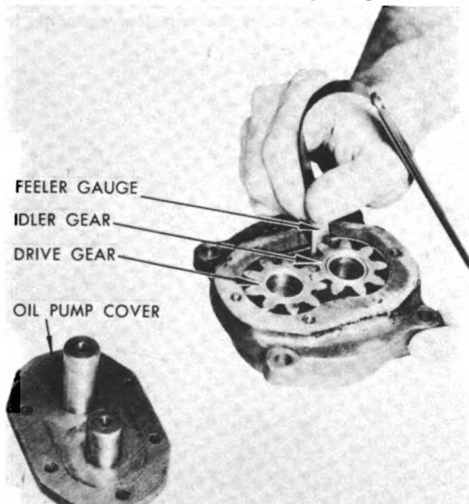
Figure 318. Checking Oil Pump Gear Clearance to Pump Case.
