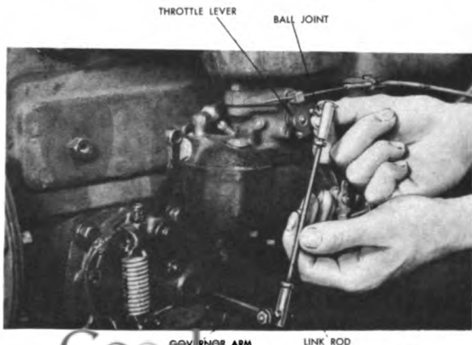
Figure 306. Adjusting Governor Link Rod.
