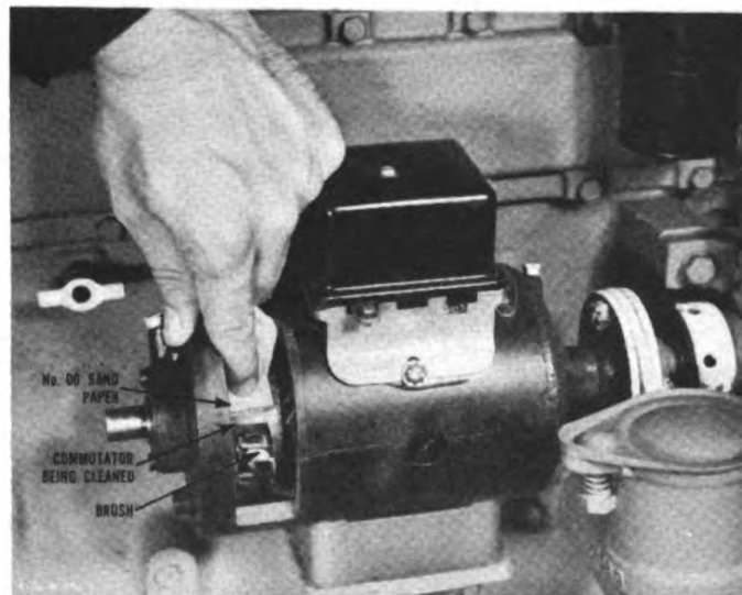
Figure 54. Cleaning generator commutator.
