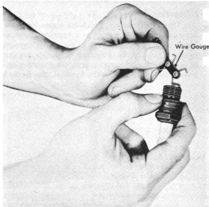
Figure 63. Checking spark plug gap.
