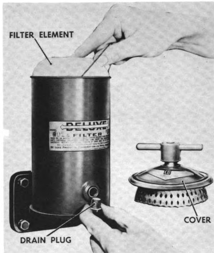
Figure 326. Removing Filter Element.
