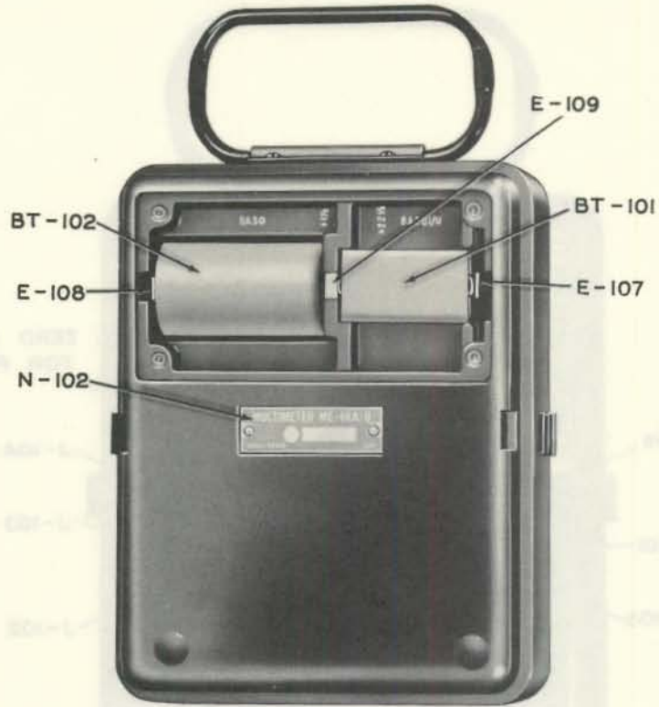
Figure 3-3. Battery Compartment, Cover A-103 Removed.
