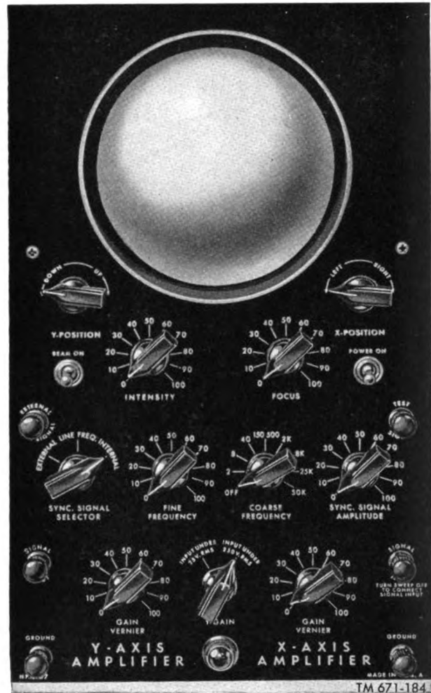
Figure 179. Front panel of typical test oscilloscope showing controls.
