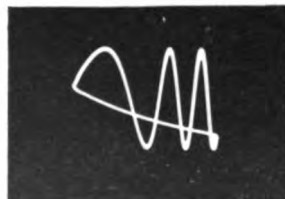
A, Nonlinear sweep; B, Distorted sine-wave trace as a result of using sweep shown in A.
