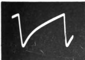
A, Nonlinear sweep; B, Distorted sine-wave trace as a result of using sweep shown in A.
