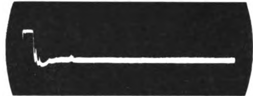
A—Receiver Not Tuned to Test Set Frequency
