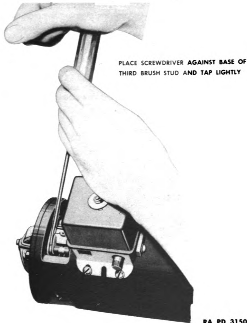
Figure 8—Adjusting Position of Third Brush
