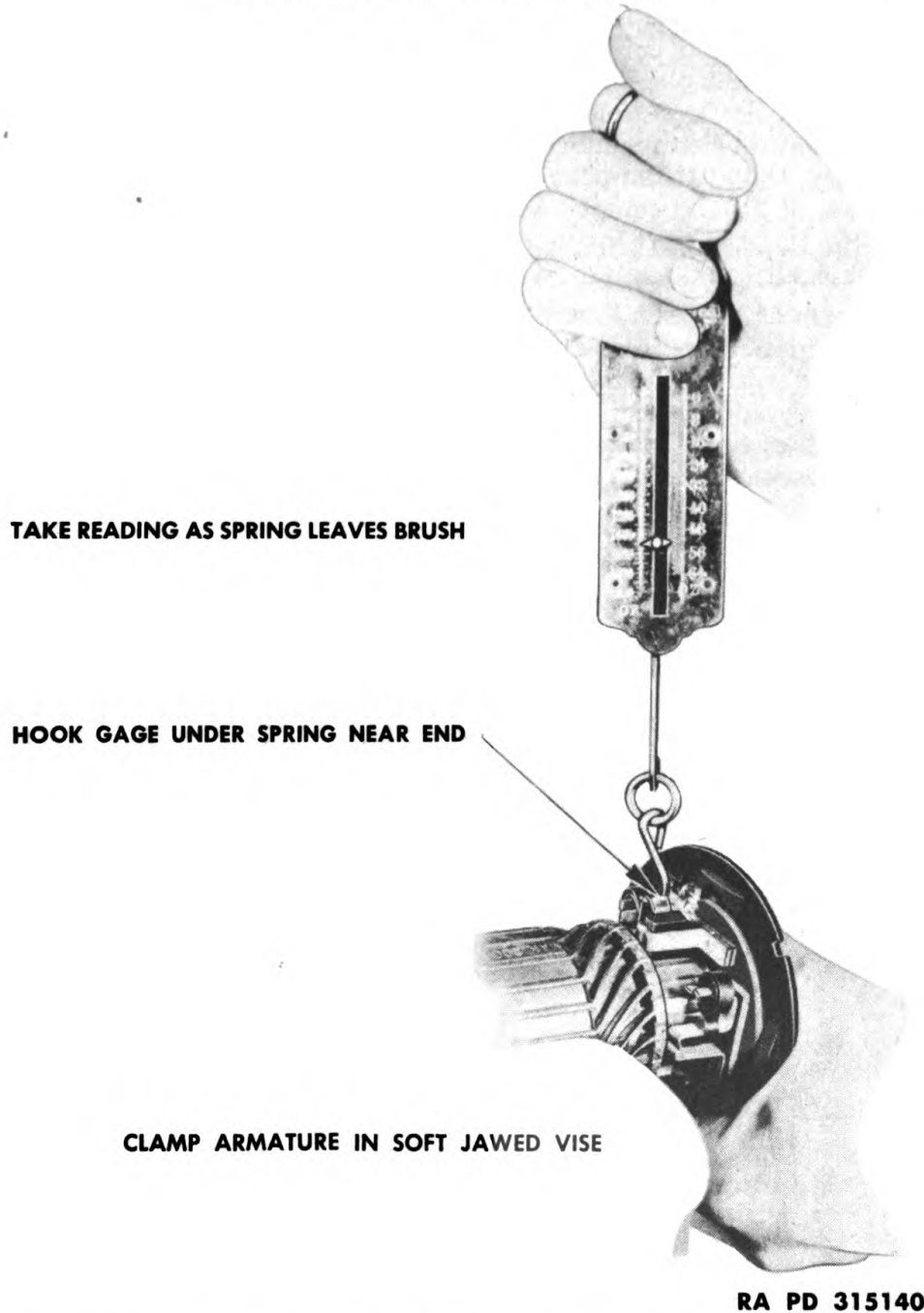
Figure 133—Measuring Brush Spring Tension with Tension Gage (41-G-105)
