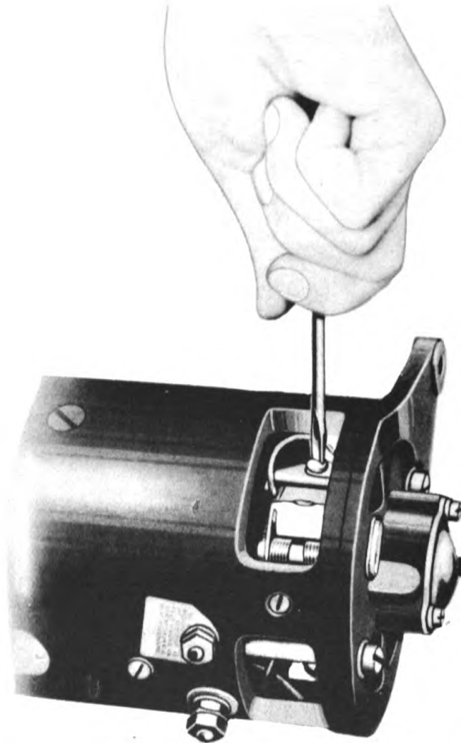
Figure 33—Disconnecting Brush Lead from Holder
