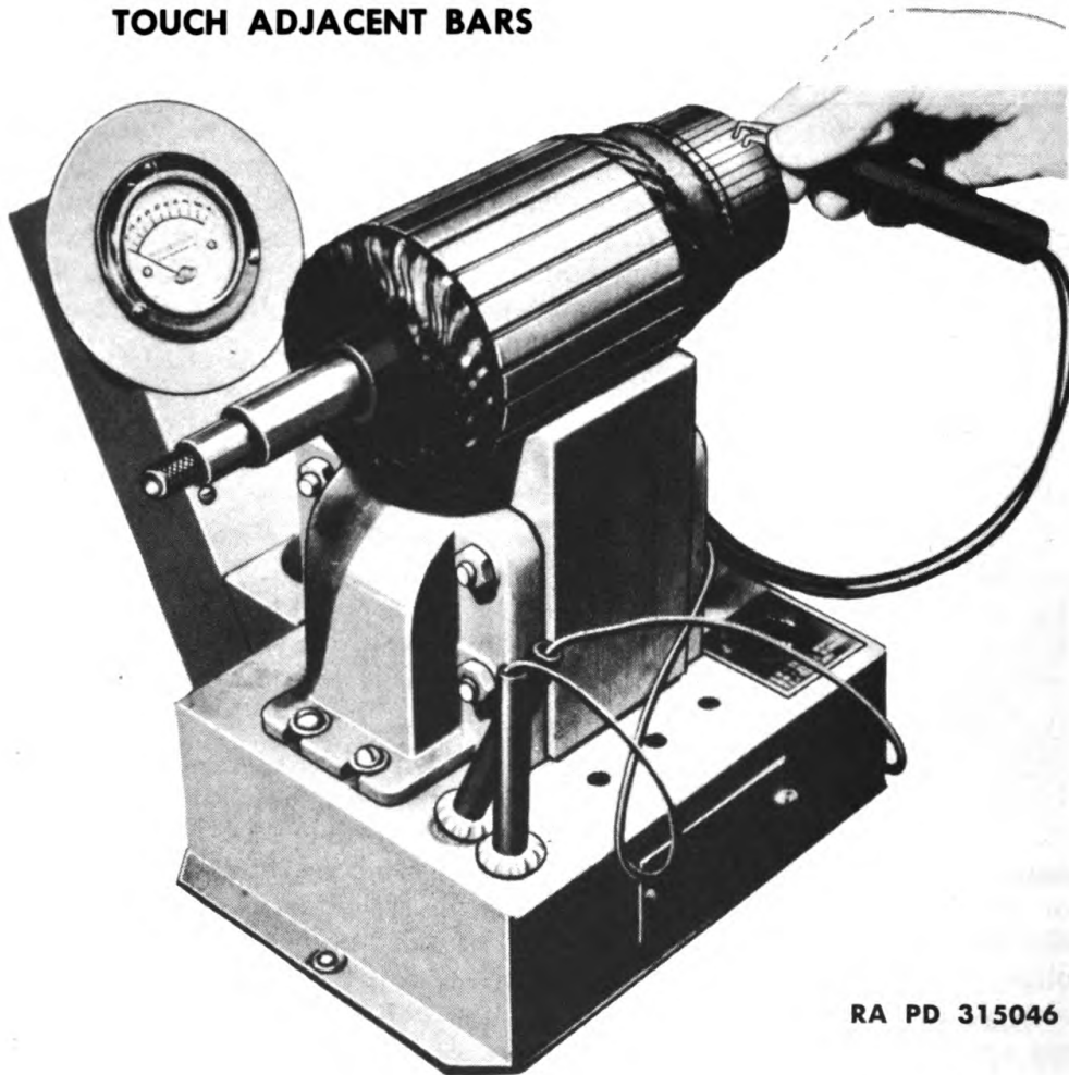
Figure 58—Testing Armature for Shorts with Growler (17-G-5940) and A-C Milliammeter
