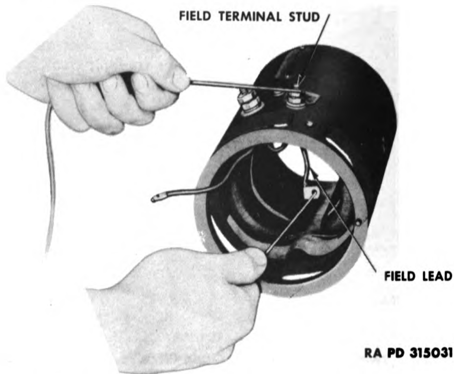
Figure 42—Testing Field Coils for Open Circuits with Test Probes— Group 2B Generators
