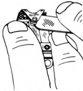
MEASURING CONTACT GAP WITH FLAT FEELER GAGE
