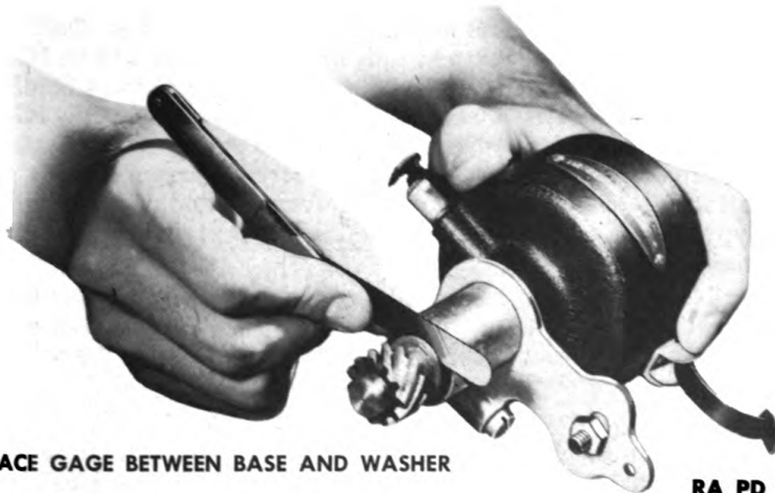
Figure 112—Measuring End Play of Shaft with Thickness Gage (41-G-400)
