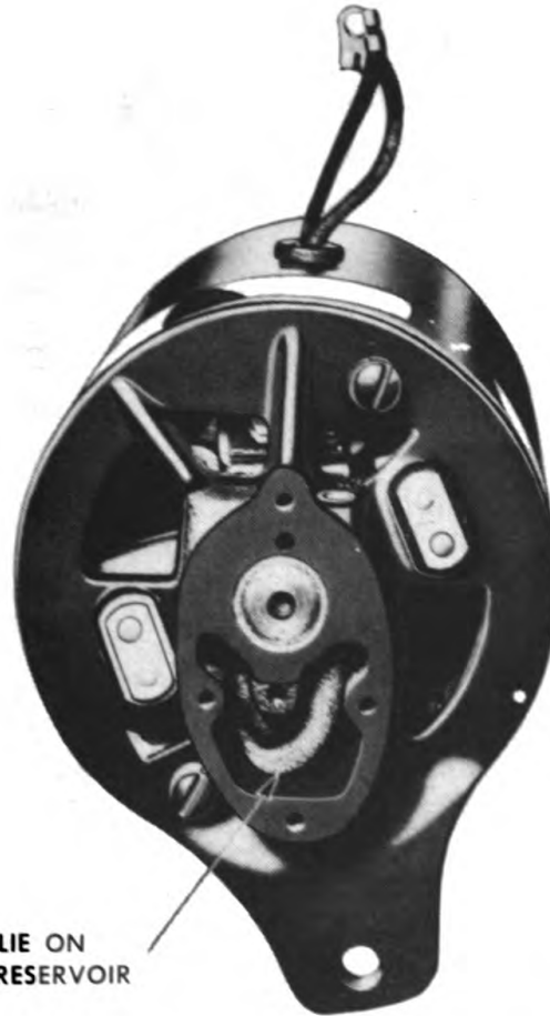
Figure 49—Position of Felt Wick in Oil Pocket
