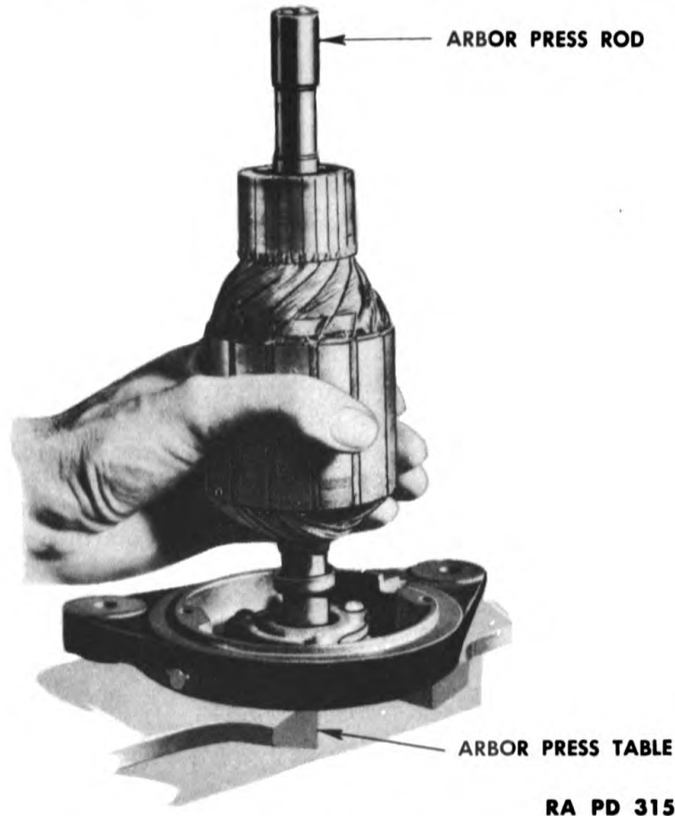
Figure 27—Pressing Armature Shaft into Drive End Head with Arbor Press
