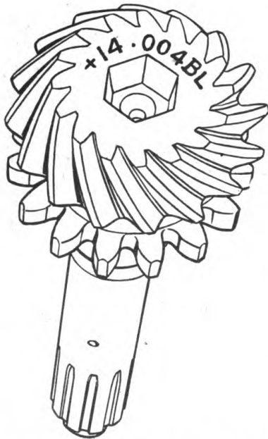
Fig. 76. Spiral Bevel Gear and Clutch Shaft Showing Gauge and Back Lash Markings
