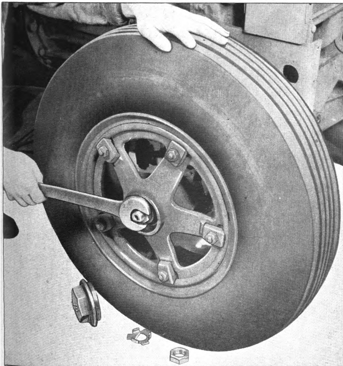
Fig. 92. Adjusting Front Wheel Bearing
