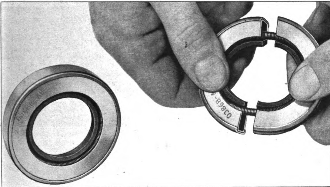
Fig. 84. Detail of Oil Seal. At Left Complete Seal Ready for Installation with face Toward the Oil Pressure. Seal at Right Cut Open to Show Arrangement of Leather and Coiled Spring in Seal
