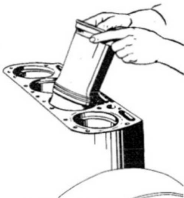
Fig. 21. Installing Cylinder Sleeves
