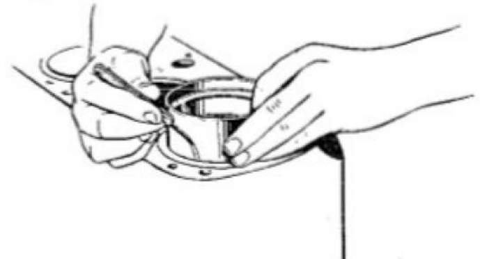
Fig. 24. Checking Piston Clearance in Cylinder
