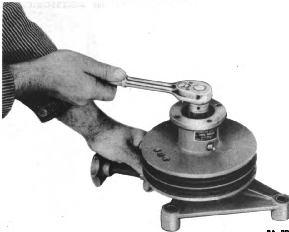
Figure 98 – Removing Nut from Fan Pulley Spindle
