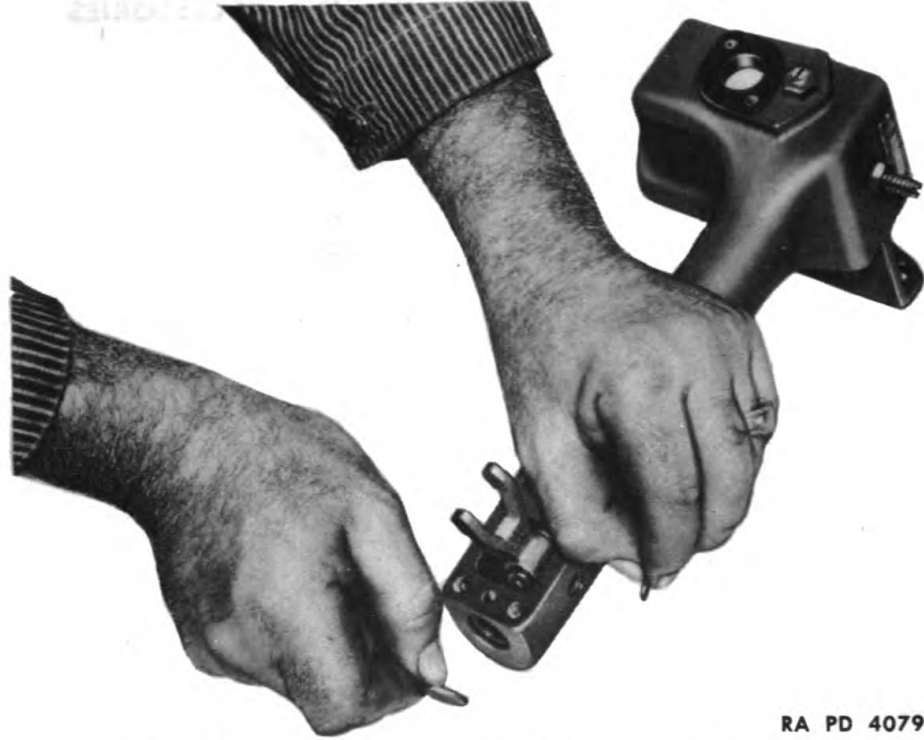
Figure 156 – Expansion Plugs Removed from Control Housing
