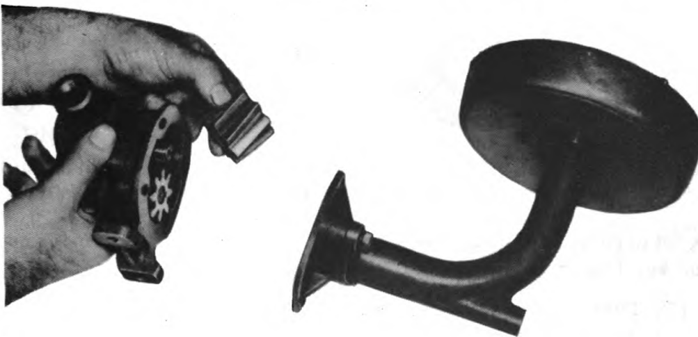
Figure 139 – Removing Lubricating Oil Pump Gear Cover
