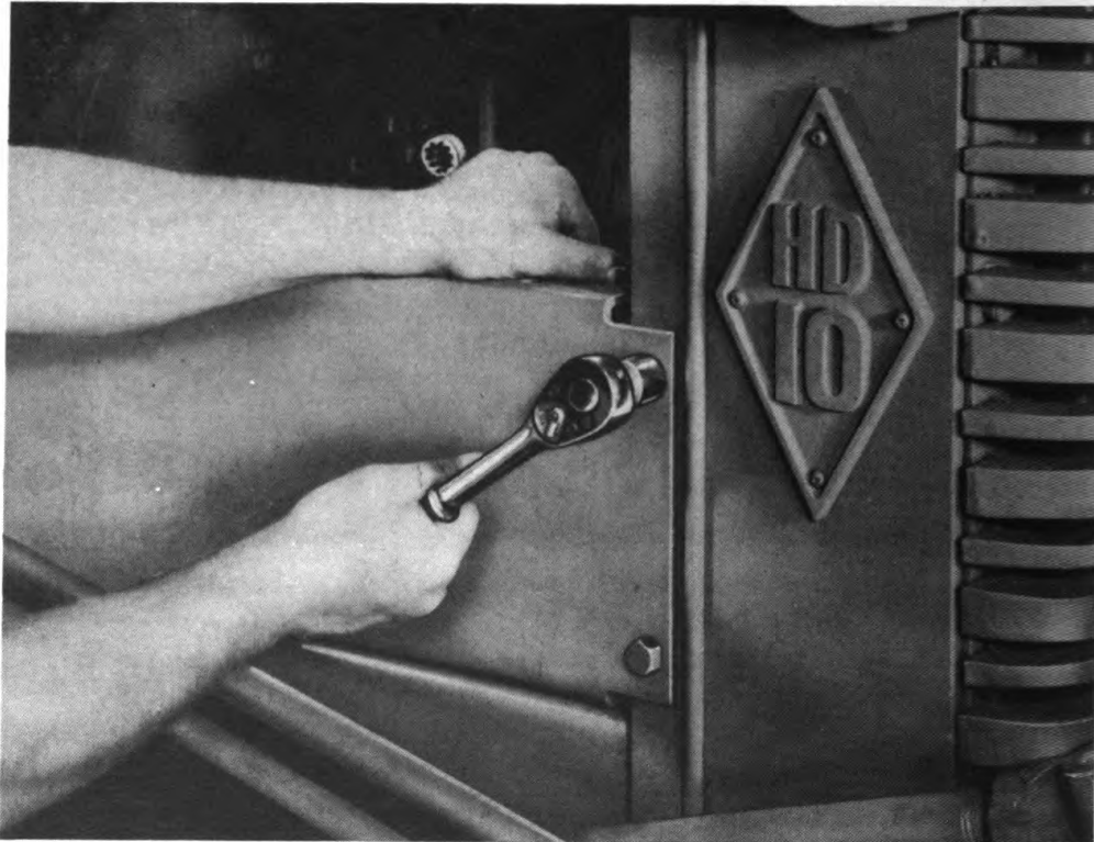
Figure 91 – Removing Right Front Fender
