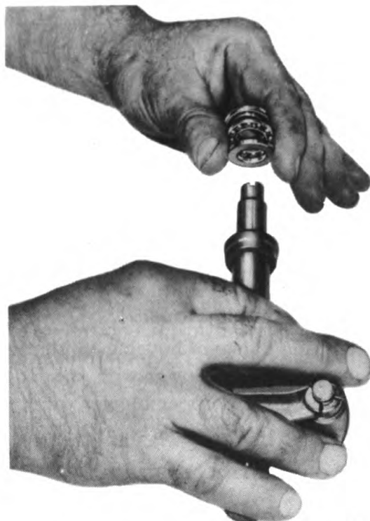
Figure 166 – Installing Riser and Thrust Bearing on Weight Carrier Shaft
