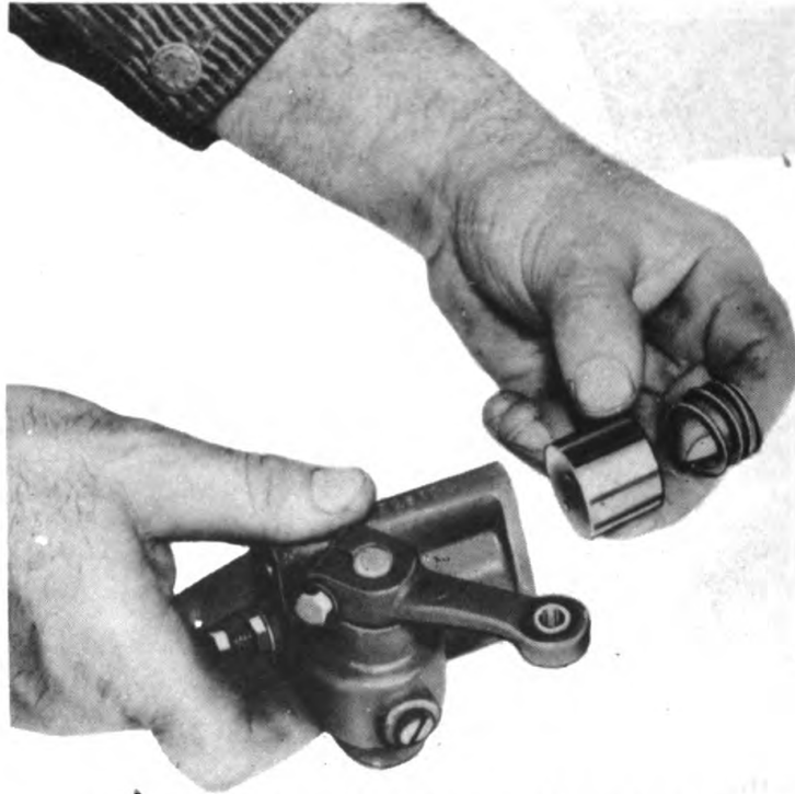
Figure 163 – Installing Variable Speed Spring Retainer
