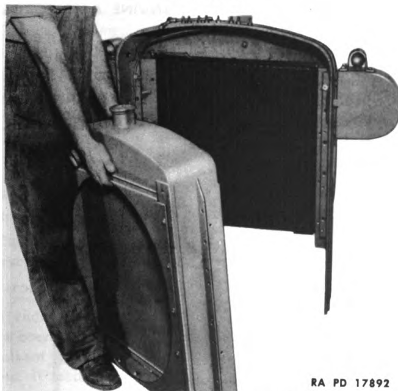
Figure 108 – Radiator Removed from Shell
