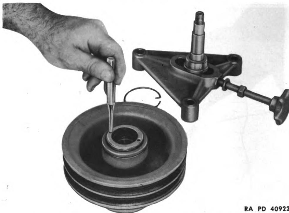
Figure 99 – Removing Cork Retainer from Pulley
