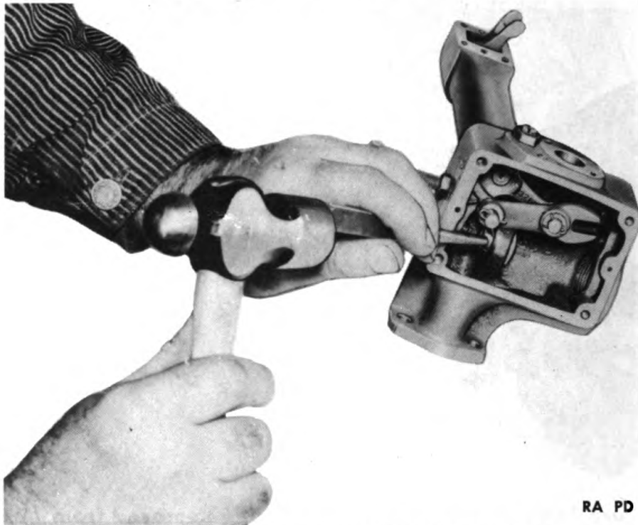
Figure 155 – Removing Variable Speed Spring Plunger Guide
