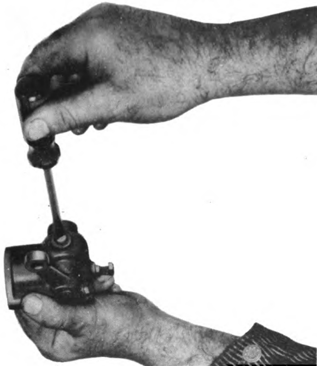
Figure 159 – Removing Pipe Plug from Spring Housing
