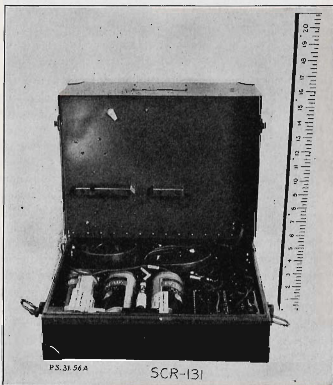
FIGURE 4.—Radio receiver and transmitter BC-148 (151), showing interior of battery-compartment box.
