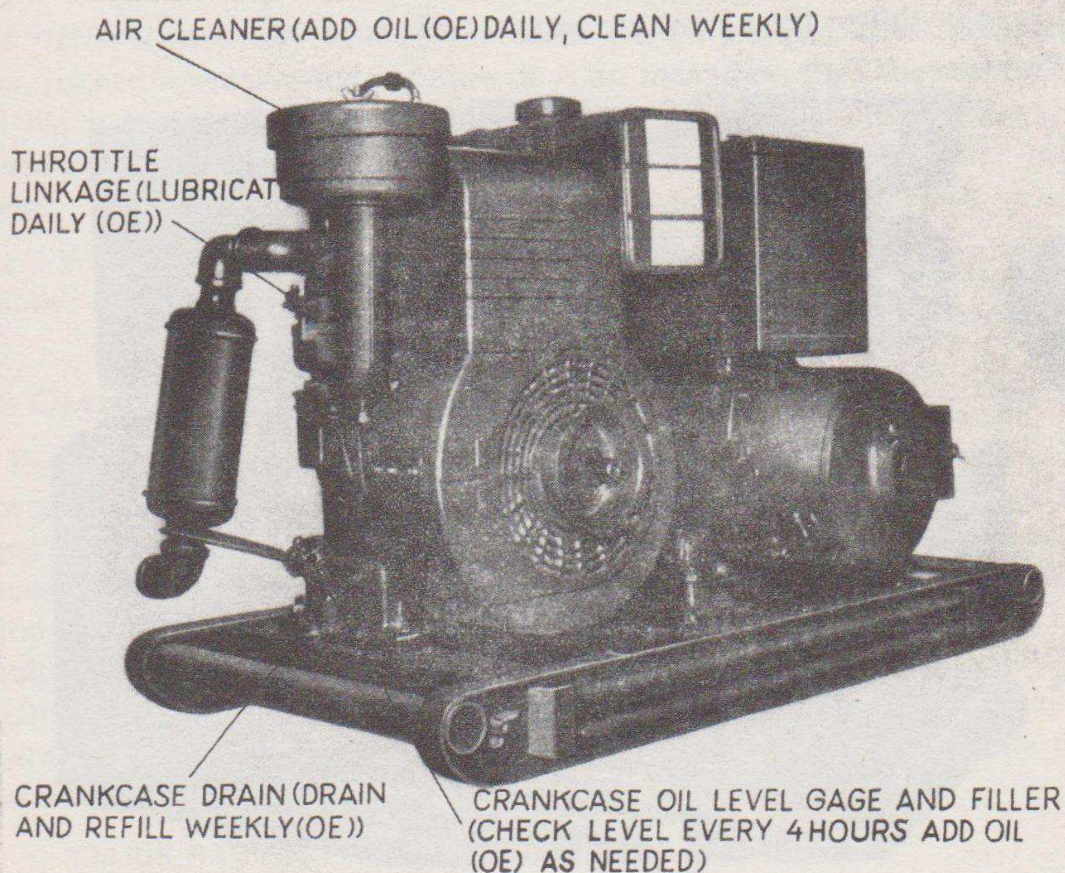
Figure 8. Power Unit PE-75-AF-GY, lubrication.
