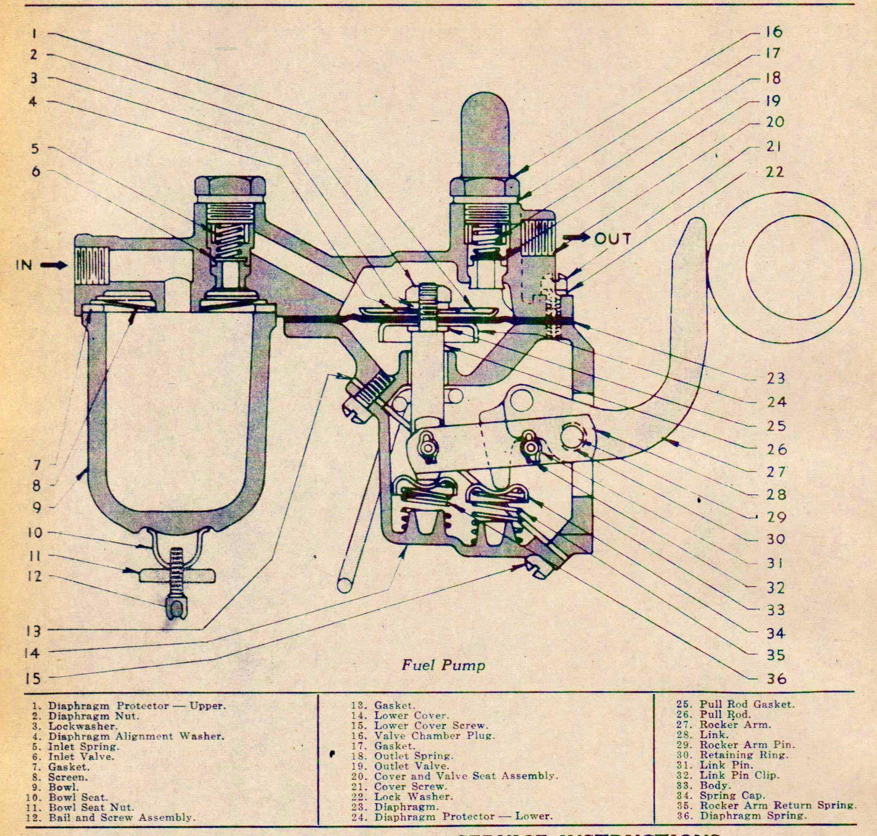
forces the diaphragm up and the fuel through to the carburetor. When the carburetor is full, the needle valve builds up a pressure in the pump chamber, holding the pump spring down until more fuel is needed.
