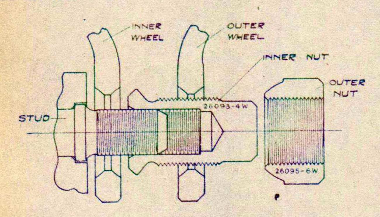
The dual wheels are locked with double cap nuts. The inner dual is individually held by a sleeve-like inner cap nut. The inner dual must be mounted and tightened down before the outer wheel is put on. The outer dual slips over the inner cap nuts and is locked in place with the outer nuts. The wheels do not pilot at the hub center; the entire load is distributed over the cap nuts and studs.
