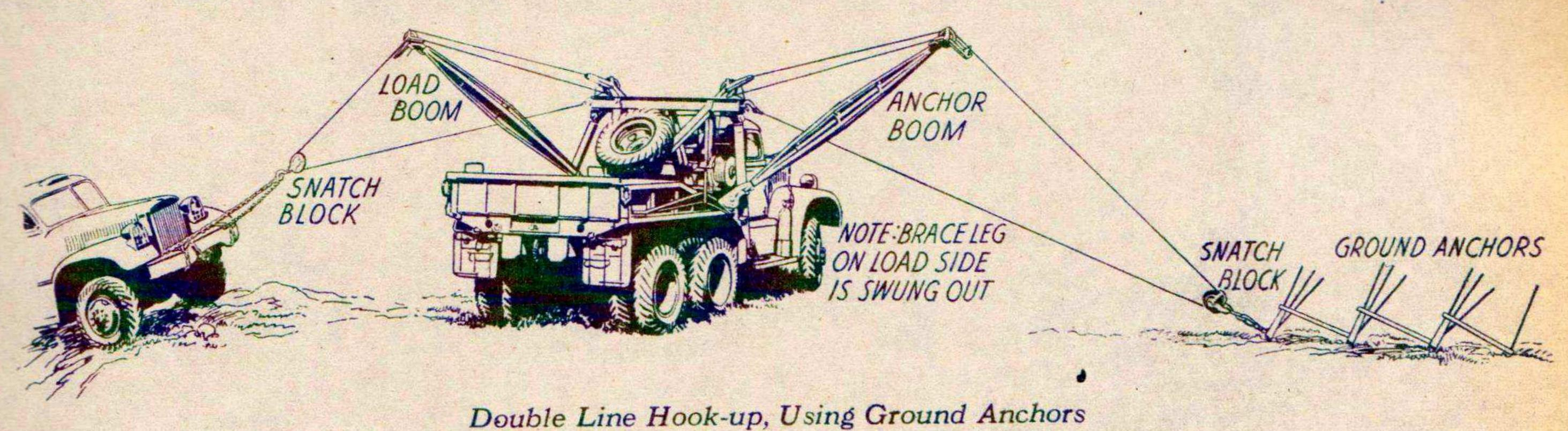
Illustration shows hook-up with double line on load side and on anchor side, both booms out, and in line with each other. Brace leg out on load side only. Snatch blocks should be used in both load and anchor
