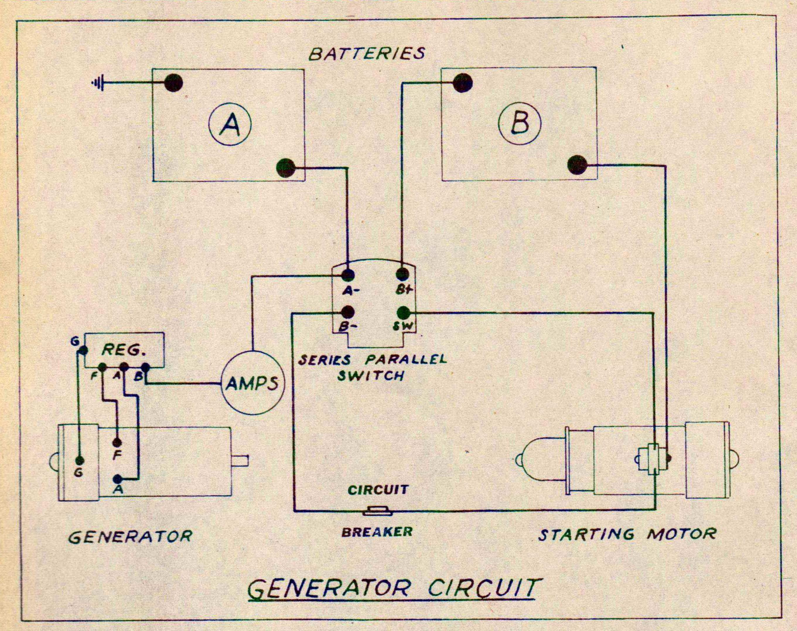
voltage regulator to hold the system voltage constant within close limits under operating conditions of the system's capacity.
