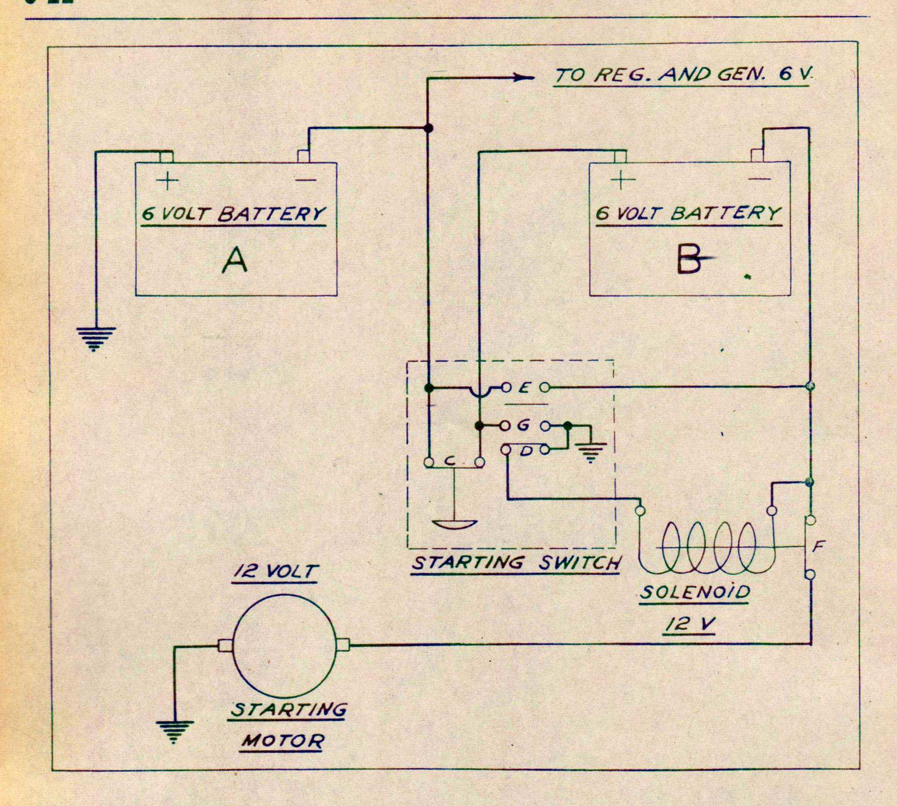
Series-Parallel Circuit — Two switches are used in this circuit, one a solenoid switch mounted on the starting motor and the other a manually operated series parallel switch.
