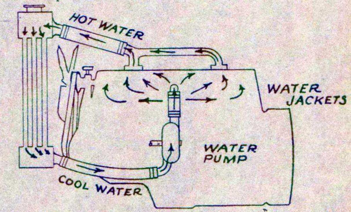
This is a pressure cooling system with a mechanism in the radiator cap to keep the internal pressure of the system several pounds per square inch above atmospheric pressure. The radiator is always sealed unless the pressure increases beyond the setting limit, in which event the seal is broken and vapor, air or water escape through the overflow tube until such time as the internal pressure has returned to its proper level.
