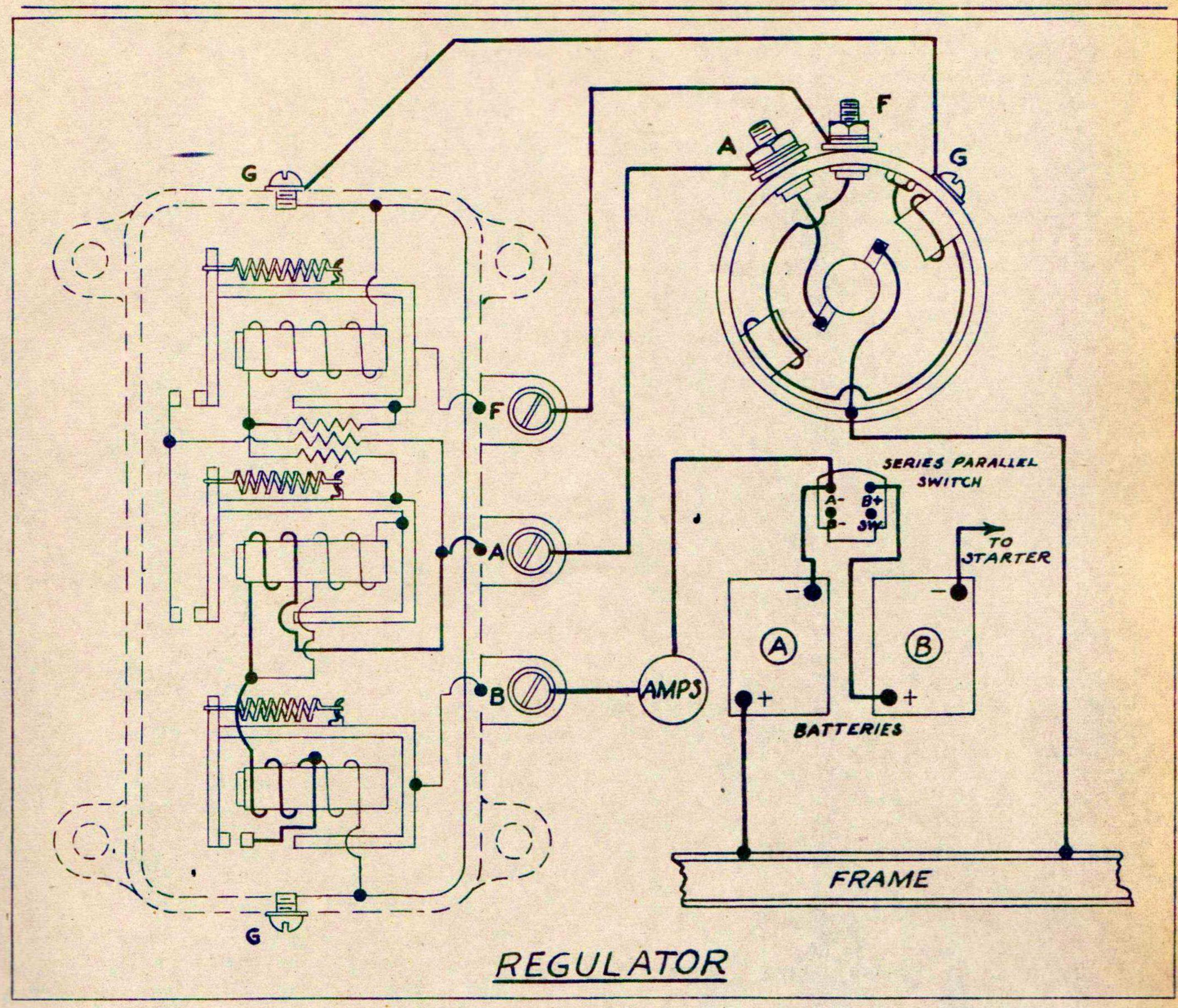
In operation when the generator output reaches its predetermined maximum, the regulator points are opened, inserting resistance in the field circuit and reducing the ampere output of the generator. Immediately upon the dropping of the output the points close, shorting out the resistance and the output rises completing one cycle of operation.
