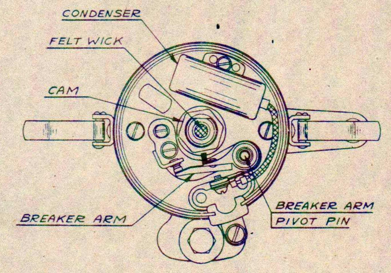
to have a smooth, flat contact with each other. Also be sure they are properly aligned so as to have full face contact.
