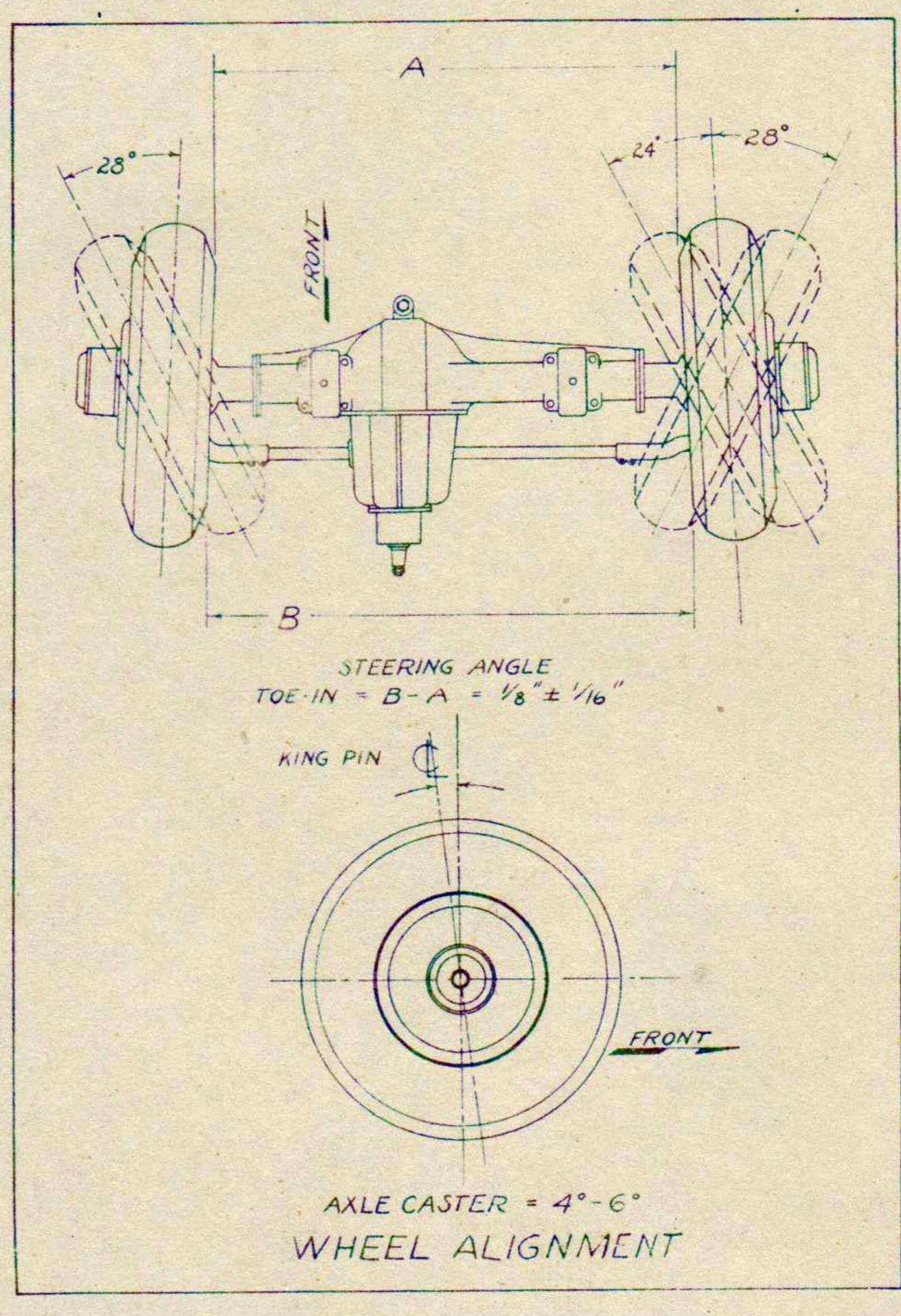
angle of 28° for the inside wheel. When this condition is reached, the outside wheel has a turning angle of about 24°. These stops are welded in correct adjustment and it should not be necessary to make any changes. If the steering angle should come out of adjustment, it would be caused by worn or bent parts in the steering linkage, sprung axle housing or stops broken from axle.
