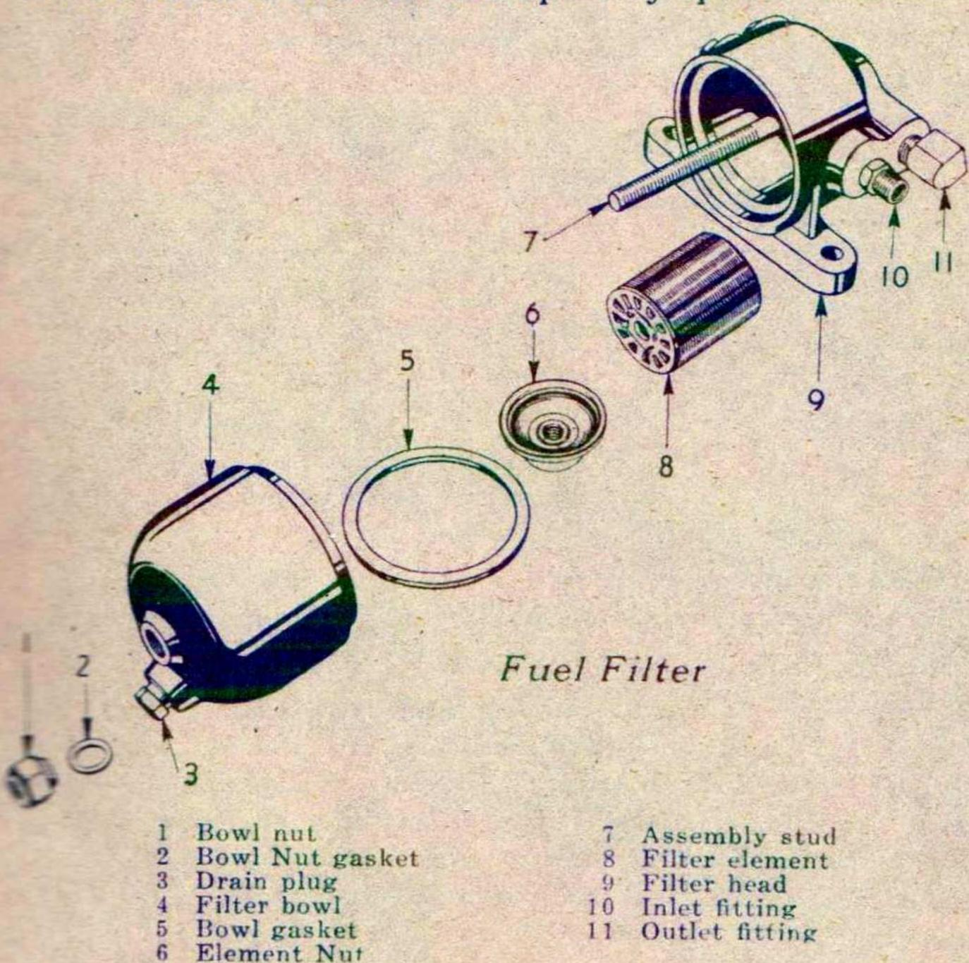
The filter bowl should be drained frequently to remove water and foreign matter that has collected and should be periodically cleaned as follows.
