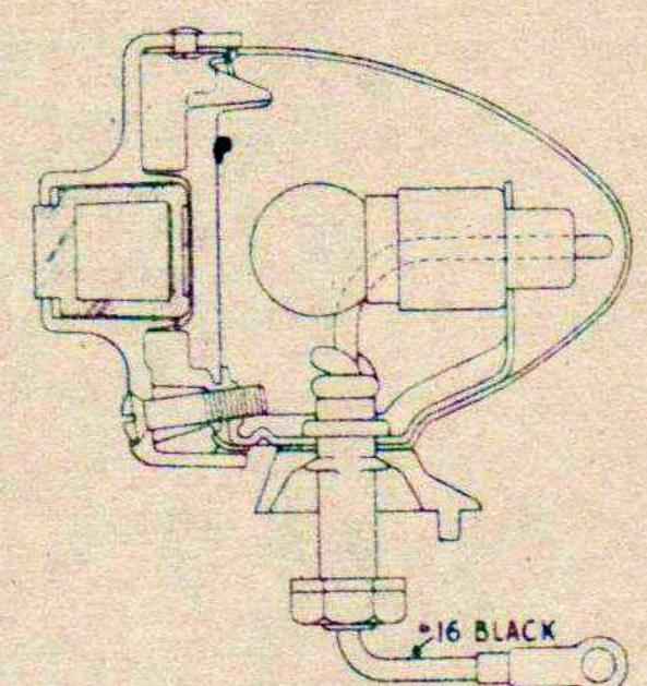
With the main switch in the blackout position the electrical circuit is completed through the blackout lights rather than the service lights.
