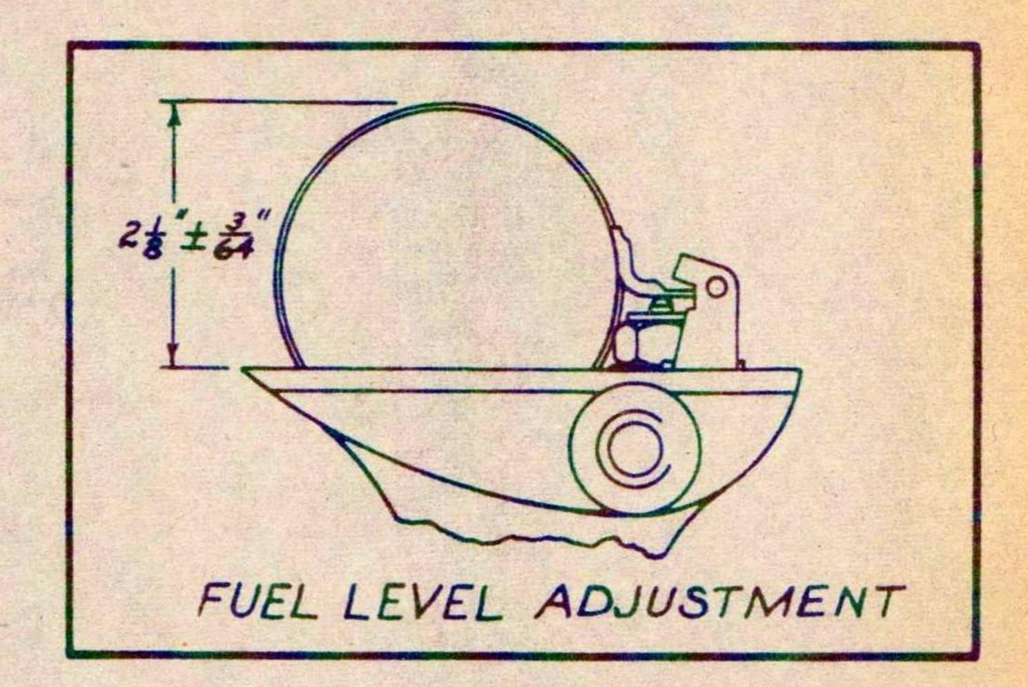
Fuel Level — Maintenance of the correct fuel level in the bowl is very important in obtaining fuel economy. This level may be checked with a conventional fuel level gauge or by removing upper cover assembly and measuring the height of the float. The float arm may be bent to obtain the proper adjustment. The illustration shows the method of checking the float level and gives the necessary dimensions.
