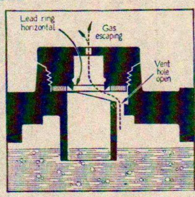
Replacing vent plug tilts ring and opens vent hole. for normal passing of charging gas.
