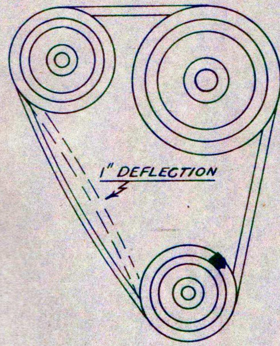
When making a belt adjustment, first loosen the clamping nut back of the fan assembly. Then turn adjustment screw in the top of the fan bracket until the desired condition is reached. Tighten clamping nut.
