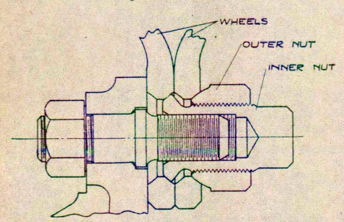
Cap nuts should be tightened with the wheels off the ground. The outer nuts must be backed off at least two full turns to facilitate tightening the inner cap nuts, which must not be neglected. The cap nuts should be tightened in a criss-cross fashion and not around the wheel.
