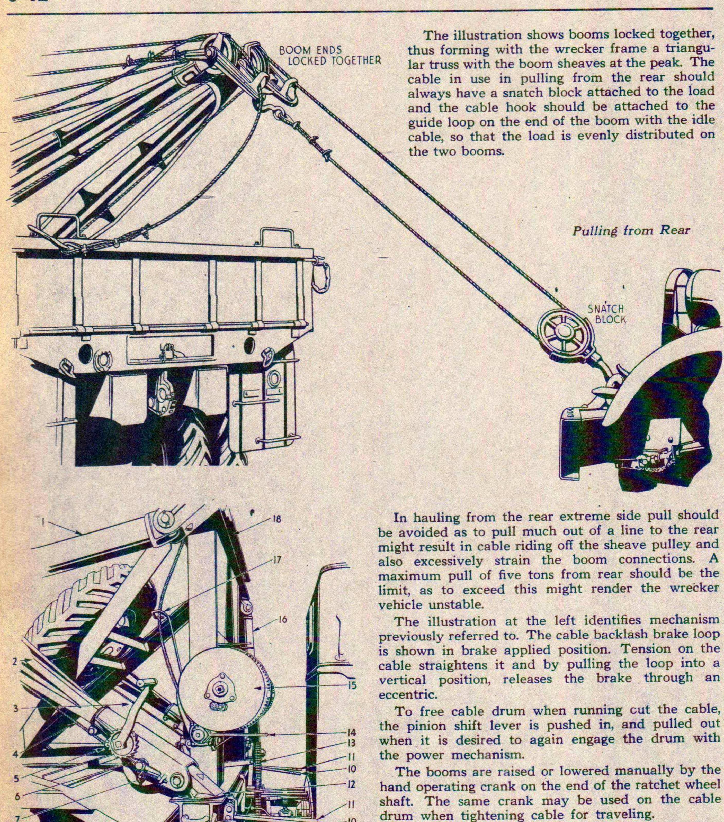
To free cable drum when running cut the cable, the pinion shift lever is pushed in, and pulled out when it is desired to again engage the drum with
